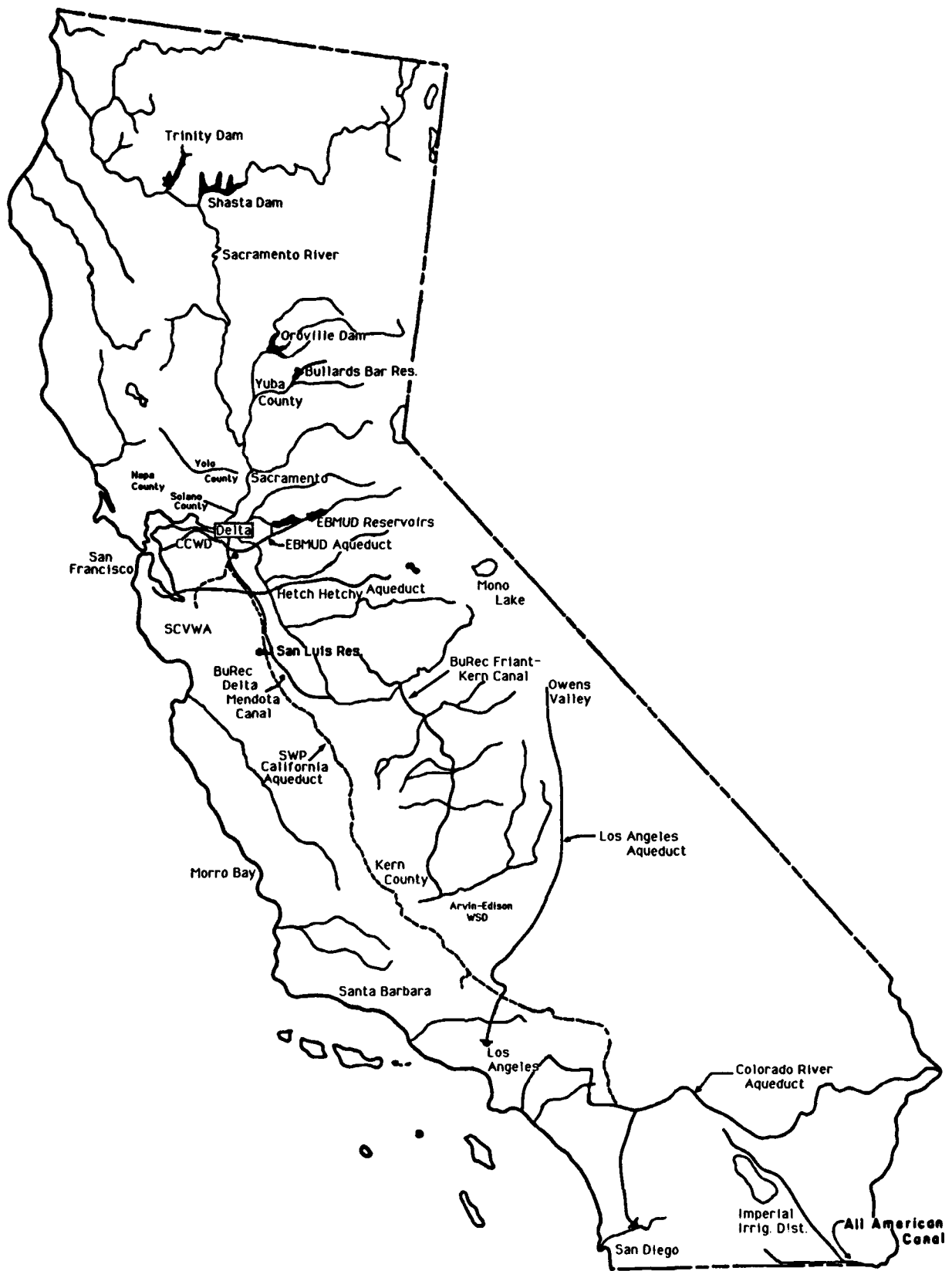
Figure 2-5 Major Water Storage and Conveyance Facilities
