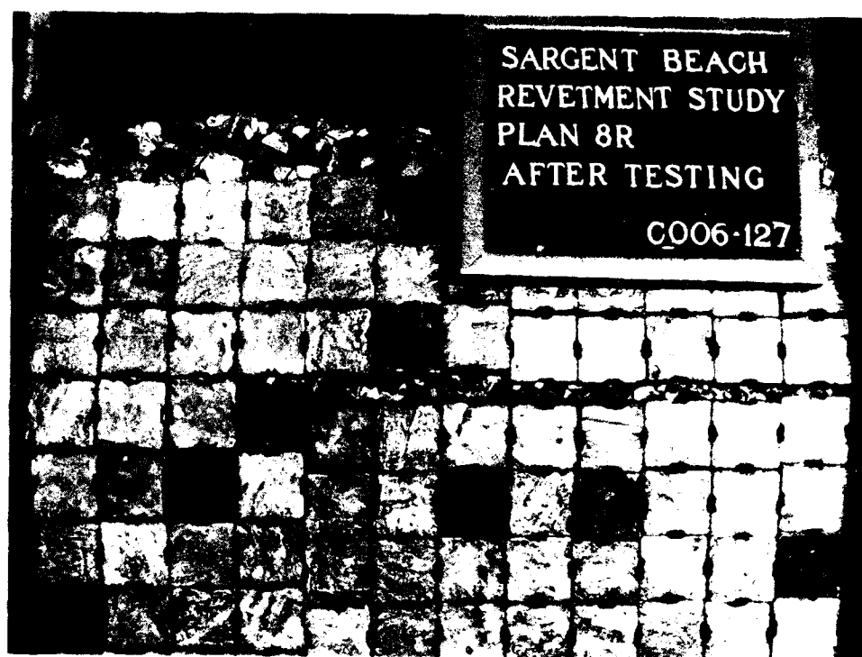
Photo 46. Overhead view of Plan 8R after wave attack
