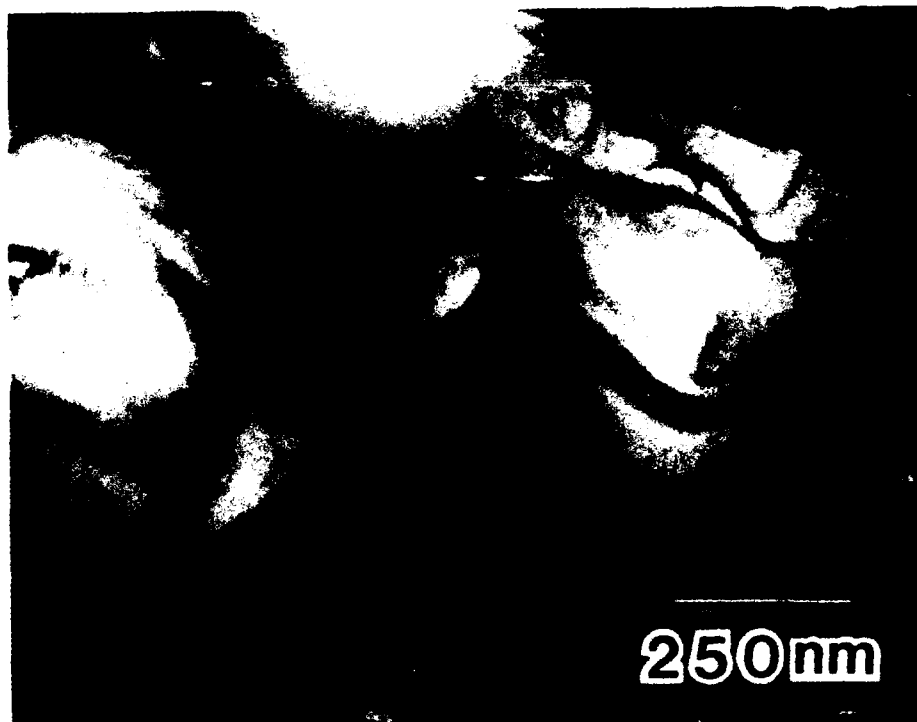
Figure 3.45 Bright field TEM micrograph of as-melt spun Nb-10Al-10Cr-10Ti-10W-1Er (alloy S5)
