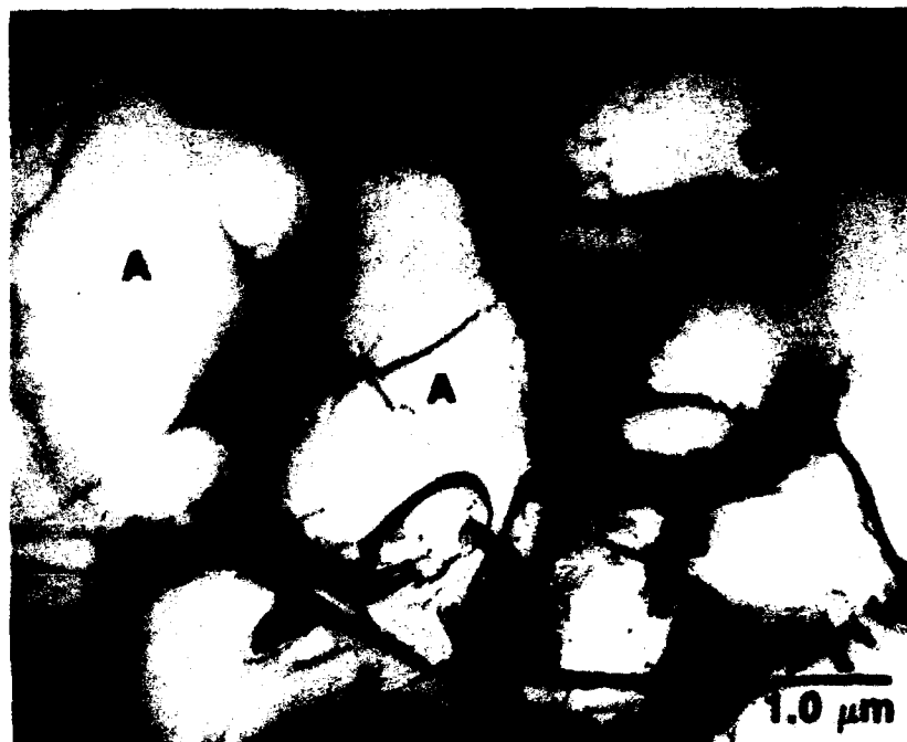
Figure 3.58. Bright-field transmission electron micrographs recorded from typical areas taken from thin foils of powders of alloy P5. Note the dendritic and interdendritic regions, marked A and B, respectively. Also note the presence of small particles, which have been identified as \text{Er}_2\text{O}_3 .
