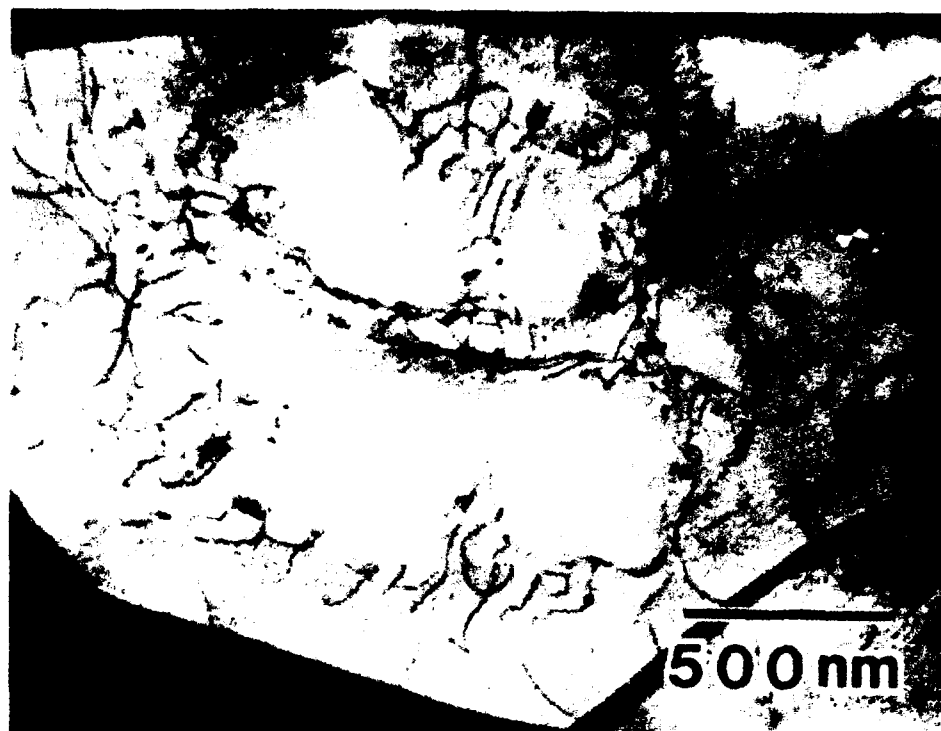
Figure 3.50 Bright field TEM micrograph of as-melt spun and heat treated Nb-15Ti-15W-3Mo-1Zr-1Er (alloy S7). Heat treatment was 600°C for 1 hour.
