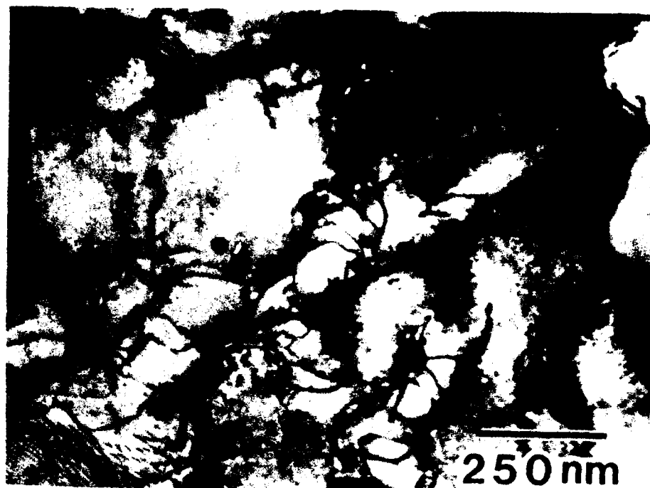
Figure 3.46 Bright field TEM micrograph of as-melt spun and heat treated Nb-10Al-10Cr-10Ti-10W-1Er (alloy S5). Heat treatment was at 600°C for 1 hour.
