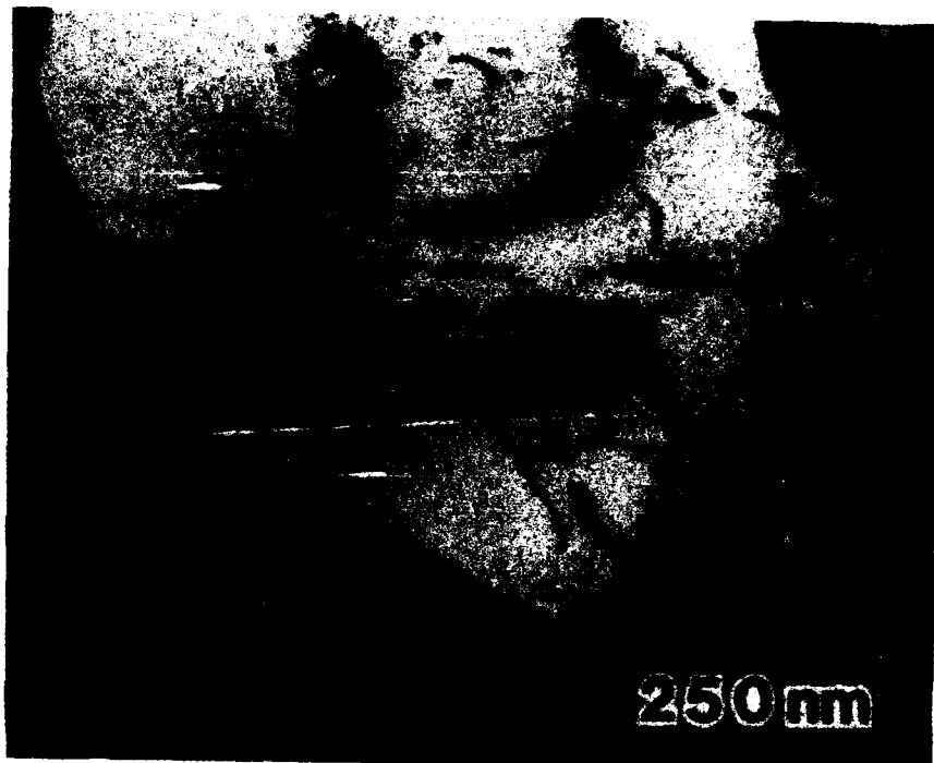
Figure 3.33 Bright field TEM micrograph of Nb-10Al-10Cr-10Ti (alloy H7) melt-spun ribbon after heat treatment at 600°C for 1 hour.
