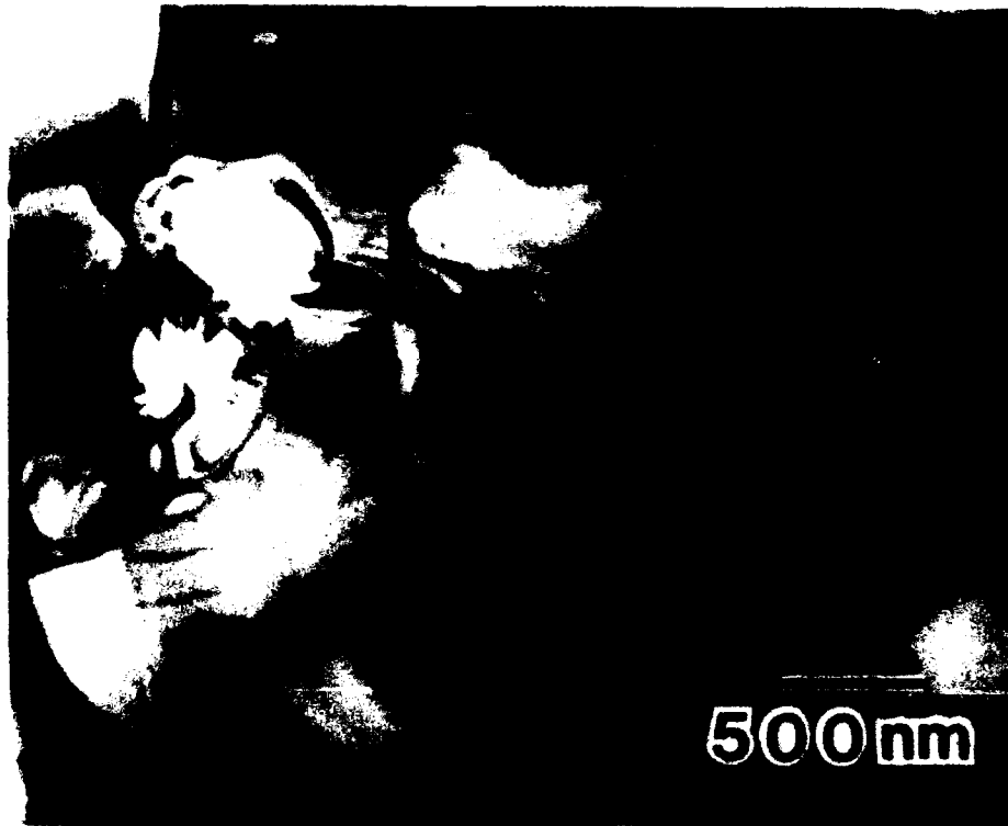
Figure 3.44 Bright field TEM micrograph of as-melt spun Nb-10Al-10Cr-10Ti-10W-1Zr (alloy S4).
