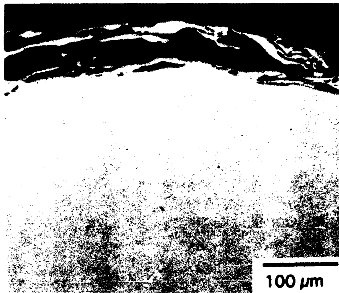
Figure 4.46 Cross sectional optical micrographs of Alloy 17 ( Nb-20Ta-15Cr ) after cyclic oxidation at 800°C for 140h. The lack of Ti in the alloy harms oxidation resistance and resulted in massive spallation.
