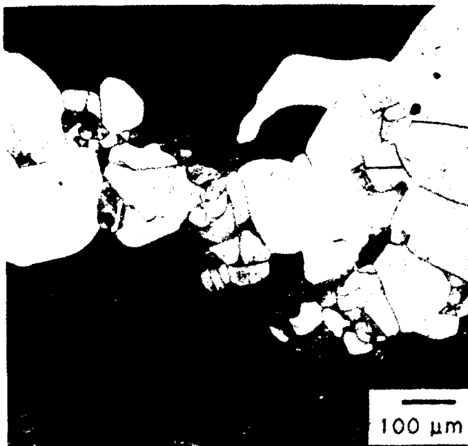
Figure 5.22 Optical micrographs of specimens from Alloy 12 which had been heat treated at a) 1000°C / 24h, b) 1000°C / 4h plus 500°C / 24h, c) 1000°C / 4h plus 600°C / 24h, and d) 1000°C / 4h plus 700°C / 24h.
