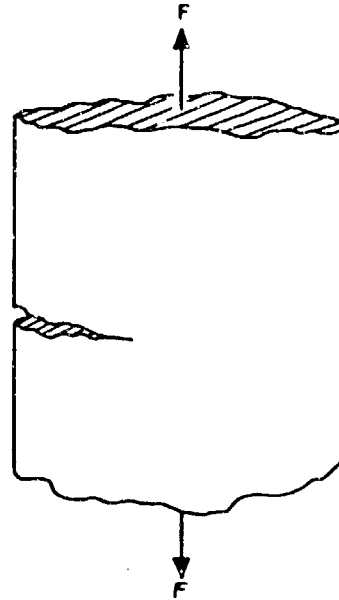
Figure 16.3 Stress Corrosion Cracking
