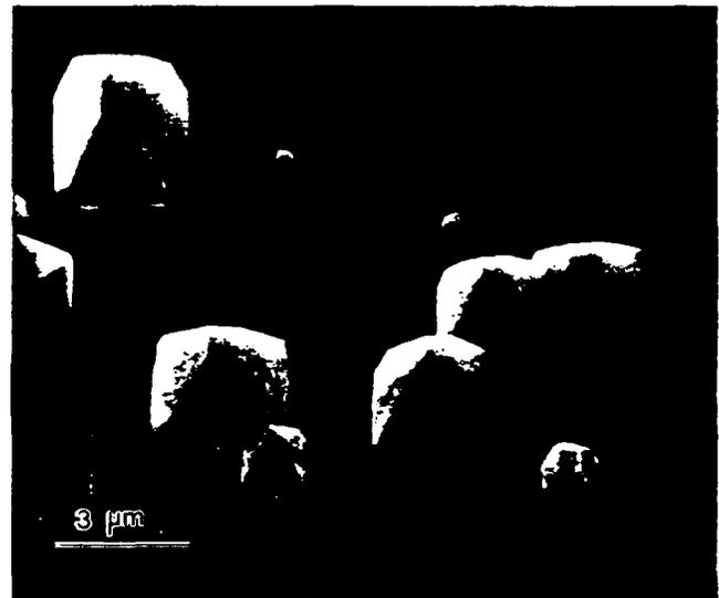
FIG. 3. SEM of the center region taken at a  $45^\circ$  tilt to show (111) faceting.
