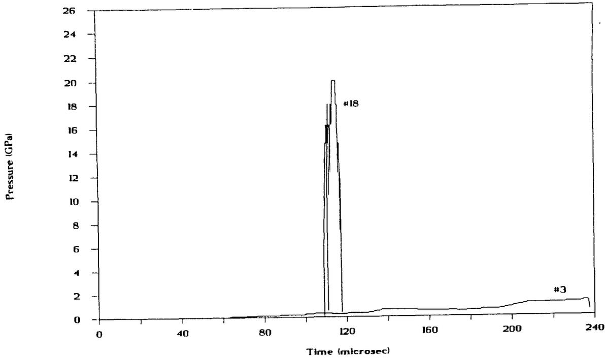
Figure 5. Carbon resistor gauge records for nose-only detonations.
