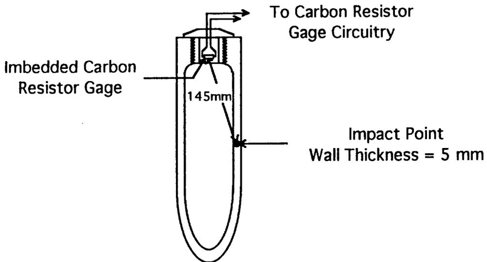
Figure 2. Cross-section view of a carbon resistor gage in a 105-mm HEP-T warhead.
