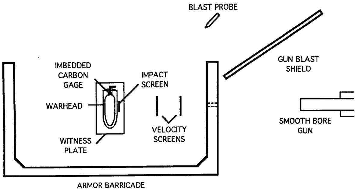
Figure 1. Experimental arrangement (overhead view).
