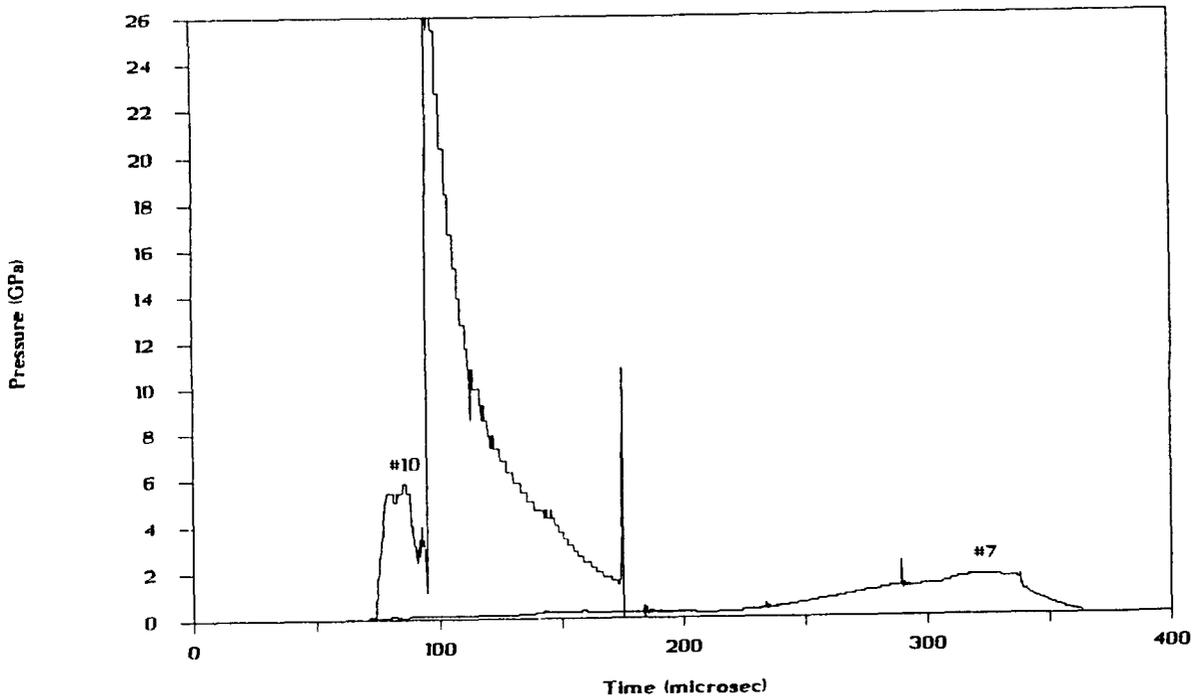
Figure 6. Carbon resistor gauge records for nondetonations.
