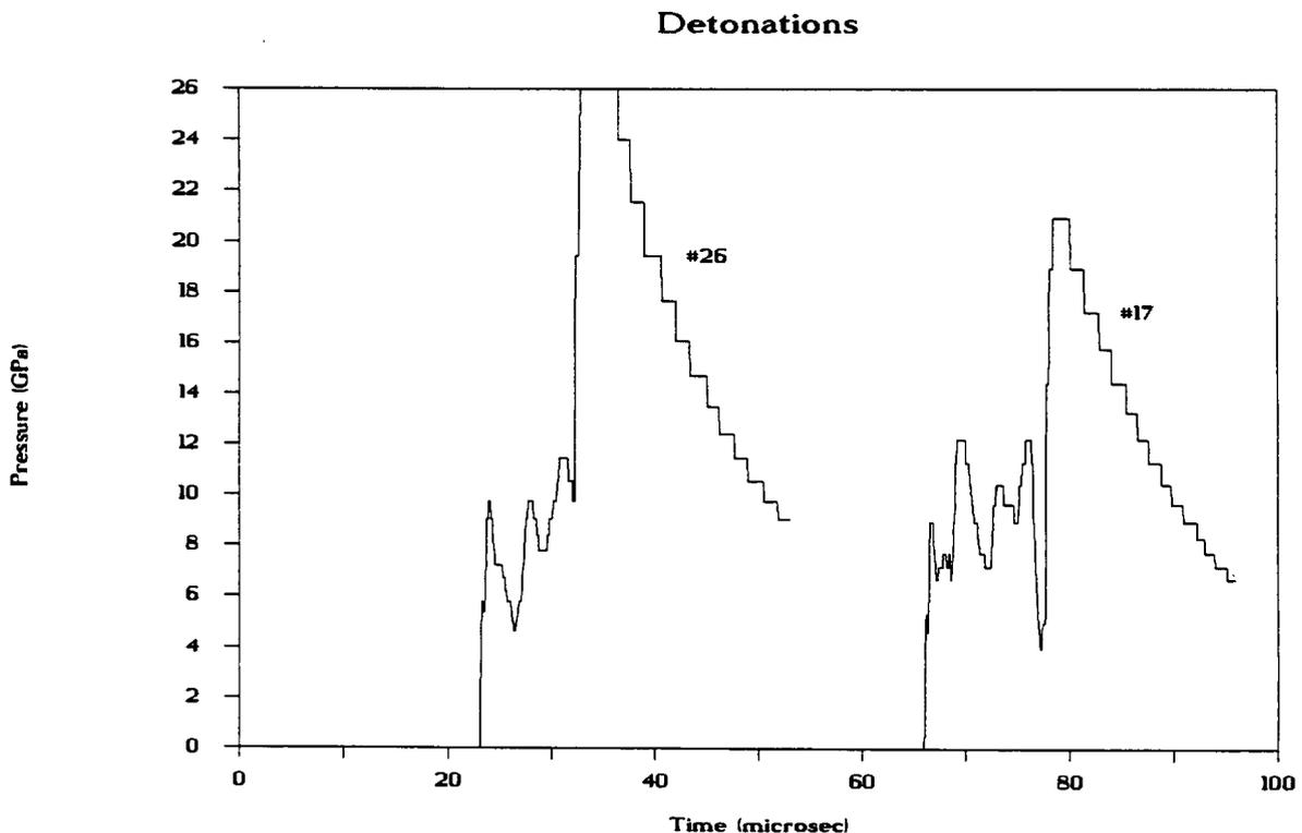
Figure 4. Carbon resistor gauge records for detonation.
