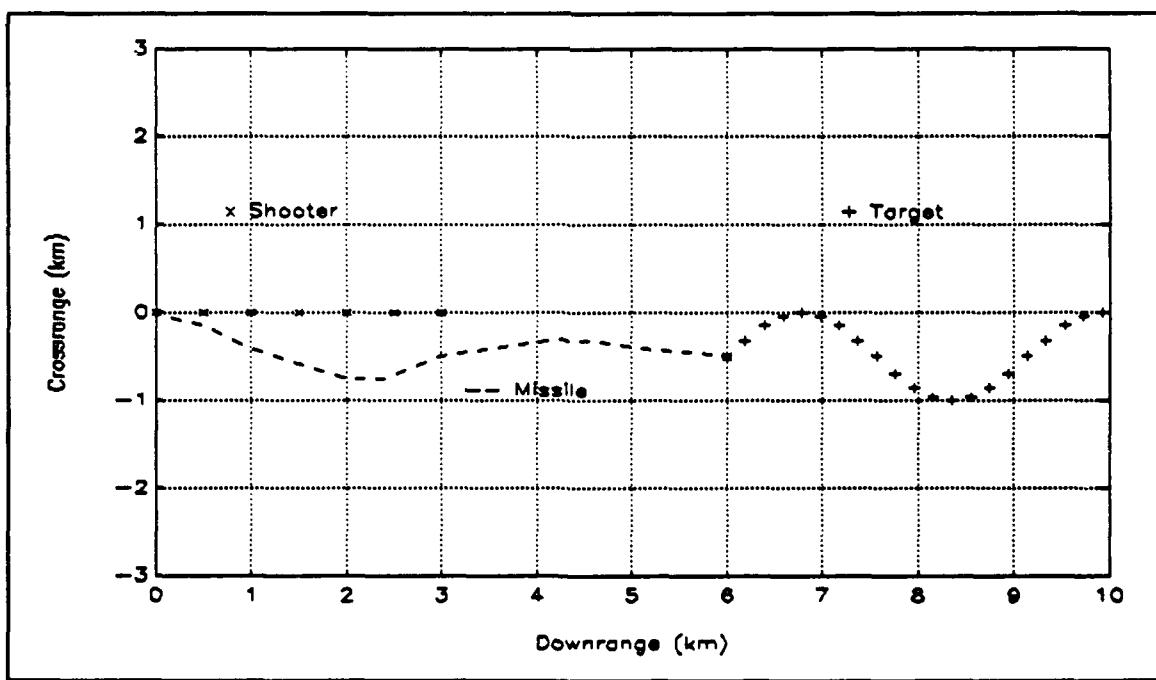
Figure 13 Head-on Shot Against a Maneuvering Target
