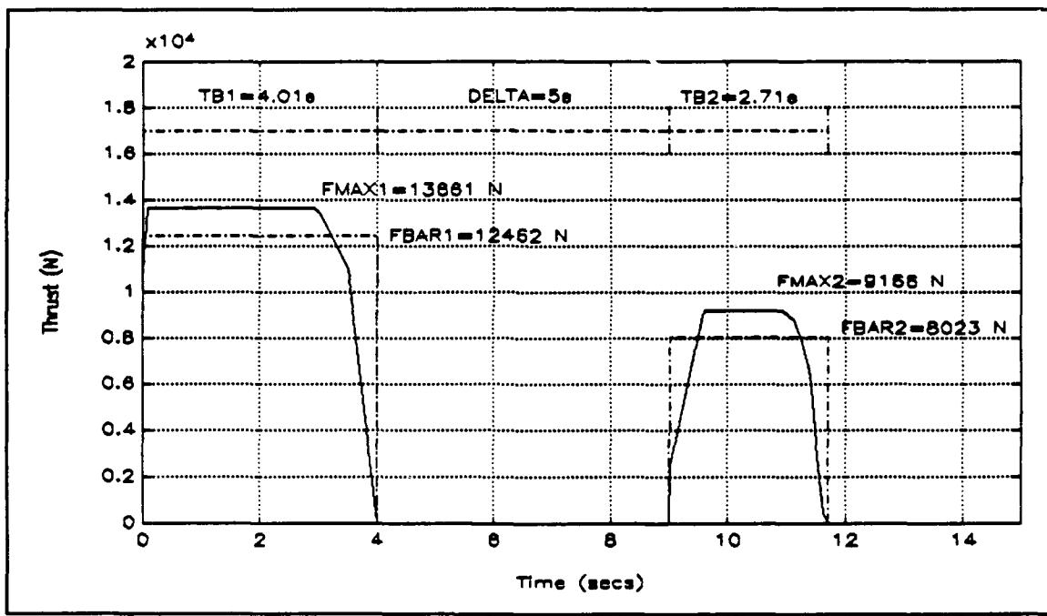
Figure 11 Typical DIT Thrust-Time Profile
