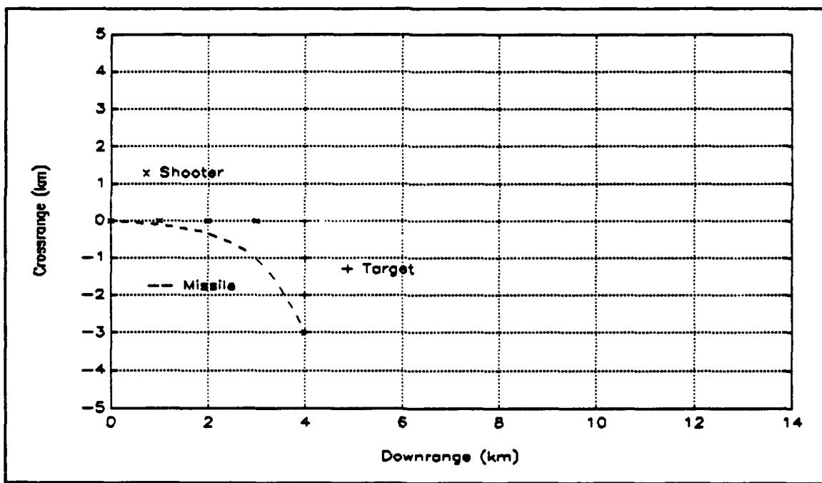
Figure 16 Beam Shot Against a Non-Maneuvering Target
