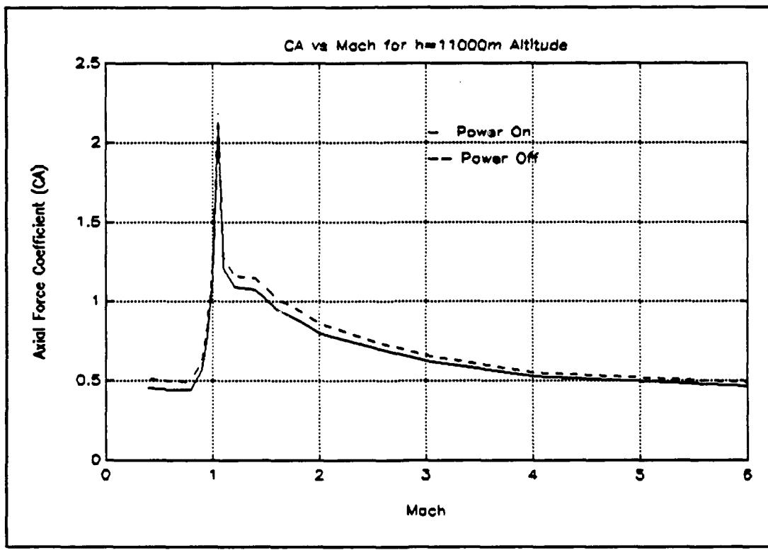
Figure 5 CA vs Mach for Generic SRAAM,  $h=11000\text{ m}$
