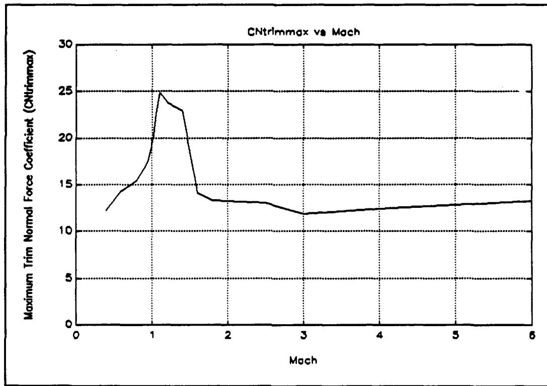
Figure 7 CNtrimmax vs Mach for generic SRAAM
