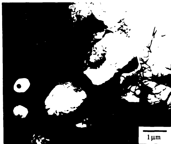
Figure 1. TEM micrograph of typical HIPed Cerac MoSi 2 powder, showing SiO 2 (light phase) and Mo 5 Si 3 (dark phase).
