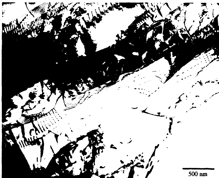
Figure 42. TEM micrograph showing high density of subgrain boundaries in an MoSi 2 grain in compressed MoSi 2 + Ti.
