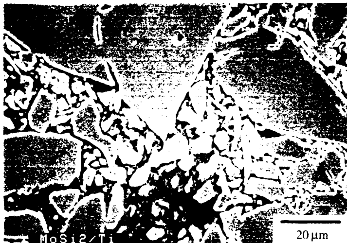
Figure 38. Typical distribution of phases in HIP reacted MoSi 2 + 10 vol% Ti.
