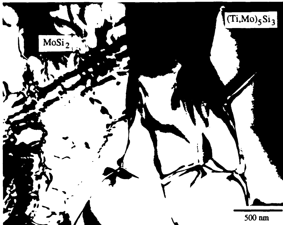
Figure 41. TEM micrograph of HIP reacted MoSi 2 + Ti compressed at 1300°C.
