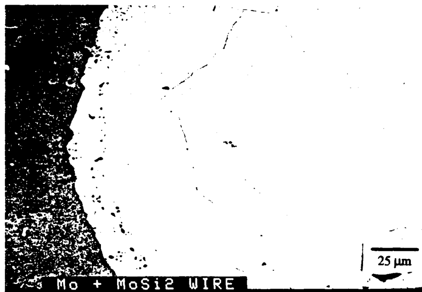
Figure 18. Mo wire in MoSi 2 HIPed at 1700°C/4 h.
