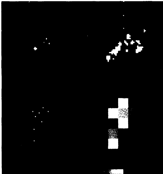
FIGURE 21. Target feature extraction and spatial coding for a single target. The upper left quadrant shows the input slant-plane image of a target at a depression angle of 15^\circ . In the upper right quadrant, feature blobs have been extracted from the input image and projected in the ground plane. After the feature blobs are reoriented in the target frame of reference, a DEB network is used to reduce the blobs to points, as shown in the lower left quadrant. The feature points are then coarsely coded by a 9 \times 9 array of overlapping receptive fields (cf. Figure 7), as shown in the lower right quadrant. The color bar at the bottom of the figure denotes increasing (from black to white) reflectivity for the upper left image, and increasing receptive-field activity for the lower right image.
