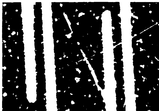
Fig. 8. Photomicrograph of a Au/Cr striped anode, backlighted to reveal voids. The dark stripes are metal, the white stripes are quartz. The thin ( 25\text{ }\mu\text{m} ) metal stripes are only voided at their edges. 200\times .
