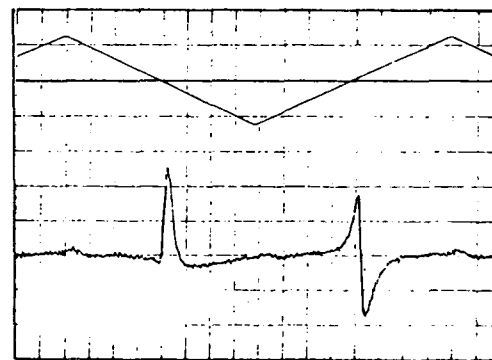
Fig. 4: Transmitted light, triangle-wave modulation. Total time is 50mS, slope is 40gs/sec.
