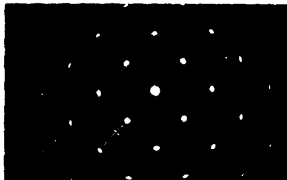
Figure 3(b). Transmission electron diffraction pattern from the film with the beam along the film normal i.e. along Ag[001]. Ag(200) indicated.
