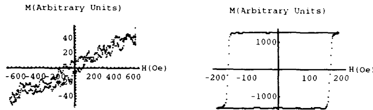
Fig.2: Longitudinal (left) and polar (right) M-H loops for 35 Å Ni/3000 Å Cu/Si(100).
