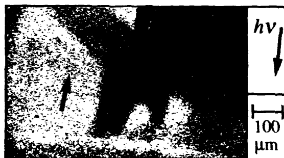
Fig. 4: Domain image from an "L"-shaped Fe(100) whisker using L_3VV Auger electrons (703 eV kinetic energy). Photon energies and helicity as in Fig. 3. Arrows mark the orientation of magnetization in individual domains.
