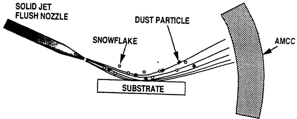
Figure 20 Advanced contamination removal and collection system incorporating the jet spray, ion beam and AMCC.
