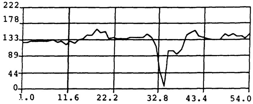
Figure 13 MacPhase profile of typical microabrasion of Figure 10.
