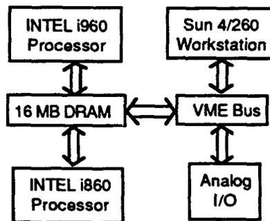
Fig. 8 - Real-time emulation of 800-b/s Voice Encoder
