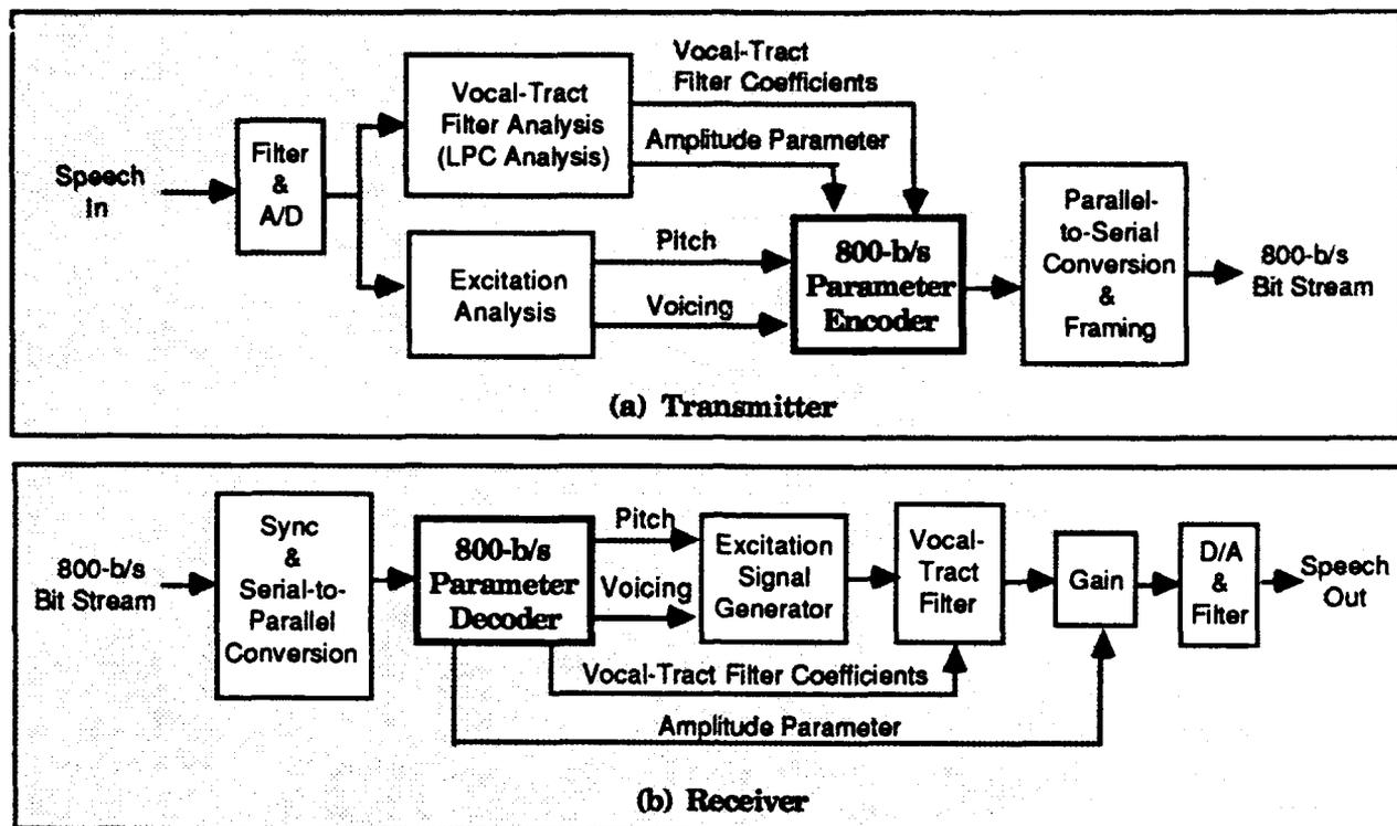
Fig. 1 - Block diagram of 800-b/s voice encoder. The general layout of computational blocks are identical to that of the 2400-b/s LPC. The only blocks unique to the 800-b/s voice encoder are the parameter encoder and parameter decoder identified by heavy-lined blocks. Since the other blocks are well-known, we will not elaborate further on them.
