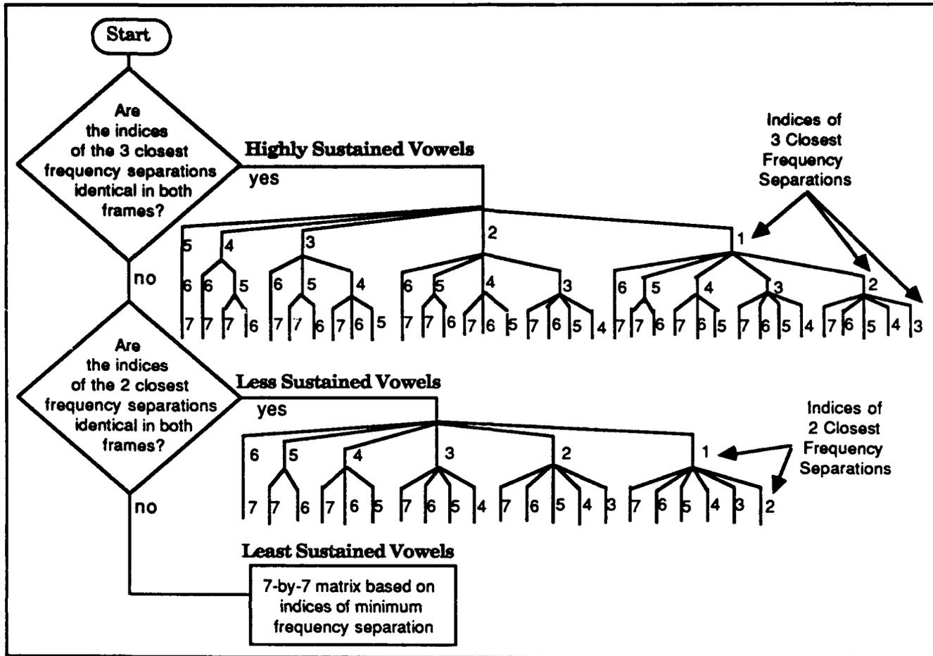
Fig. 7 - Filter coefficient partition for Case 4 (both frames are voiced)
