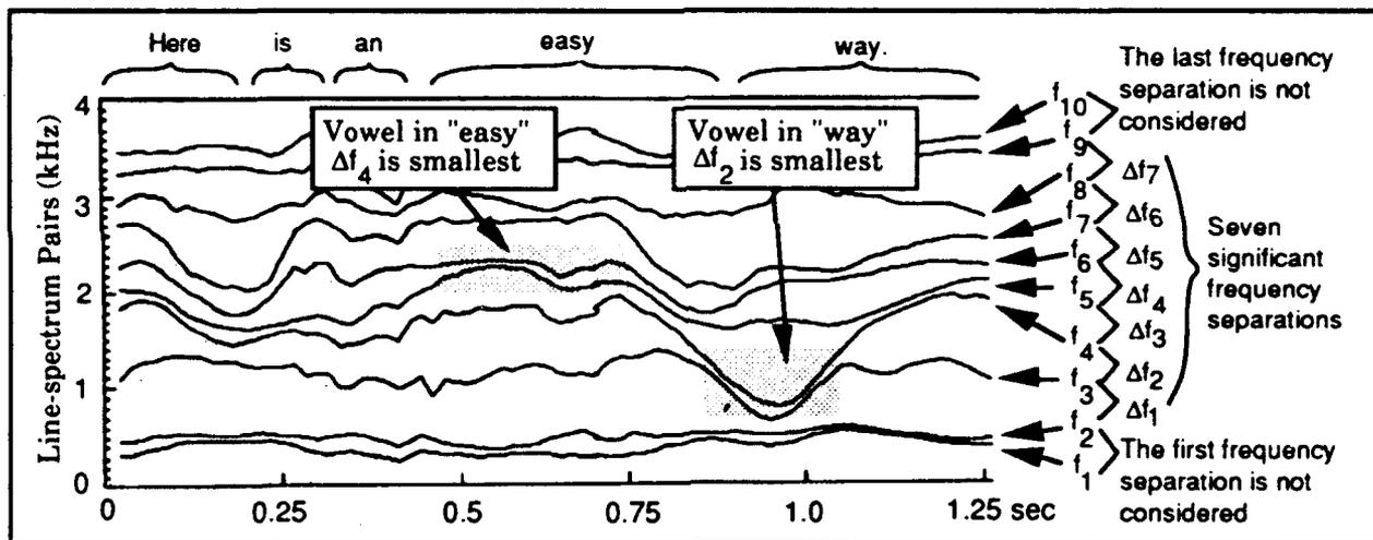
Fig. 5 - Seven significant frequency separations in LSP trajectories. The first and last frequency separations are not considered because they are more or less stationary, therefore, they not too useful for LSP partition.
