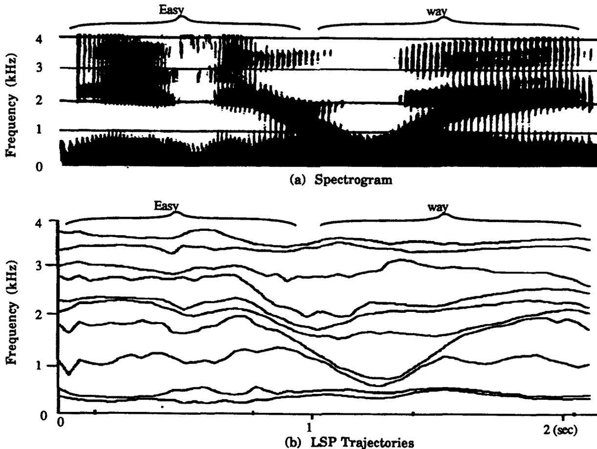
Fig. 3 - Comparison of spectrogram and LSP trajectories derived from the same speech. As noted, line-spectrum frequencies are close together where formant frequencies are located.
