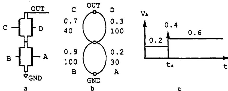
Figure 2. (a) A CMOS gate; (b) Graph of the n-part; (c) Input waveform.
