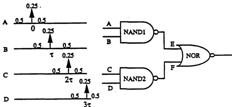
Figure 4. A test CMOS combinational circuit and the input statistical descriptions.  $t_{HL}$  and  $t_{LH}$  are both  $0.2\text{ns}$  for each input event. Simulation period  $T = 20\text{ns}$ .
