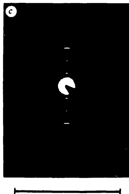
FIG. 3 Optical micrograph, taken with crossed polarizers, of the small-molecule liquid crystalline compound 4-cyano-4'- n -hexylbiphenyl (K 18, BDH Ltd) grown on a glass substrate that was coated with a thin layer of PTFE in a helical pattern. In this case a continuous, nonlinear structure was produced by moving a pencil-shaped PTFE rod in a spiralling path across the glass substrate. The liquid crystalline compound was then applied to the decorated substrate. This optical micrograph shows that the liquid crystalline material formed domains with a continuously changing director following the orientation of the underlying PTFE layer. Scale bar represents 1 mm.
