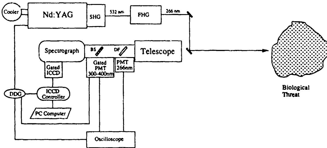
FIGURE 1: UV Fluorescence Lidar System
