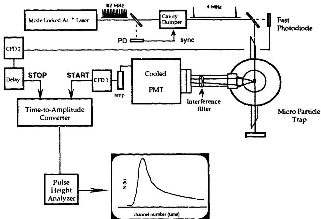
**Figure 1.** Schematic of experimental apparatus used to measure R6G fluorescence lifetimes in levitated microdroplets.
