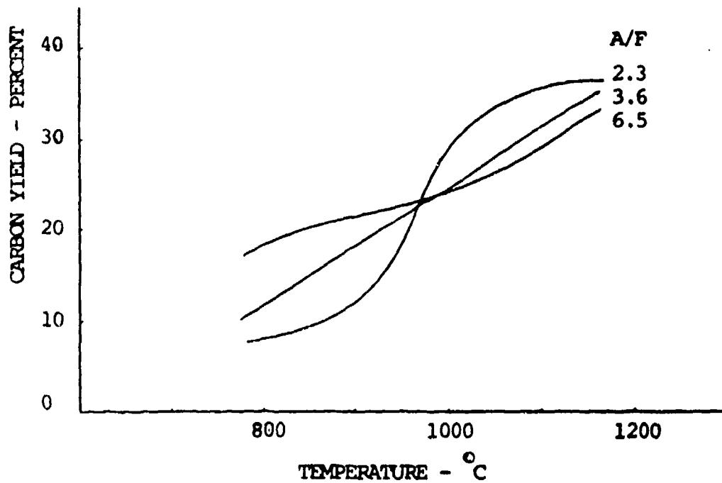
Figure 2. Effect of temperature on carbon yield.
