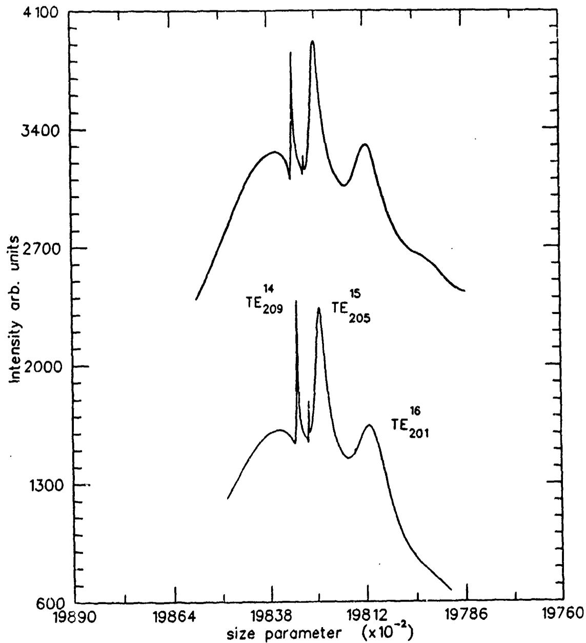
Figure 2. Experimental scattering curve of a glycerin/methanol droplet evaporating from  $r = 15.41$  to  $15.37 \mu\text{m}$  (top) along with the corresponding theoretical curve for  $n=1.4722$  and  $k=0.0$  (bottom).
