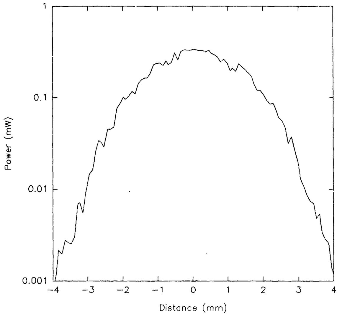
Figure 4b. Scan of the incident beam for a wavelength of  $1.06 \mu\text{m}$  and a receiver aperture of  $1.07 \text{ mm}$ .
