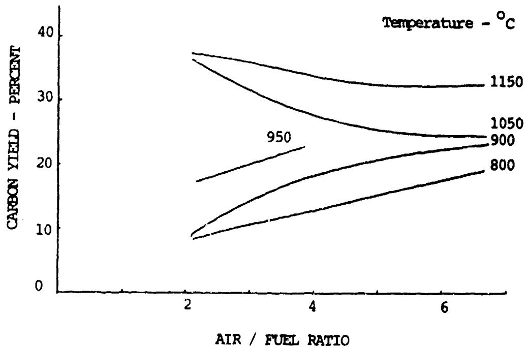
Figure 3. Effect of air/fuel ratio on carbon yield.
