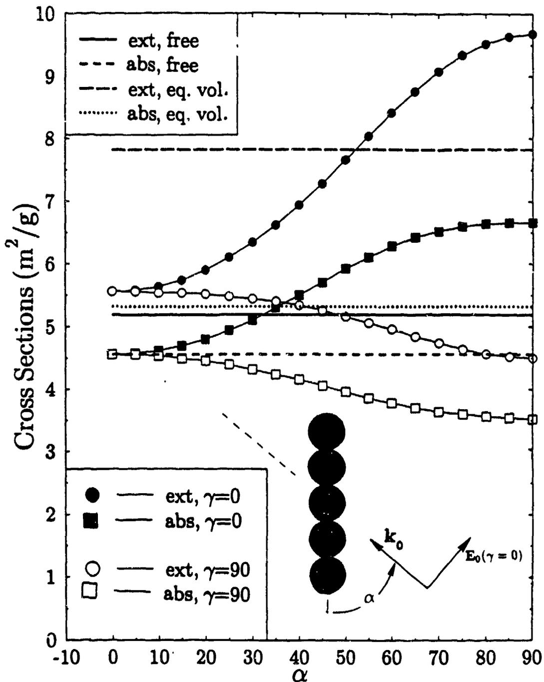
Figure 11. Extinction and absorption cross sections of a linear chain of five carbon spheres. Each of the monomers has a radius of  $0.05 \mu\text{m}$  and a refractive index of  $1.8 + 0.5i$ .
