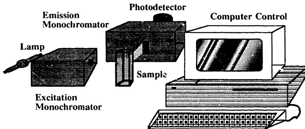
**Figure 1:** Experimental set-up. The light is from a continuous xenon arc lamp. The excitation wavelength is selected by a monochromator with a 10 nm bandwidth. This light is imaged onto the bacterial suspension in a quartz cuvette. The fluorescence is collected at 90° and passes through a second monochromator with 10 nm bandwidth. The fluorometer and subsequent data analysis is all under computer control.
