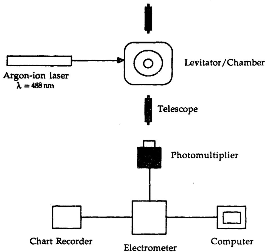
Figure 1. Experimental apparatus used to detect suppression of MDR's in microdroplets
