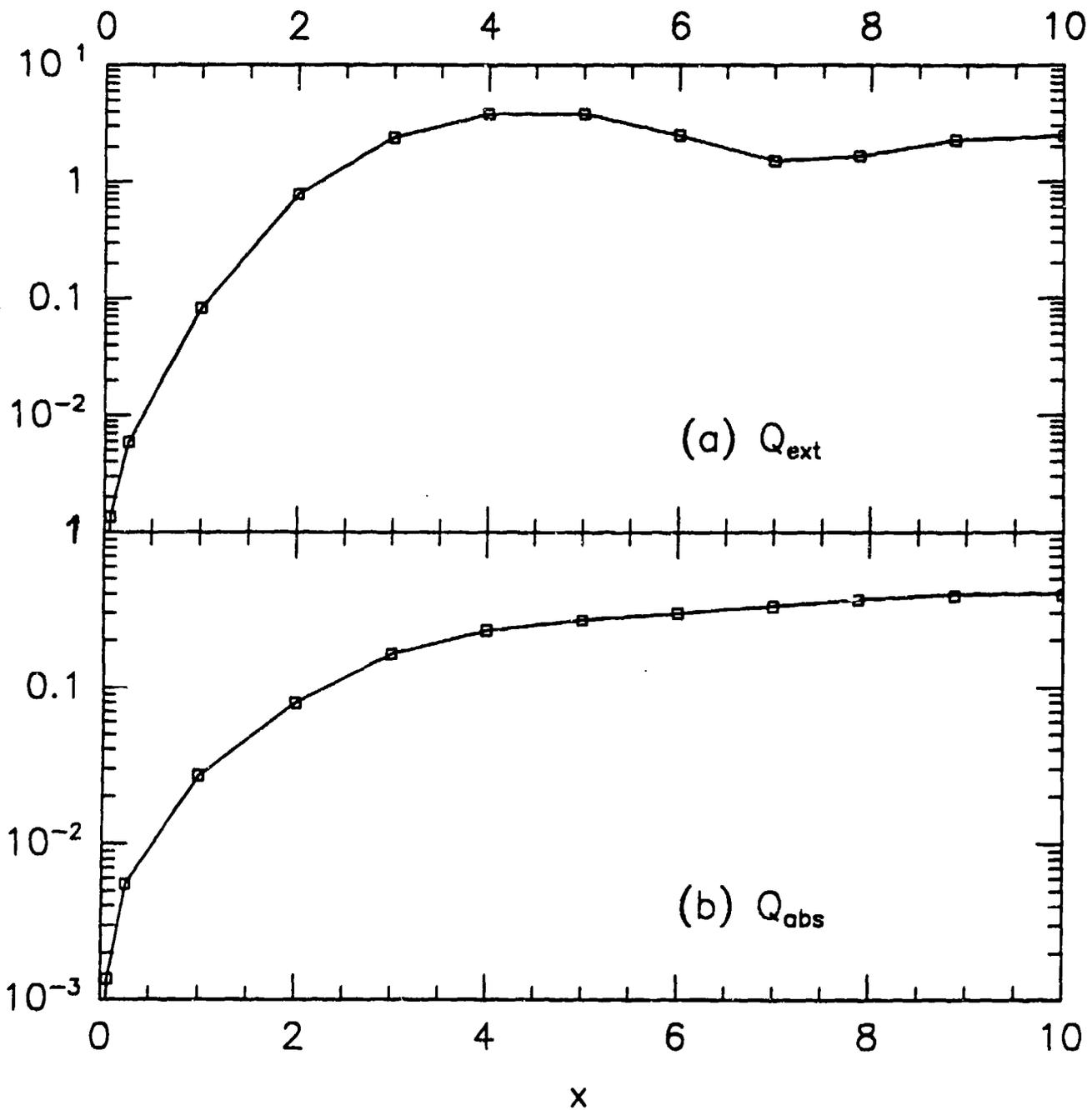
Figure 4. Comparison of extinction and absorption efficiencies of the particles discussed in Figs. 2 and 3 as a function of the size parameter of the equivalent-volume sphere. To obtain these efficiencies, the respective cross sections were normalized by the geometric cross section of the equivalent-volume sphere.
