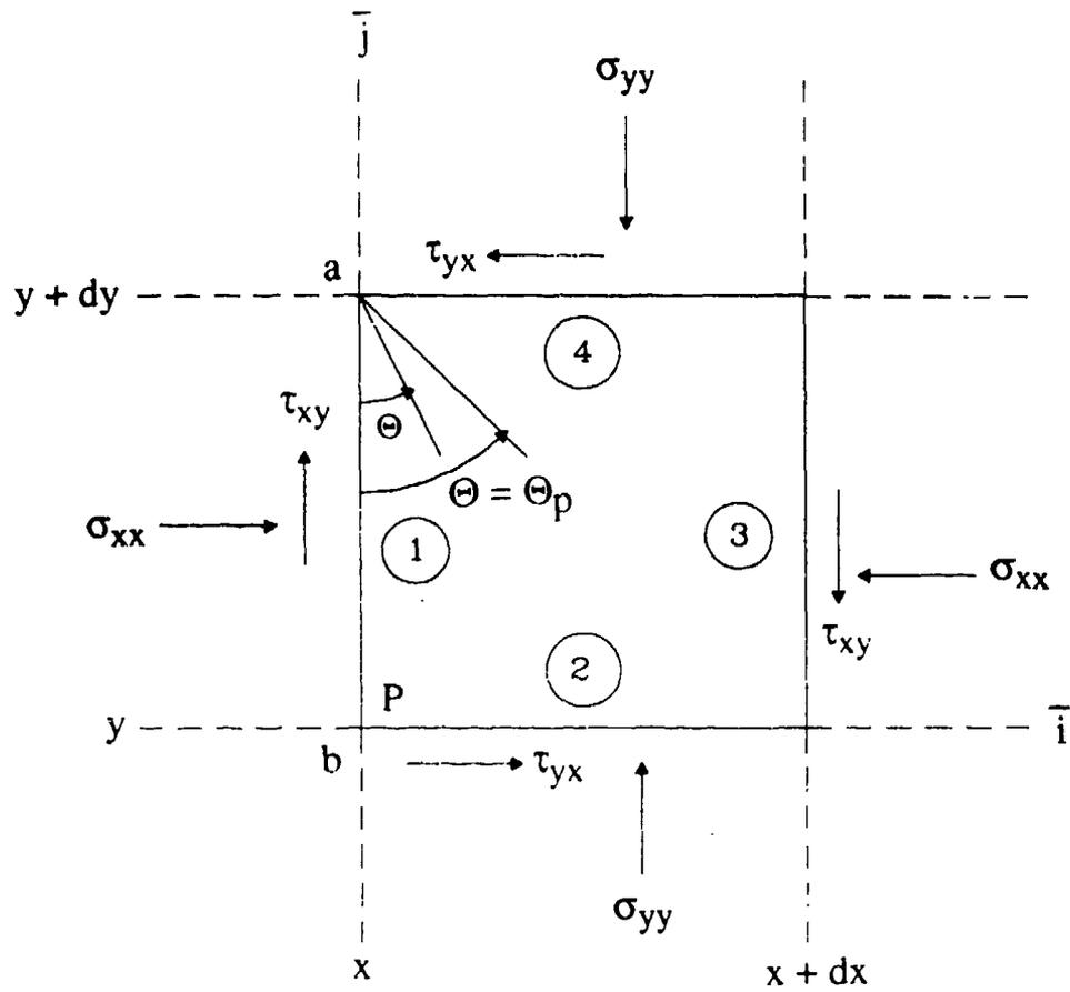
**Fig 1b** Stresses on Element of Bulk Powder Oriented Parallel and Perpendicular to the  $\bar{i}$  and  $\bar{j}$  Coordinate Axes Located at Point P.
