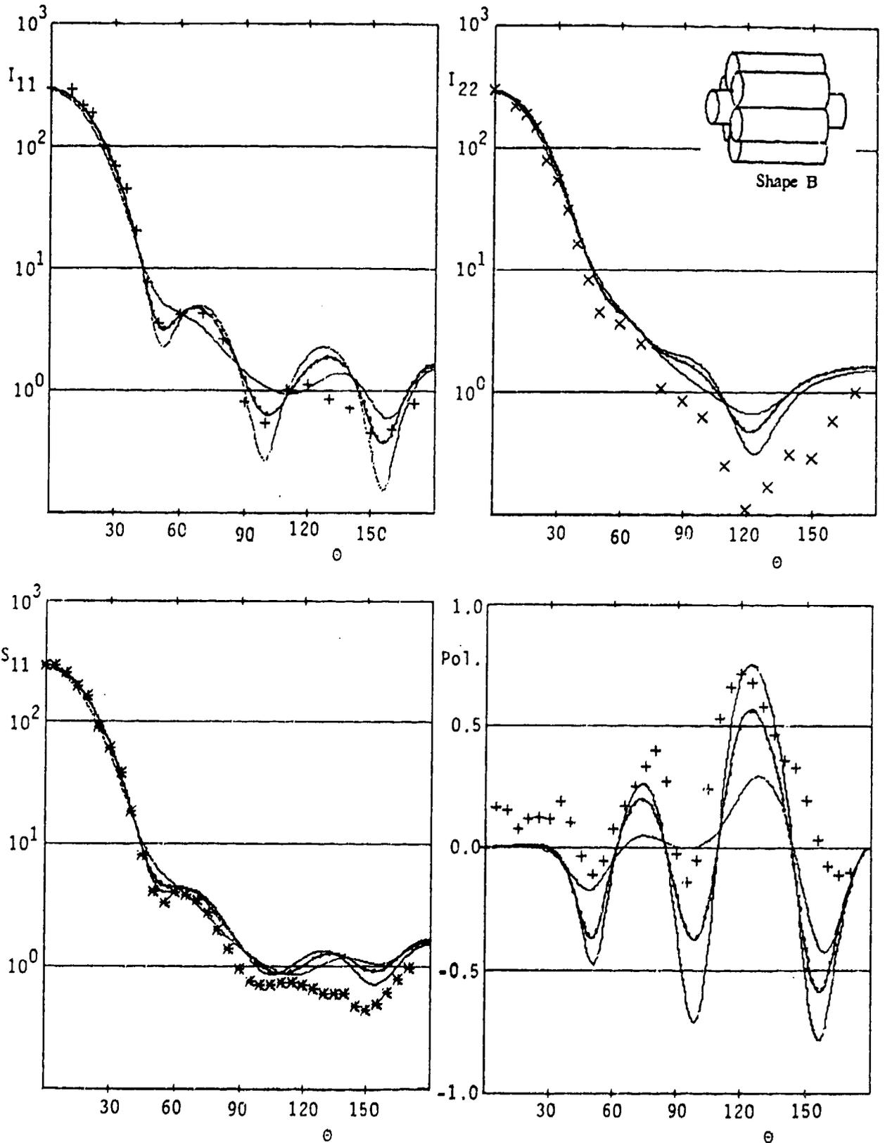
Figure 3 Microwave Angular Scattering Data (symbols) Averaged Over Random Orientations of a Rough Particle with  $x = 4.257$  and  $m = 1.366 - i0.005$ . Curves show the averaged Mie data over gamma-size-distributed spheres. 3 effective variances of the distributions are employed:  $b = 0.001$ ,  $b = 0.005$  (marked as ----) and  $b = 0.025$ .
