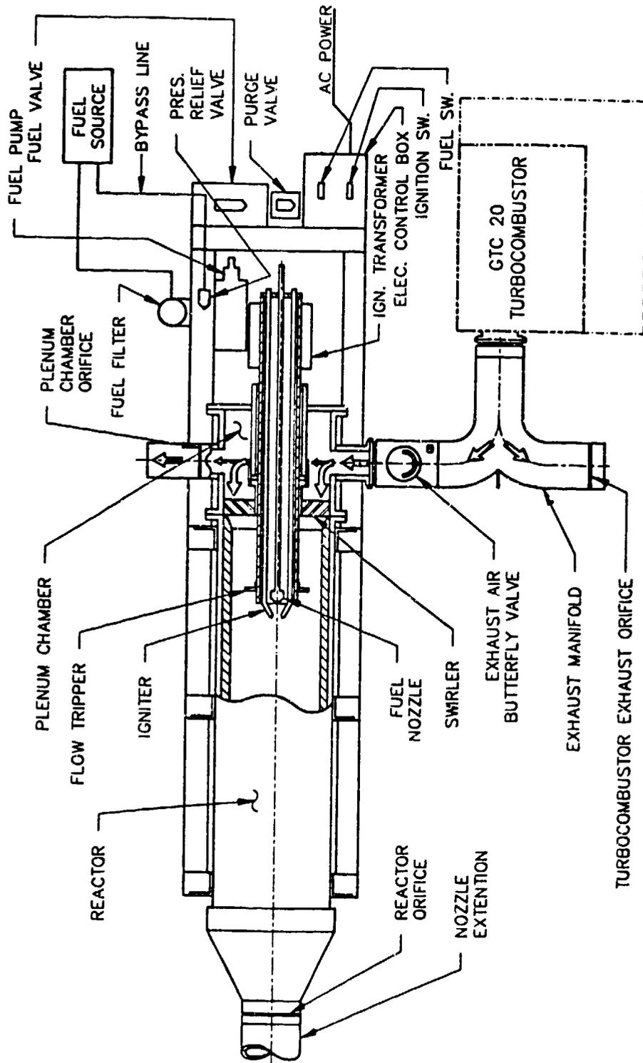
Figure 5. Integrated turbocombustor/prototype carbon particle generator.
