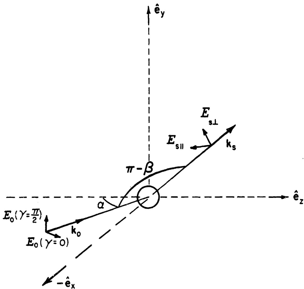
Figure 1. The reduced-symmetry geometry for light scattering by a sphere.
