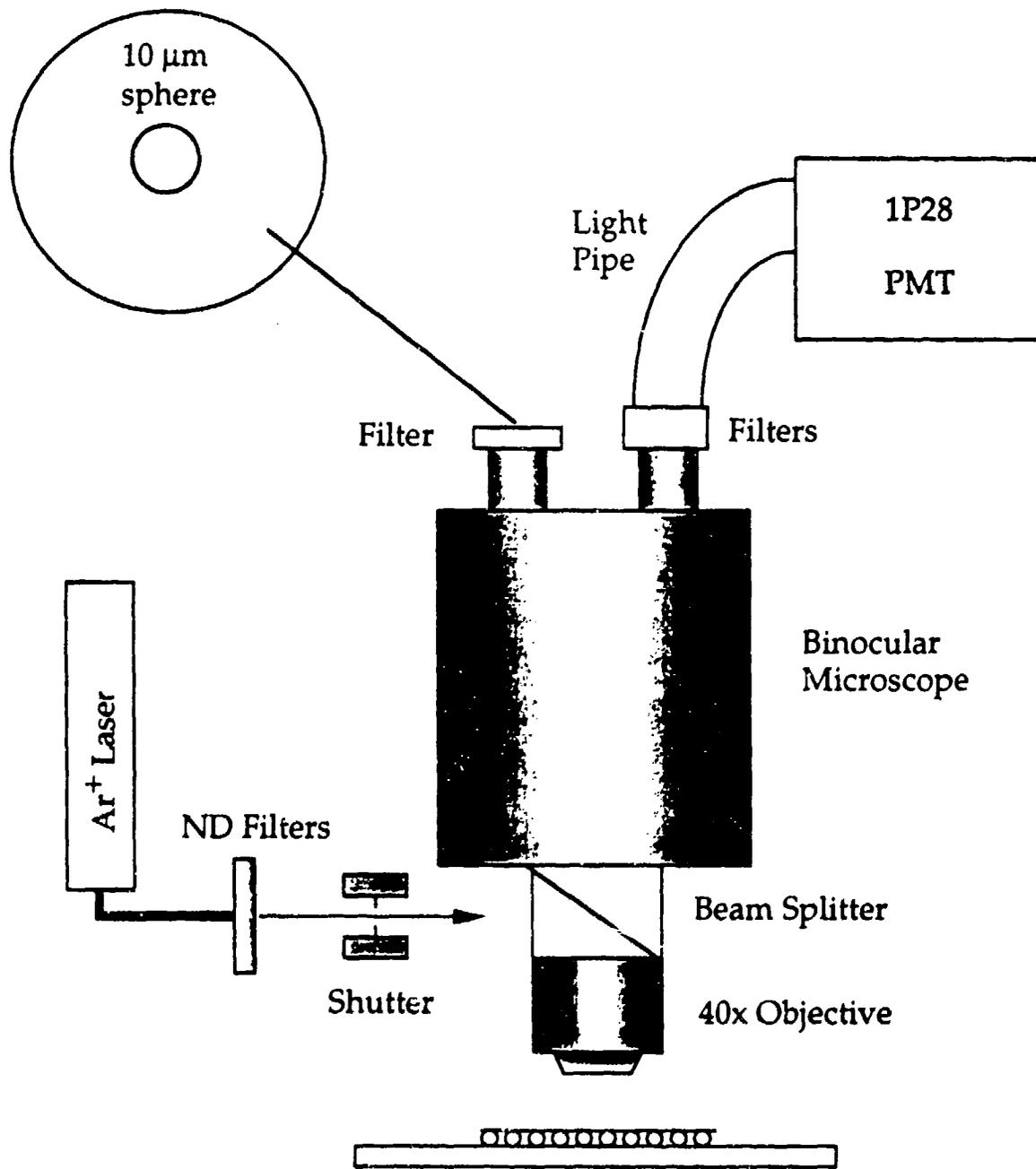
Fig. 1. Apparatus for measuring fluorescence of individual microspheres.
