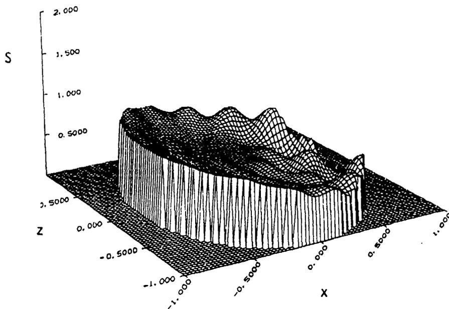
FIGURE 5. Internal normalized source function distribution in the  $x$ - $z$  plane for a plane wave incident on a homogeneous 1.3 to 1.0 axis ratio prolate spheroid. ( $\alpha = 10$ ,  $\bar{n} = 1.18 + 0.07i$ ,  $\theta_{bd} = 90^\circ$ ,  $\phi_{bd} = 0^\circ$ )
