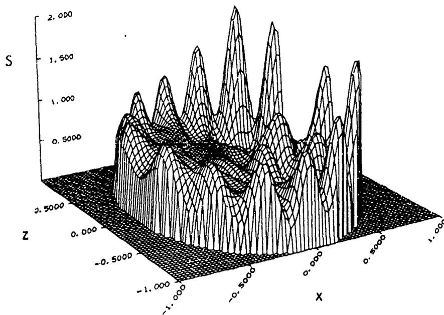
FIGURE 6. Internal normalized source function distribution in the  $x$ - $z$  plane for a plane wave incident on a layered 1.3 to 1.0 axis ratio prolate spheroid. ( $\alpha = 10$ ,  $\bar{n}_1 = 1.18 + 0.07i$ ,  $\bar{n}_2 = 1.48 + 0.0055i$ ,  $\bar{a}_{12} = 0.9$ ,  $\theta_{bd} = 90^\circ$ ,  $\phi_{bd} = 0^\circ$ )
