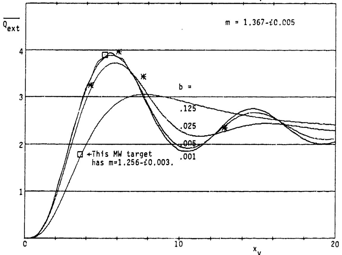
Figure 1 Extinction Efficiency  $\overline{Q_{ext}}$  vs Volume-Equivalent Size Parameter  $x_v$ . The microwave data (symbols) are the averaged data over random orientations of each rough particle. Curves show the averaged Mie data over gamma-size-distributed spheres, several values of the effective variance  $b$  employed for the distributions are as shown.
