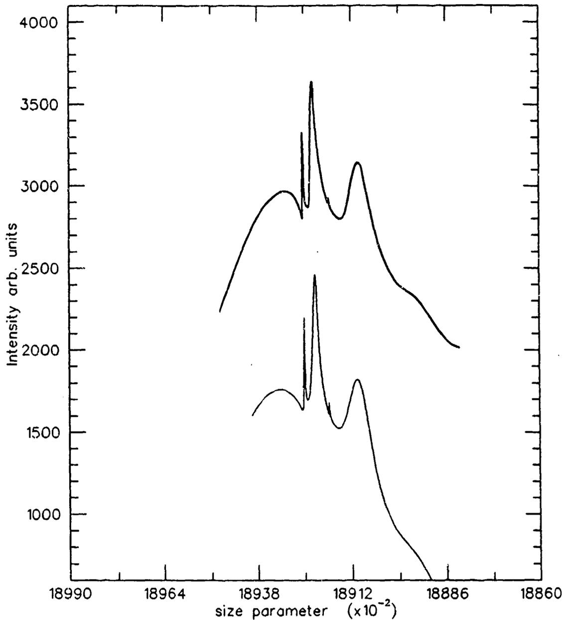
Figure 8. Experimental scattering curve of a glycerin/methanol droplet evaporating from  $r = 14.71$  to  $14.68 \mu\text{m}$  (top) along with the corresponding theoretical curve for  $n=1.4722$  and  $k = 2.6e-6$  (bottom).
