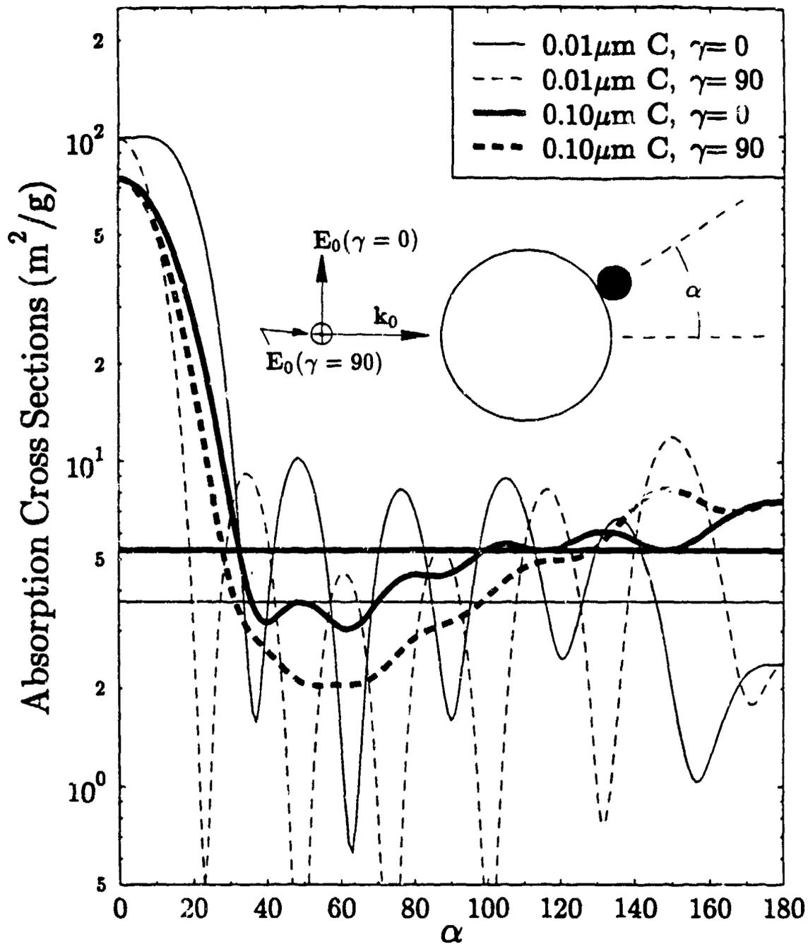
Figure 4. Same as Figure 3, but with either a  $0.1$  or  $0.01 \mu\text{m}$  carbon grain. The heavy and light lines show the absorption cross sections of isolated  $0.1$  and  $0.01 \mu\text{m}$  grains, respectively. The inset is drawn to scale for the  $0.1\mu\text{m}$  carbon sphere.
