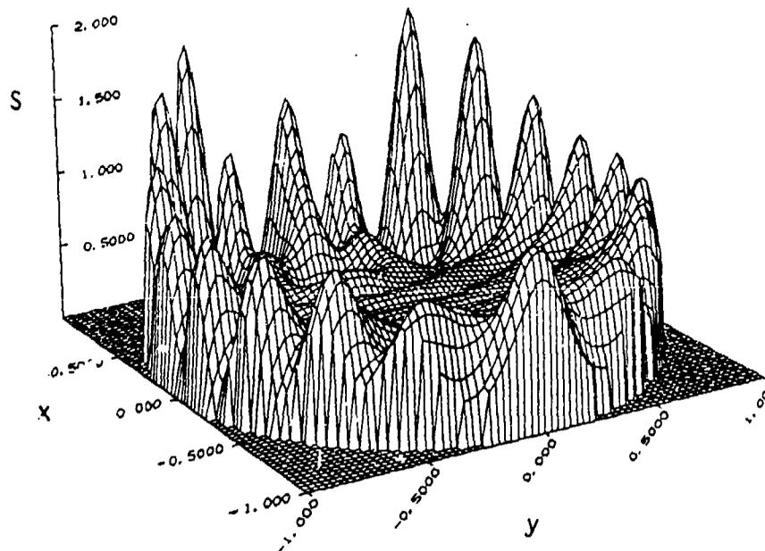
FIGURE 8. Internal normalized source function distribution in the x-y plane for a plane wave incident on a layered circular cylinder. ( $\alpha = 10$ ,  $\bar{n}_1 = 1.18 + 0.07i$ ,  $\bar{n}_2 = 1.48 + 0.0055i$ ,  $\bar{a}_{12} = 0.9$ ,  $\theta_{bd} = 0^\circ$ ,  $\phi_{bd} = 90^\circ$ )
