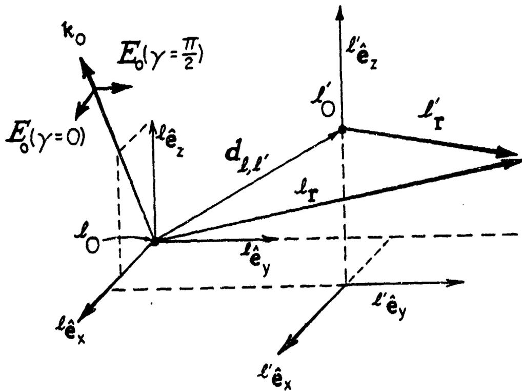
Figure 2. The scattering geometry for multiple scattering centers.
