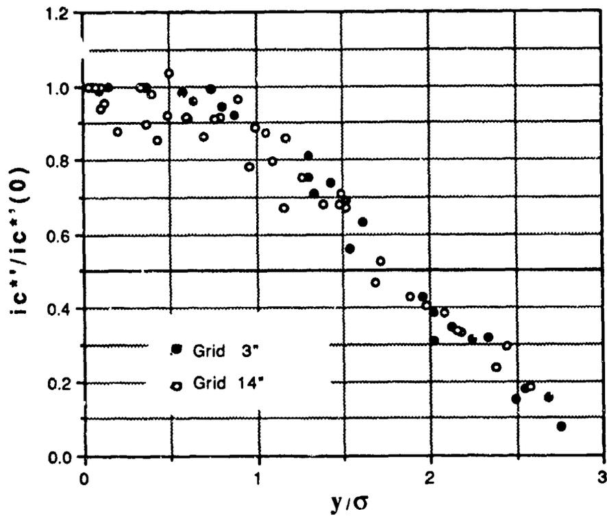
Figure 4. Comparison of the lateral distributions of the relative rms of the fluctuation,  $ic^{**}/ic^{**}(0)$ , downwind of the 14 in. grid ( $2.07 \leq x/M \leq 17$ ) and the 3 in. grid ( $20 \leq x/M \leq 102$ ).
