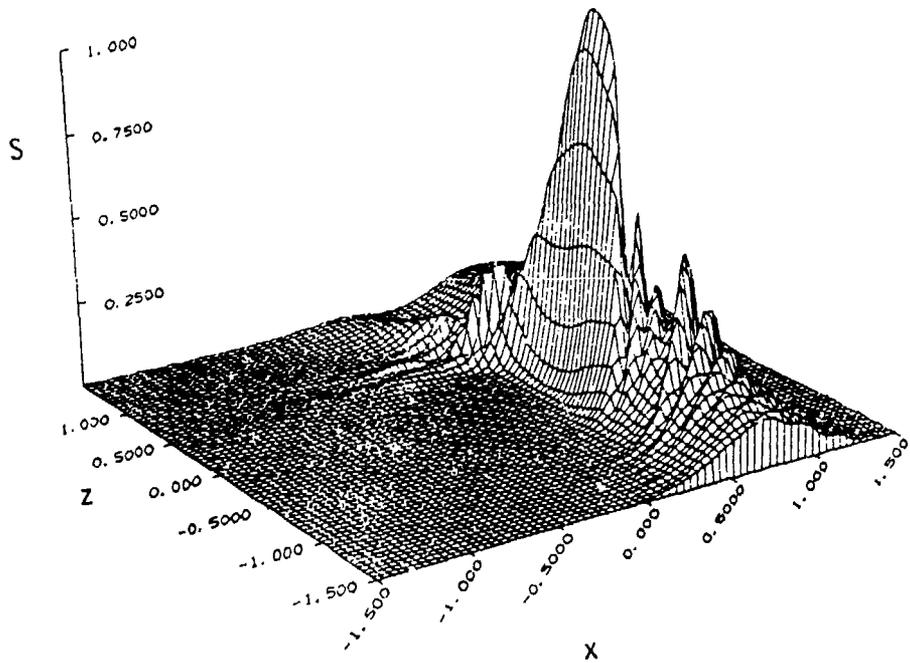
FIGURE 2. Normalized source function distribution in the x-z plane for a beam focused on a layered sphere. ( $\alpha = 30$ ,  $\bar{n}_1 = 1.33 + 1.0 \times 10^{-6}i$ ,  $\bar{n}_2 = 1.1 + 1.0 \times 10^{-6}i$ ,  $\bar{a}_{12} = 0.7$ ,  $\bar{w}_0 = 0.2$ ,  $\bar{x}_0 = 0.7$ ,  $\bar{y}_0 = 0.0$ ,  $\bar{z}_0 = 0.0$ ,  $\theta_{bd} = 0^\circ$ ,  $\phi_{bd} = 90^\circ$ )
