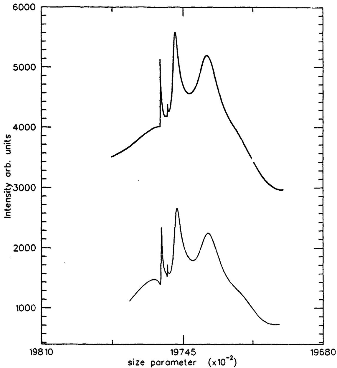
Figure 7. Experimental scattering curve of a glycerin/methanol droplet evaporating from  $r = 15.35$  to  $15.31 \mu\text{m}$  (top) along with the corresponding theoretical curve for  $n=1.4722$  and  $k=2.5e-6$  (bottom).
