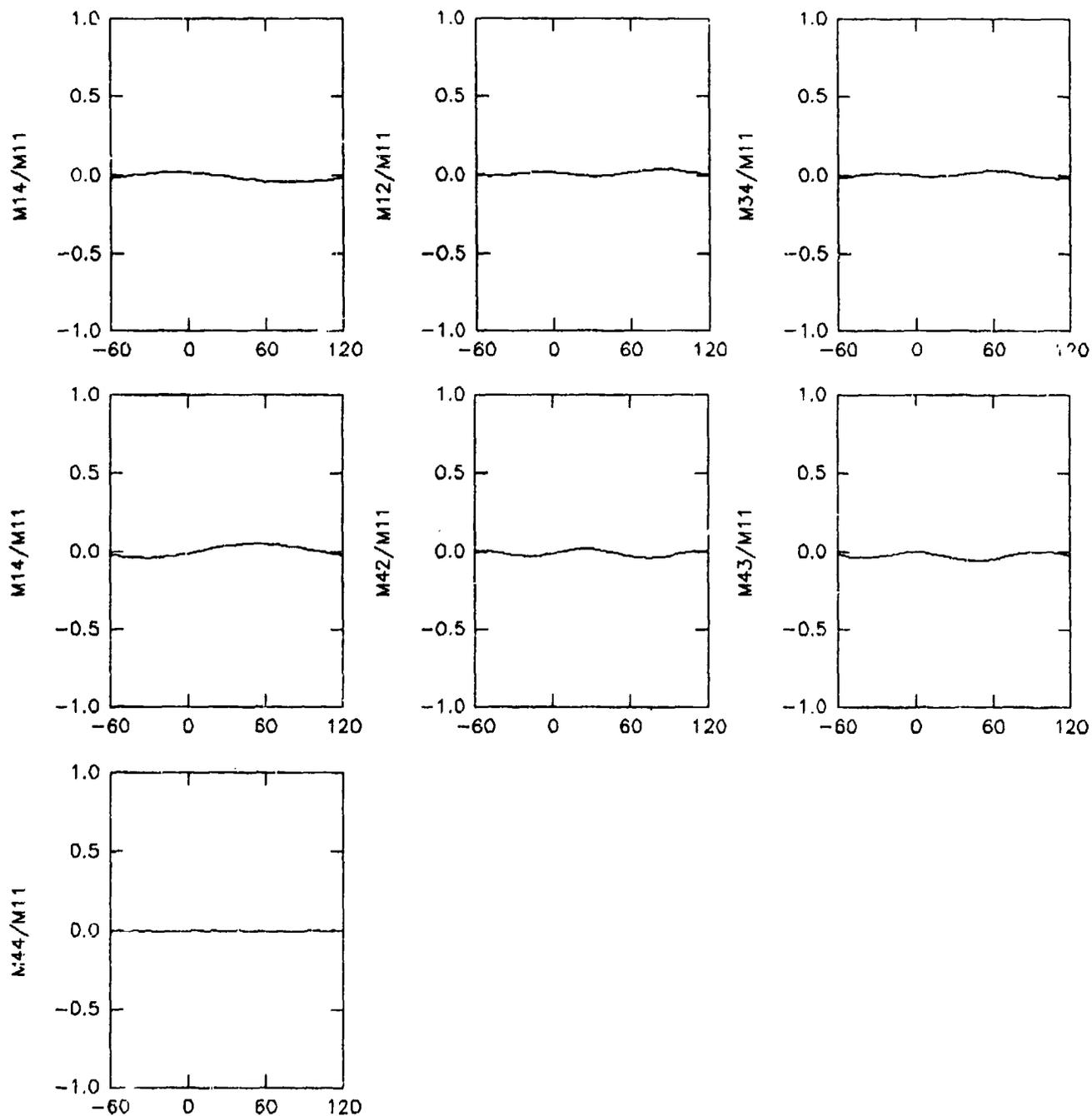
Figure 5b. Muller matrix elements for a polarizer
