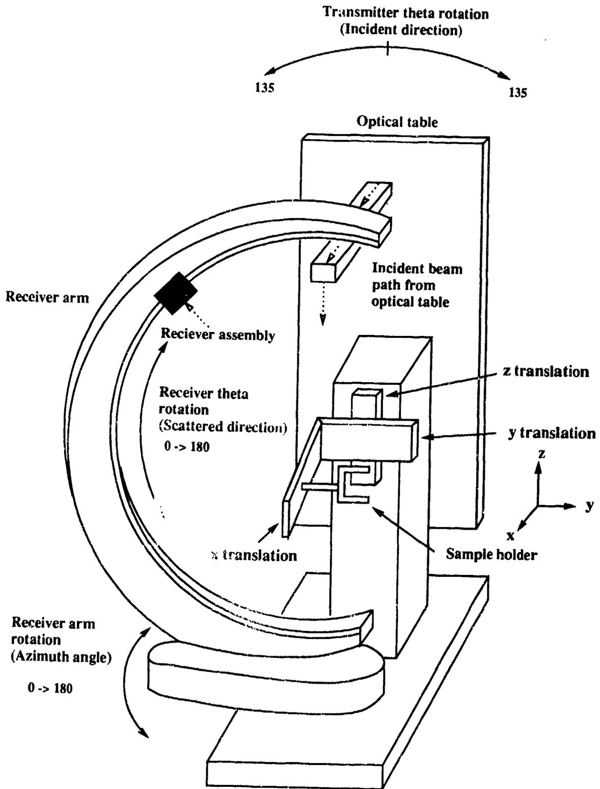
Figure 2. Schematic of the Optical Polarimetric Scatterometer.
