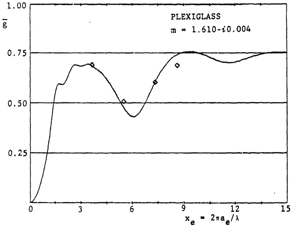
Figure 2 Asymmetry Factor  $\bar{g}$  vs Volume-Equivalent Size Parameter  $x_v$
