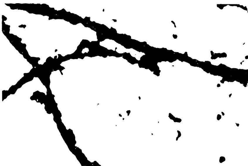
Figure 10. Carbon particles generated for diesel fuel (magnified 35X).
