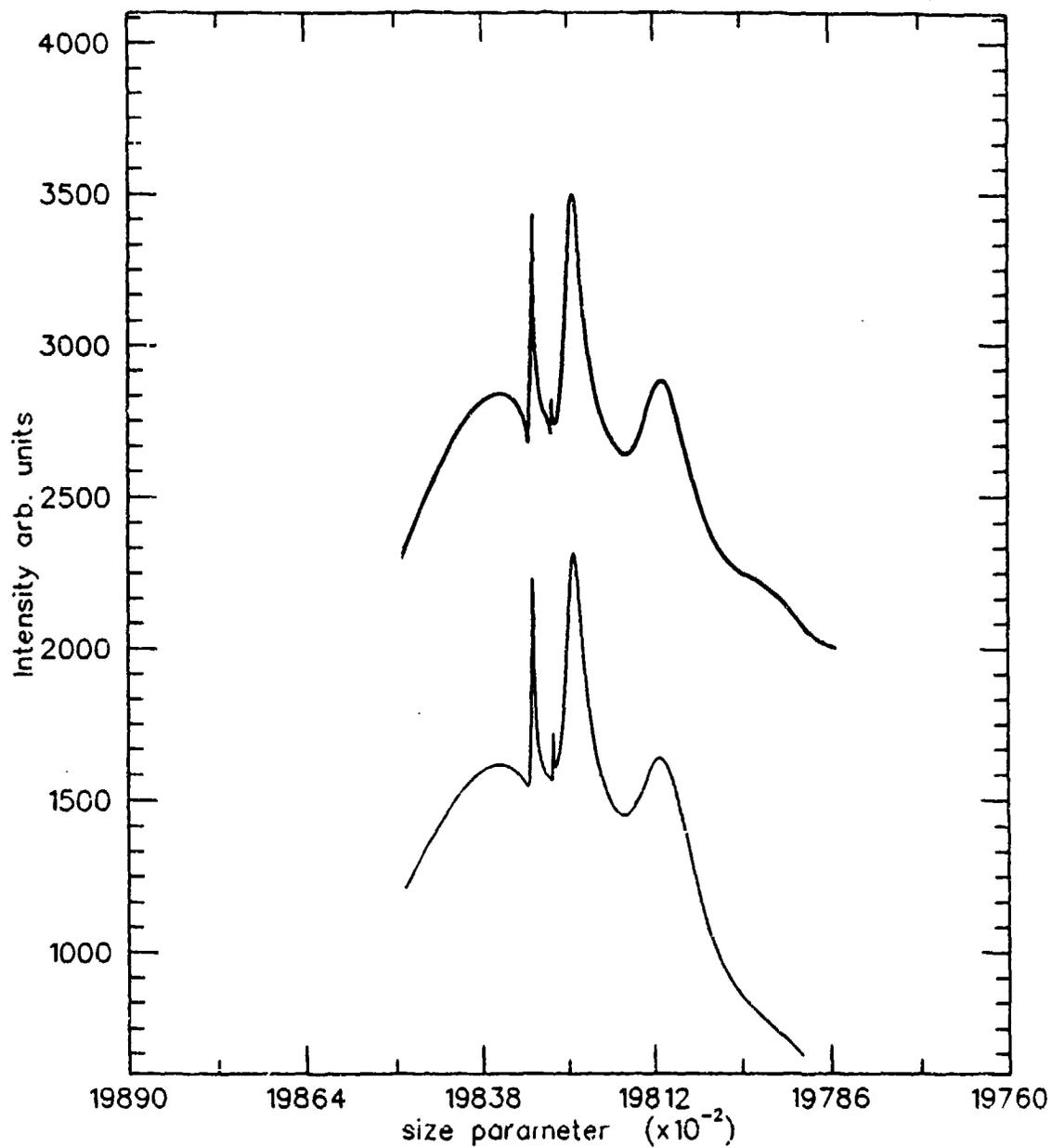
Figure 6. Experimental scattering curve of a glycerin/methanol droplet evaporating from  $r = 15.41$  to  $15.37 \mu\text{m}$  (top) along with the corresponding theoretical curve for  $n = 1.4722$  and  $k = 2.4e-6$  (bottom).
