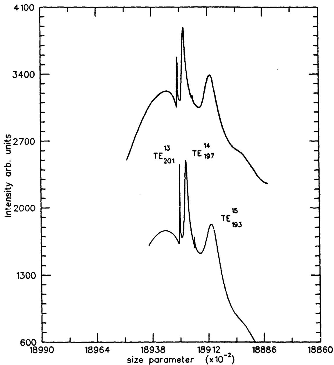
Figure 4 . Experimental scattering curve of a glycerin/methanol droplet evaporating from  $r = 14.71$  to  $14.68 \mu\text{m}$  (top) along with the corresponding theoretical curve for  $n=1.4722$  and  $k=0.0$  (bottom).
