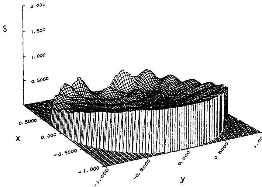
FIGURE 7. Internal normalized source function distribution in the x-y plane for a plane wave incident on a homogeneous circular cylinder. ( $\alpha = 10$ ,  $\bar{n} = 1.18 + 0.07i$ ,  $\theta_{bd} = 0^\circ$ ,  $\phi_{bd} = 90^\circ$ )
