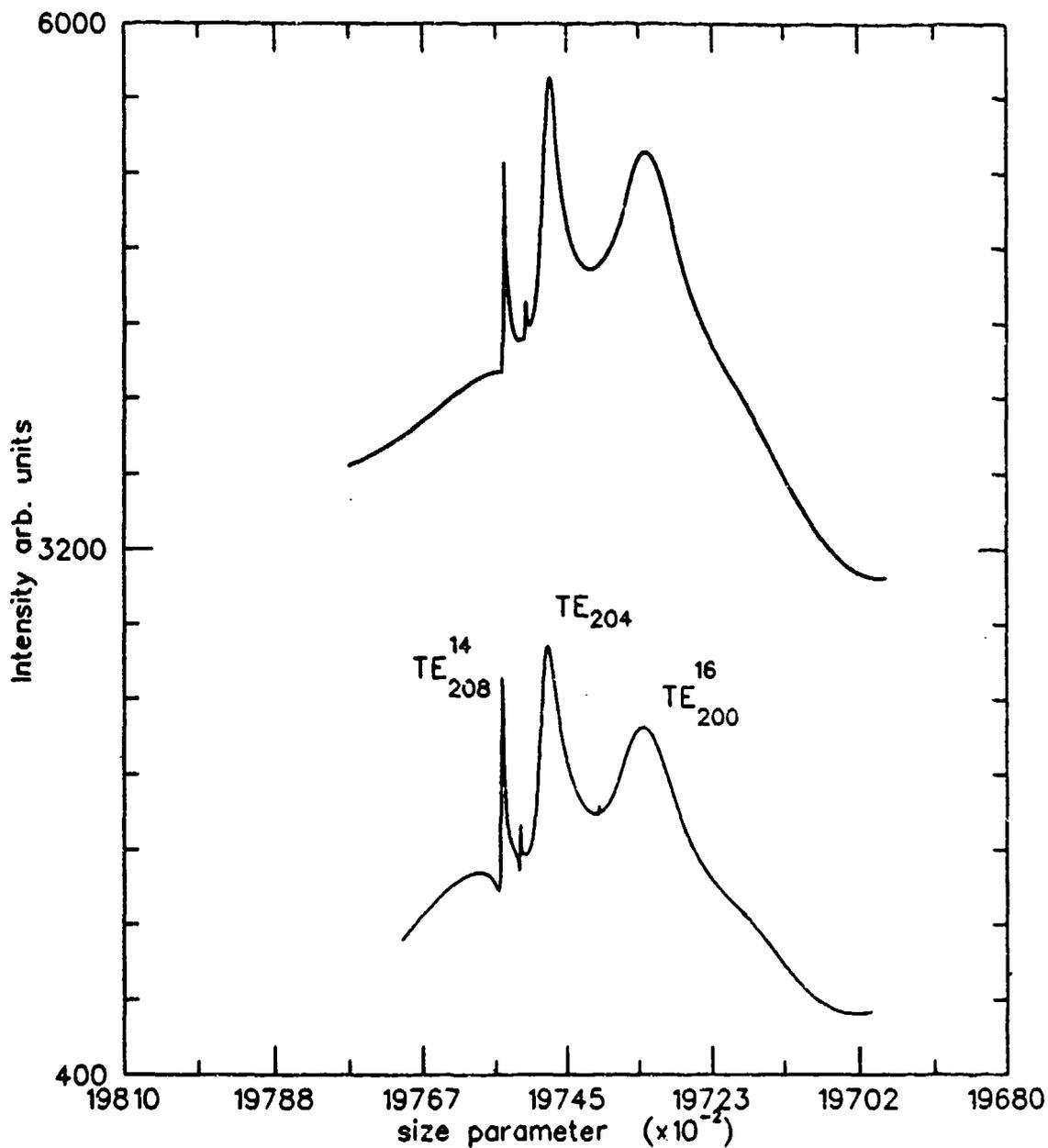
Figure 3. Experimental scattering curve of a glycerin/methanol droplet evaporating from  $r = 15.35$  to  $15.31 \mu\text{m}$  (top) along with the corresponding theoretical curve for  $n=1.4722$  and  $k=0.0$  (bottom).
