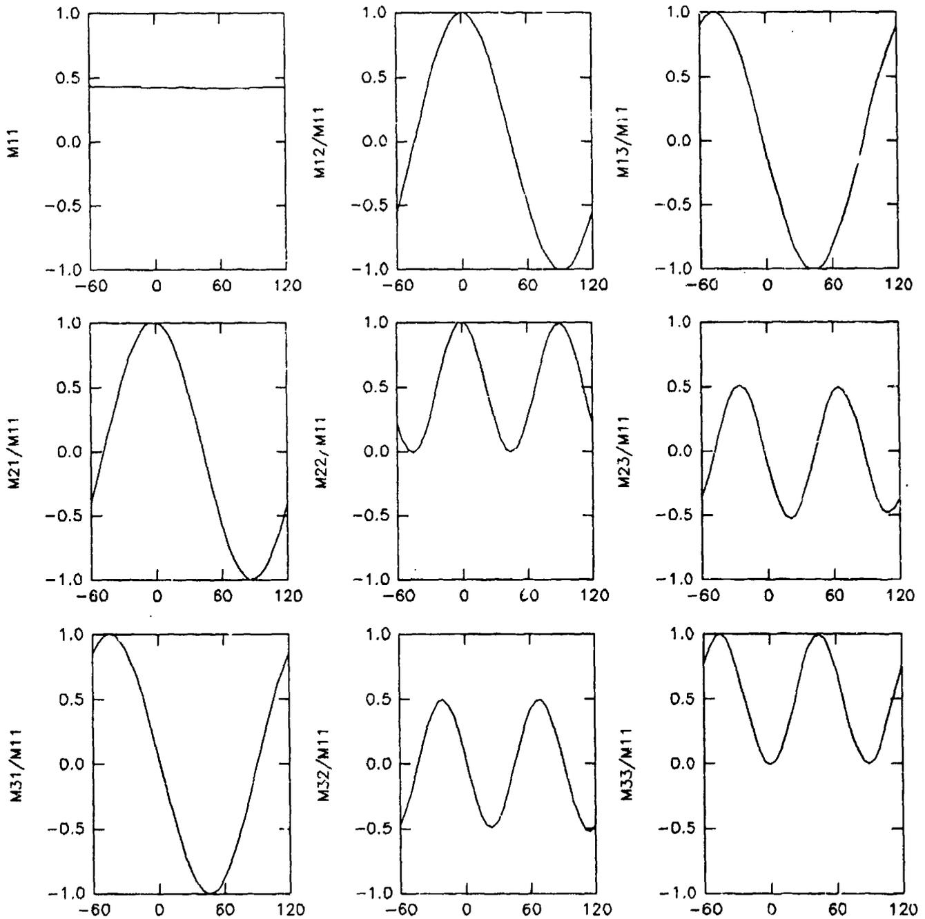
Figure 5a. Muller matrix elements for a polarizer
