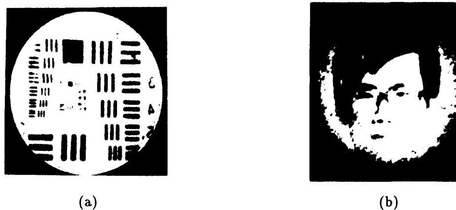
Figure 2: The converted negative coherent images. (a). U.S. Air Force resolution target. (b). A student picture, from a negative.
