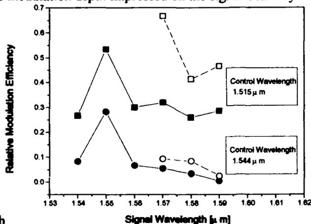
**Fig.3 Modulation of the signal wavelength by the control beam for two different control wavelengths, 1.515 (squares) and 1.544 μm (circles) as a function of the signal wavelength. Open symbols are for TE polarization, solid for TM. Input optical control power, supplied by semiconductor diode lasers, is ≤1 mW.**
