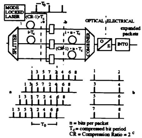
Fig. 3: Packet Decompression (PD) with  $n=8$ ,  $CR=4$ .
