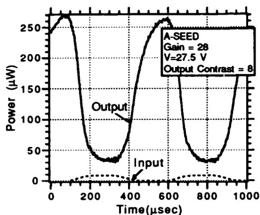
Figure 1.3: Input-Output characteristics of A-SEED device formed with unimplanted and  $1 \times 10^{13} \text{ cm}^{-2}$  implanted AIAs barrier devices.
