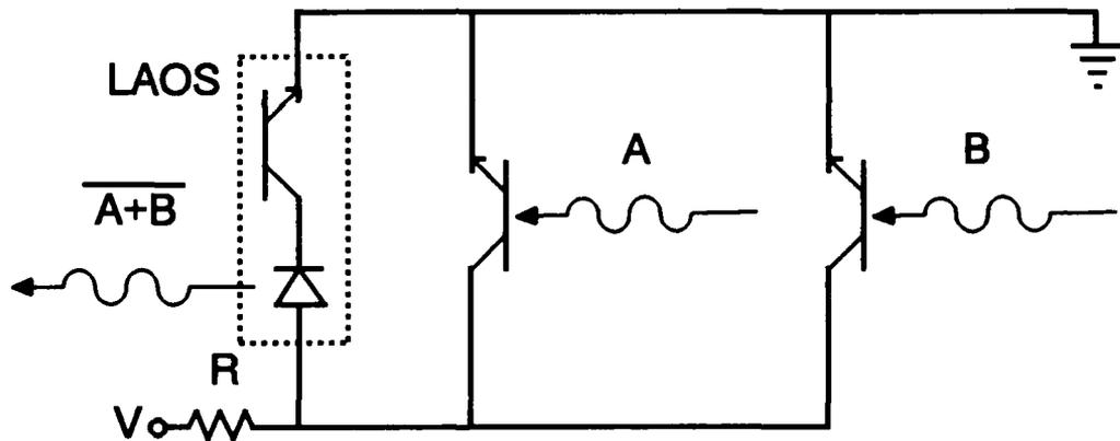
Fig. 2. Equivalent circuit diagram of one pixel of the optical NOR gate array.
