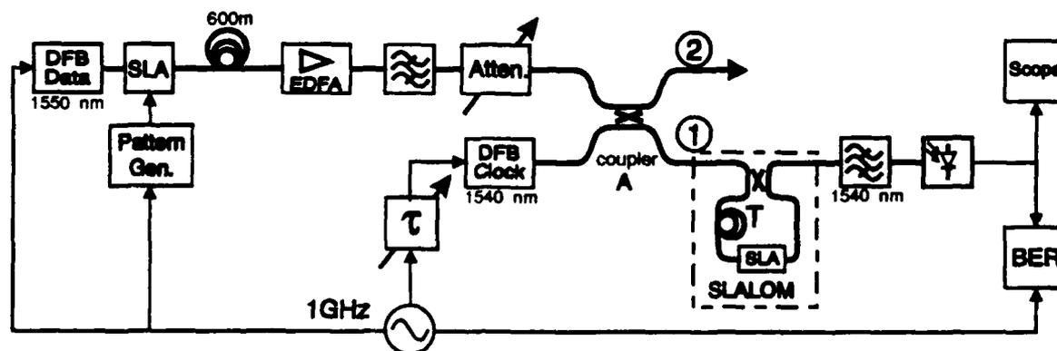
Fig.1: Experimental arrangement
