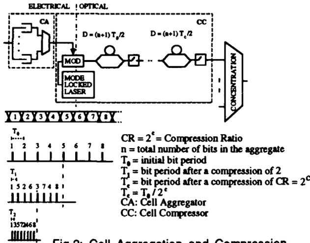
Fig. 2: Cell Aggregation and Compression (CAC) with  $n=8$  bits, and  $CR=4$ .
