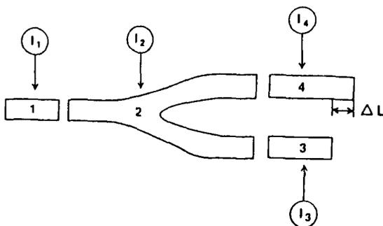
fig. 3: Schematic of an asymmetrical Y-laser
