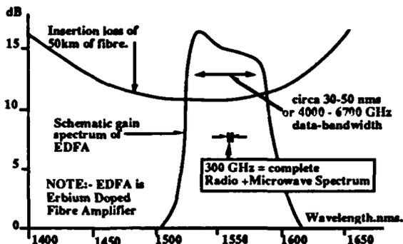
Fig.1 Schematic plot of insertion loss of 50km of fibre with an EDFA gain spectrum overlaid, showing potential transmission window.
