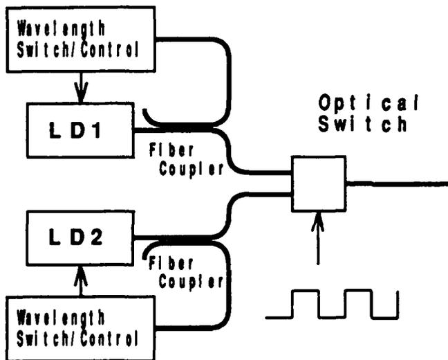
Fig. 2 Configuration for wavelength switched optical transmitter using optical switch.
