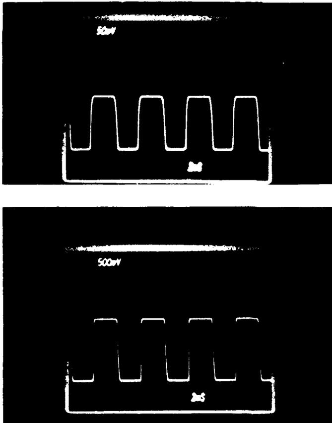
**Fig.2** Oscilloscope traces of (top) optical input control power measured on a photodiode and (bottom) electrical output voltage from the transimpedance amplifier  $V_O$ . Control wavelength is 1.544 μm and incident control power is 1.1 mW. Collector supply voltage  $V_{CC}$  and reverse bias on detector waveguide  $V_D$  are 4V.
