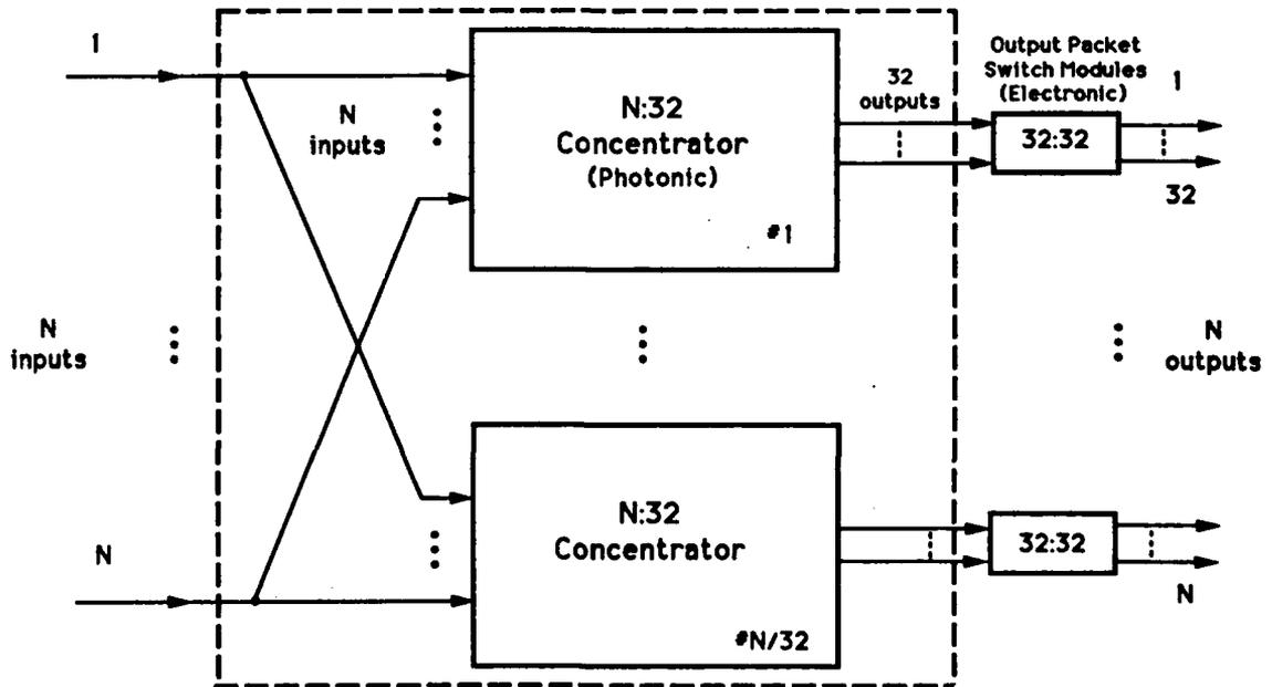
Figure 3: Growable Packet Switch Architecture; Concentrator approach.
