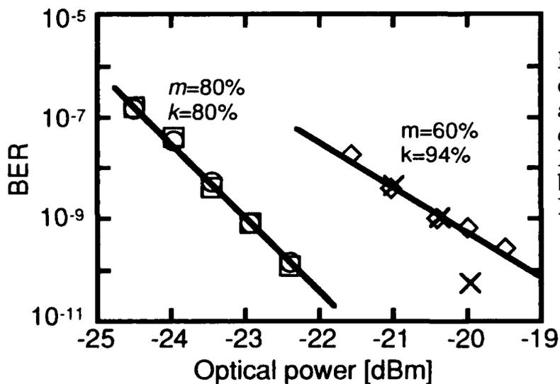
Figure 5 - BER vs. total received optical power (header+payload) at the input to the node for two different sets of values for  $m, k$ . Payload at 2.56 Gb/s represented by □ and ◇. Header at 40 Mb/s represented by ○, and ×.
