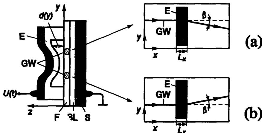
Fig. 4. Deflection of a guided wave by an effective-refractive-index-shifting element E in the form of a bridge with a spatially varying gap width  $d = d(y)$ . Left, cross-sectional view through waveguide and element E. GW, guided wave under element E at positions (a) and (b). F, planar waveguide; S, substrate with buffer layer BL.  $U(t)$ , voltage between the upper part (Si) of element E and waveguide substrate (Si) causing bending of the bridge by electrostatic forces.
