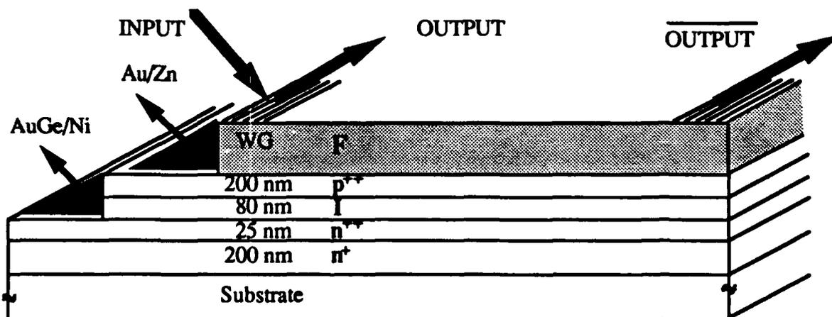
figure 1. Epitaxial layer structure for the grating-waveguide modulator where F is the waveguide film; p, I and n++/n+ form the electronic part of the modulator. The specific materials are indicated in tabel 1.
