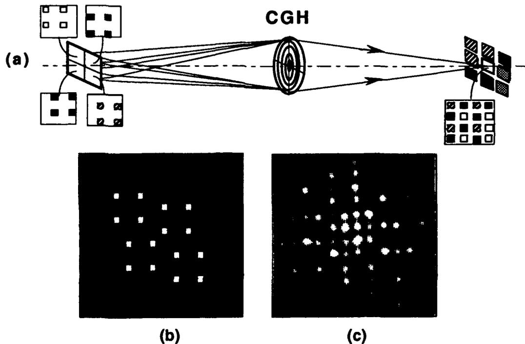
Figure 1. Folded perfect shuffle interconnection using a multiple-imaging CGH. (a); schematic diagram, (b); input with 4x4 pixel array ( $50\mu\text{m}^2$  pixels), (c); experimental result of the perfect shuffled output shown at the center region of 4x4 pixel array.
