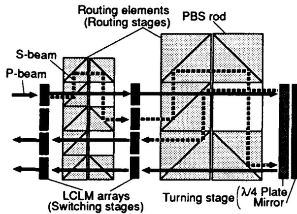
Fig.2 Optical implementation of the turnover-type switching network.
