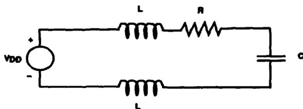
Figure 2: Equivalent circuit for power supply net.
