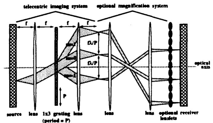
Fig. 2. Optical components used for interconnection.
