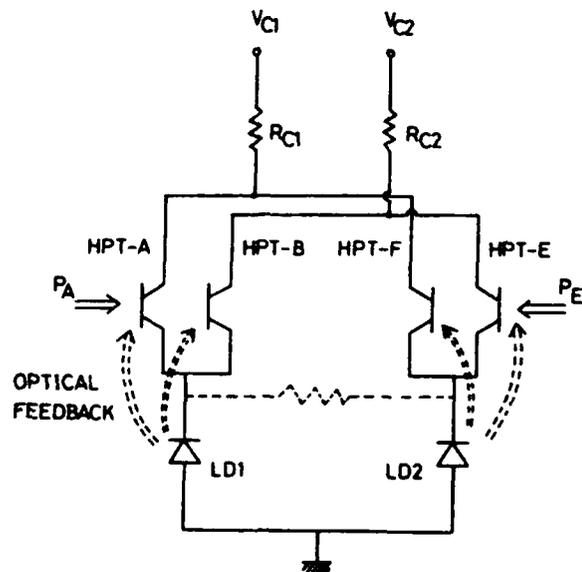
**Fig.6** Equivalent circuit for tristable set-reset flip-flop function.
