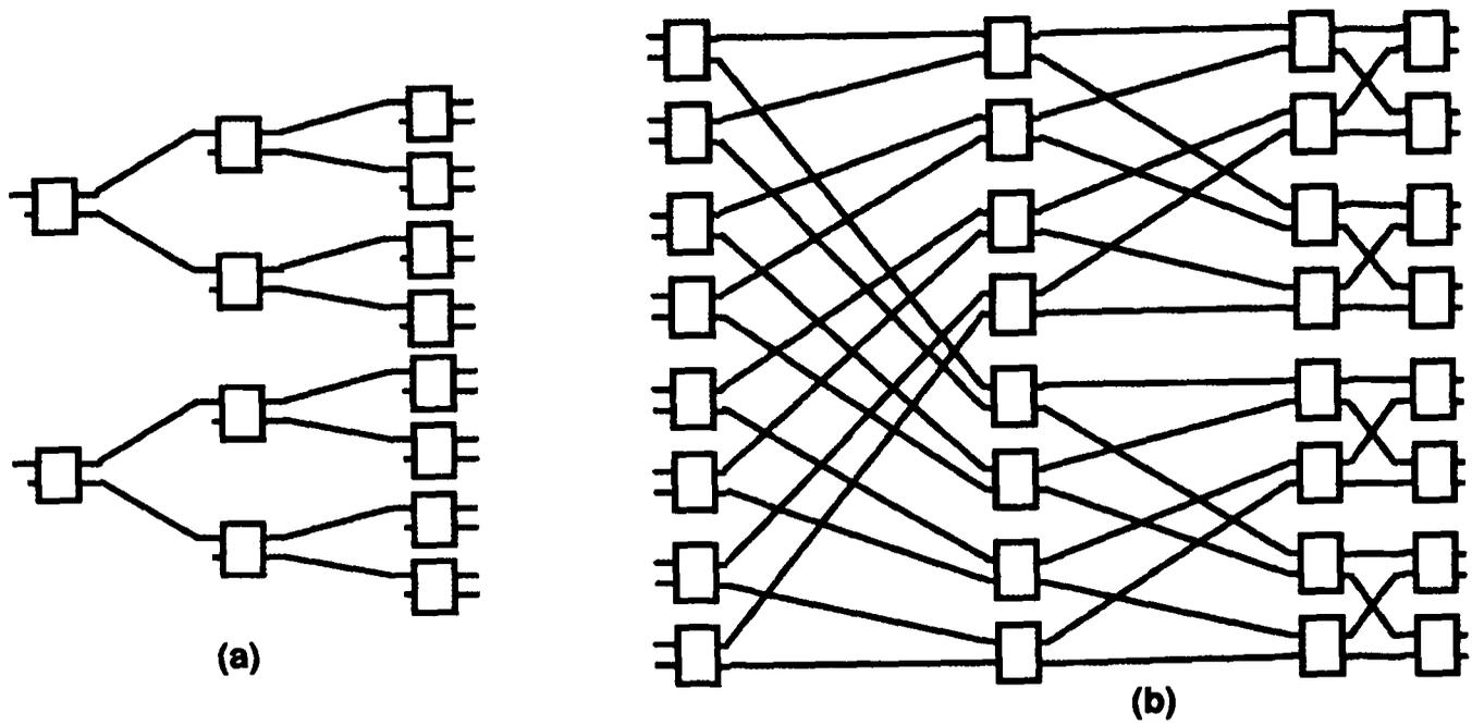
Figure 1. Dual 1x8 (a) and Center Stage (b)
