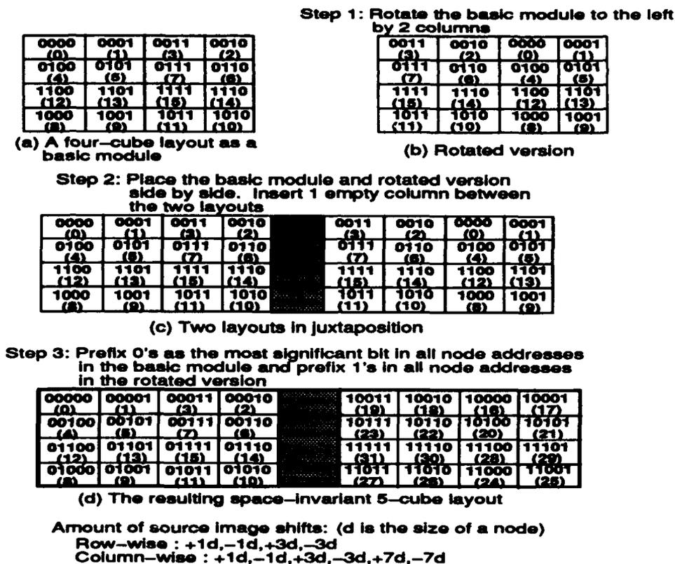
Figure 3: Construction of a 2-D space-invariant 5-cube from two 4-cubes.
