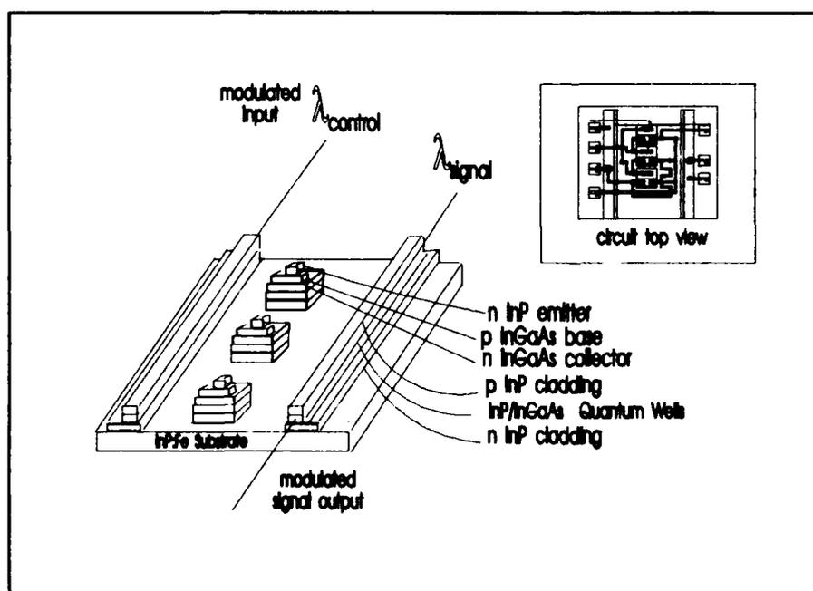
**Fig.1 Schematic of monolithically integrated quantum well p-i-n waveguide photodetector, heterojunction bipolar transistor transimpedance amplifier, and quantum well p-i-n waveguide modulator. Current generated by the control beam in the first waveguide stage is transformed by the electronic circuit to a voltage which drives the second waveguide stage. Modulation at wavelength  $\lambda_{\text{control}}$  is thus converted to wavelength  $\lambda_{\text{signal}}$ .**
