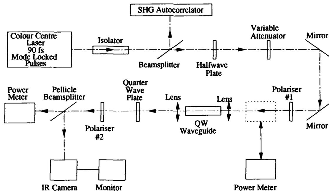
Figure 2 : Experimental Apparatus
