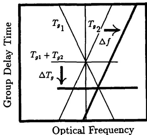
Figure 3: Operation of variable optical delay line
