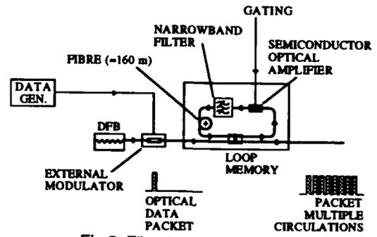
Fig. 5: Fibre loop memory set-up.
