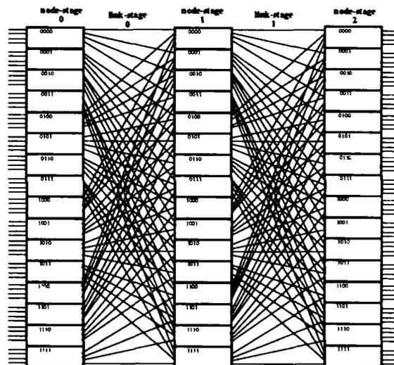
Fig. 6. 4-shuffle network with N=64 inputs.
