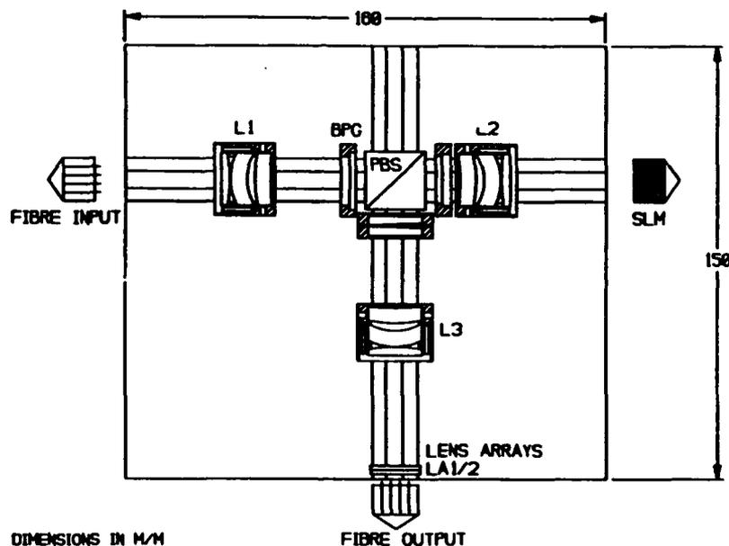
Figure 2: Layout of the 16×16 optical crossbar system
