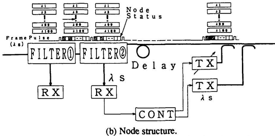
Fig. 1 Wavelength addressed optical network using slotted ring.
