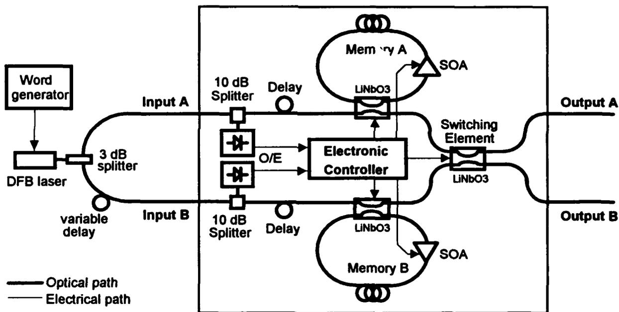
Figure 1: Architecture of the experimental 2x2 packet switch.
