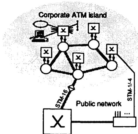
Fig.3. Optical ATM corporate transport network.
