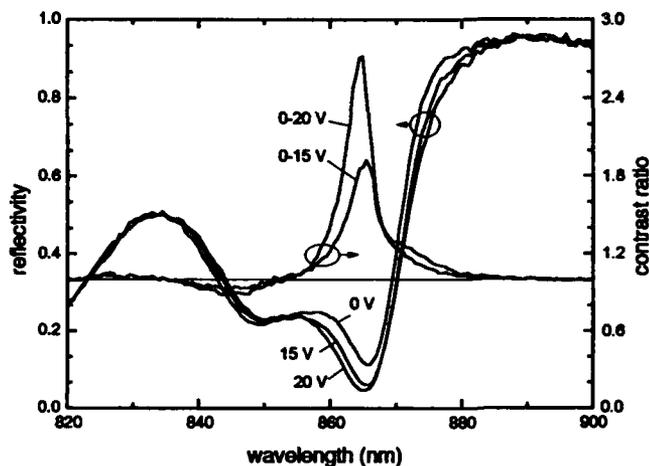
Fig. 2: Reflectivity of our modulator at different biases. Unfortunately the mirror was misaligned with the exciton, reducing performance.
