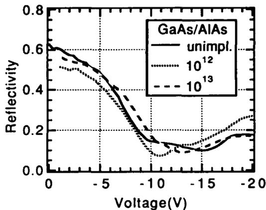
Figure 1.2: Reflectivity vs. voltage for AlAs barrier devices implanted to levels of 0,  $1 \times 10^{12} \text{ cm}^{-2}$ , and  $1 \times 10^{13} \text{ cm}^{-2}$  near 856 nm.
