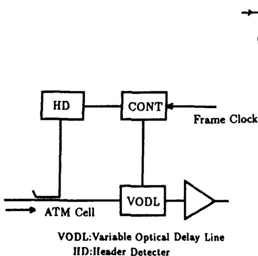
Figure 1: Frame synchronizer
