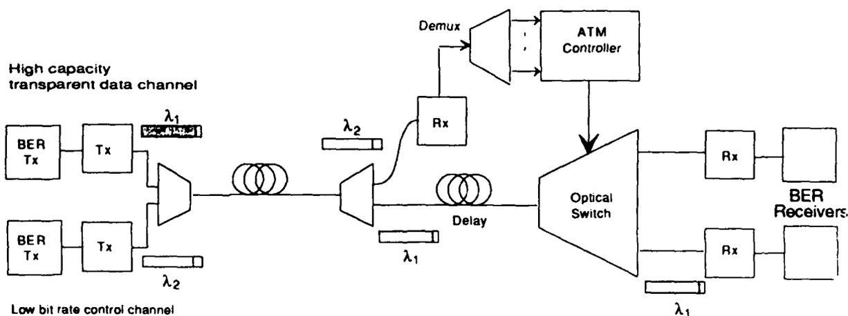
Figure 1: Experimental layout for packet switching
