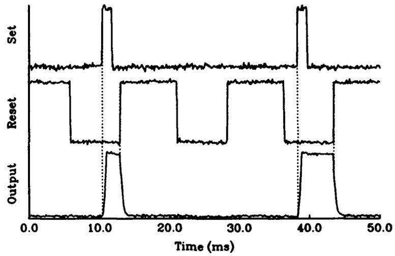
Fig. 2 Experimental demonstration of a single-mesa optical set-reset memory with oscilloscope waveforms proportional to the input and output light signals.
