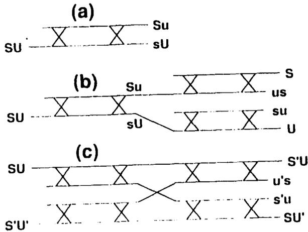
**Fig. 3.** AO switch paths for selected S and unselected U wavelengths for (a) a single-stage 2x2 switch, (b) a dilated 1x2 switch and (c) a dilated 2x2 switch.
