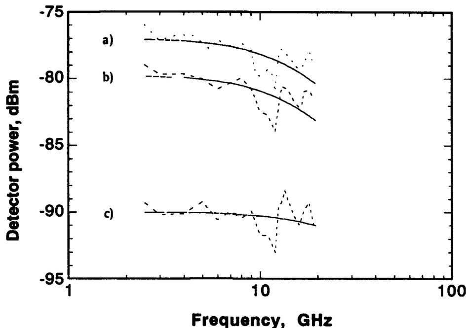
Fig. 6. Swept-frequency modulation measurements at three optical power levels: a) 550  $\mu\text{W}$ , b) 400  $\mu\text{W}$ , c) 80  $\mu\text{W}$ . Solid lines are theoretical curve fits corresponding to  $f_{3\text{dB}} = 18$  GHz, 18 GHz, and 37 GHz, respectively.
