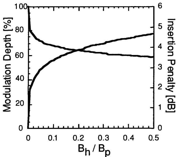
Figure 4 - Optimum modulation depth ( $m$ ) and insertion loss as a function of header/payload bandwidth (or data rate).
