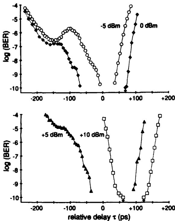
**Fig. 4:** Measured BER versus the relative delay  $\tau$  between data pulse and clock pulse for the data pulse peak powers -5 dBm, 0 dBm, +5 dBm, +10 dBm
