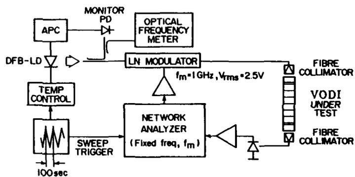
Figure 7: Optical network analyzer
