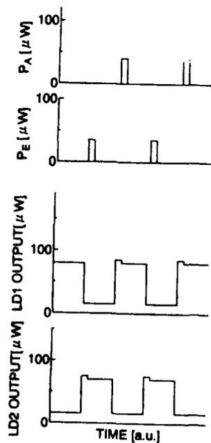
**Fig.5** Bistable set-reset flip-flop operation.
