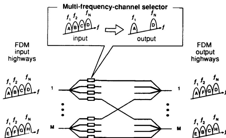
Fig. 1 Photonic FDM highway switch
