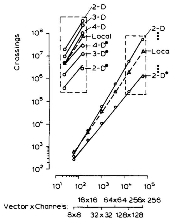
Fig. 10. Total number of crossings (pattern generation + frequency switching) for the nonblocking interconnection by shuffles (upper line), FBS (lower line and indicated by  $\star$ ) and local interconnects (dashed line).
