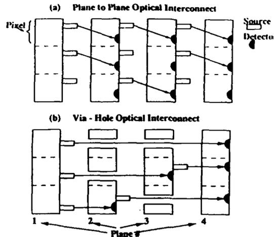
**Fig. 1.** Optical interconnections between several planes. (a) Plane-to-plane communication in which a given plane must relay data by receiving and then retransmitting it. (b) Via-hole windows which establish a permanent optical path.
