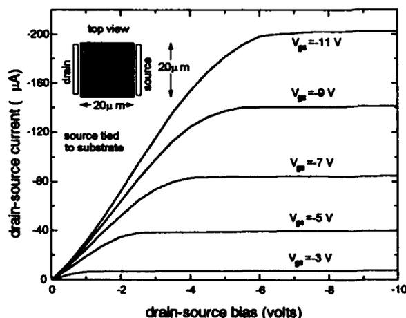
Fig. 3: Common-source characteristics of our PMOS silicon transistor.
