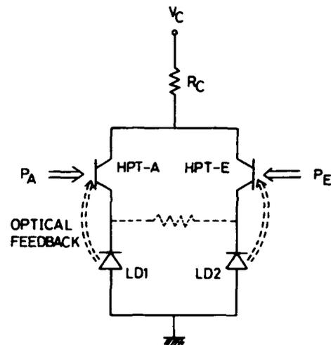
**Fig.4** Equivalent circuit for bistable set-reset flip-flop function.
