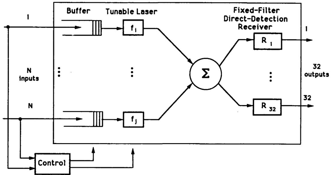
Figure 4: Tunable-transmitter WDM star-coupler based photonic concentrator.
