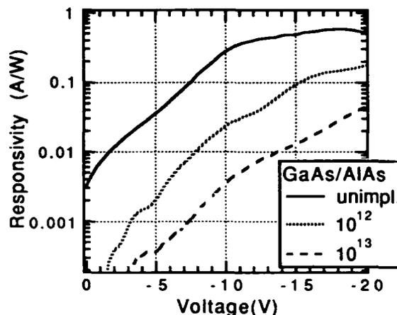
Figure 1.1: Responsivity vs. voltage for AlAs barrier devices implanted to levels of  $0, 1 \times 10^{12} \text{ cm}^{-2},$  and  $1 \times 10^{13} \text{ cm}^{-2}$  for wavelength near 856 nm.
