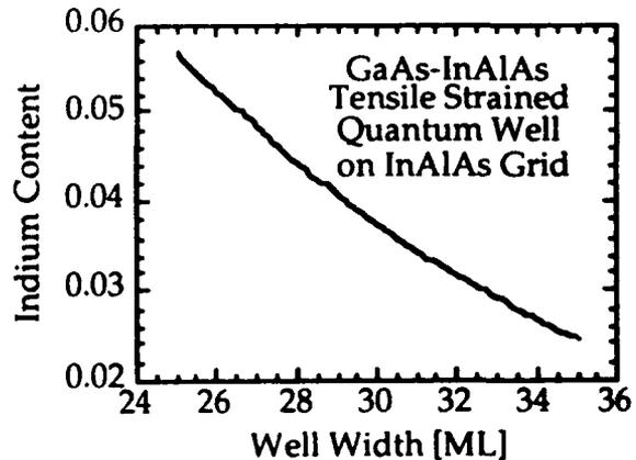
Figure 3 Variation of indium content in grid and barrier layer of tensile-strained GaAs-InAlAs quantum wells with well width for merging of zero-field heavy and light hole energy levels.
