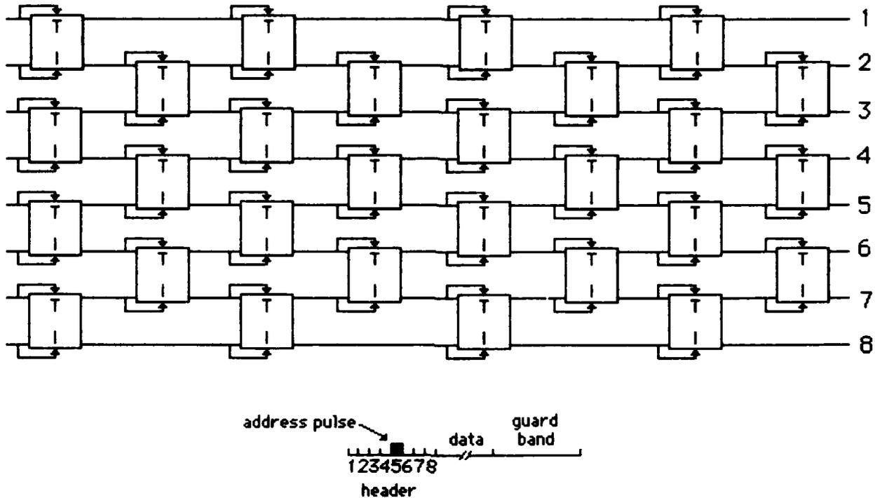
A 2D  $N \times N$  lattice switch, derived by folding a 1D lattice accordion-style, while preserving the interconnection pattern.  $N$  stages are required, which can also be implemented with feedback after the 2nd stage. Each  $2 \times 2$  switching element has inputs on the front, outputs on the back, and connections straight ahead. The self-routing rule is the same as above.
