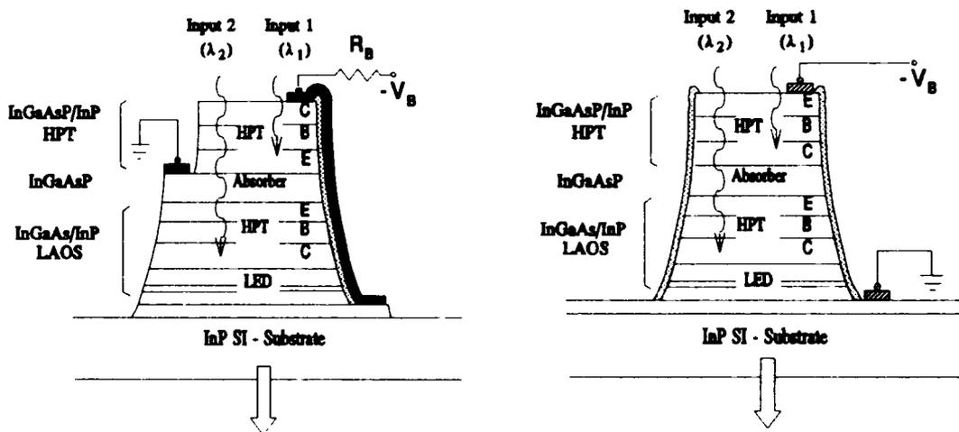
**Fig. 1 Schematic device structure of single-mesa pixels : (a) with the top HPT collector up and interconnected in parallel with an optical switch (the lower HPT/LED pair, the LAOS); (b) with the top HPT emitter up and connected in series with the switch.**
