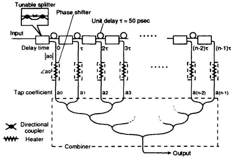
Fig. 2 Coherent optical transversal filter
