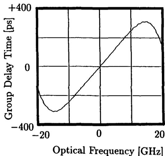
Figure 4: Characteristics of dispersive optical circuit
