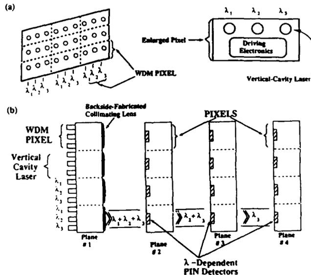
**Fig. 2.** (a) A multiple- $\lambda$  VCSEL array in which (M-1) different- $\lambda$  lasers are fabricated in each identical WDM pixel. (b) One-to-many optical plane interconnection configuration using a 3- $\lambda$  VCSEL pixel array and three  $\lambda$ -selective detecting planes.
