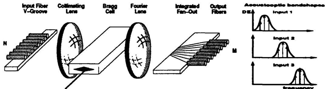
Figure 1: Optical layout of switch and AO bandshapes for each input
