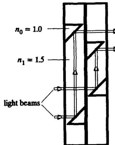
Fig. 6 A multilayer construction of the optic-slabs
