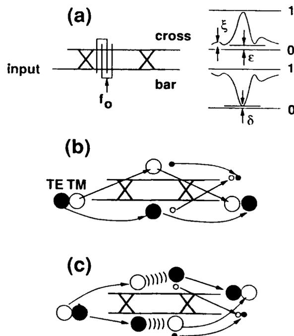
**Fig. 2.** (a) Bar (band-reject) and cross (bandpass) state spectral transmissions for a single acoustic grating; TE (open circle) and TM (closed circle) mode paths and leakage paths for (b) beamsplitter leakage and (c) incomplete polarization conversion.
