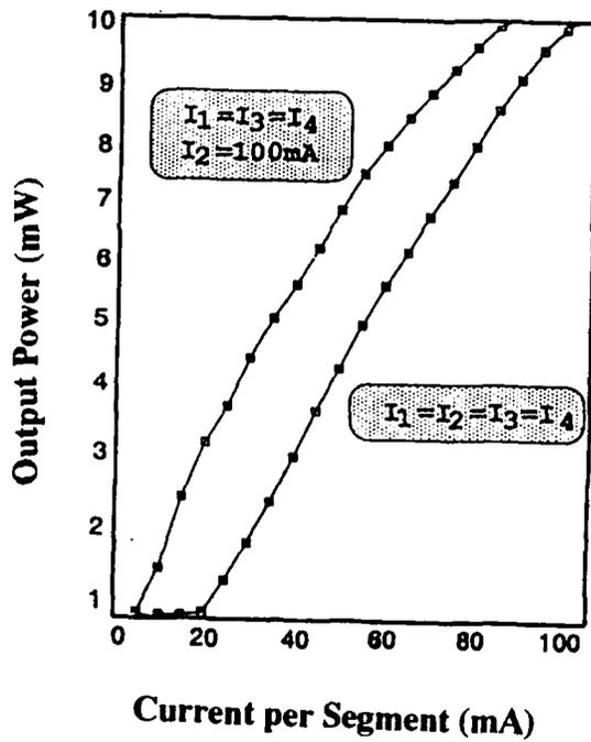
fig. 2: Y-laser light/current characteristics
