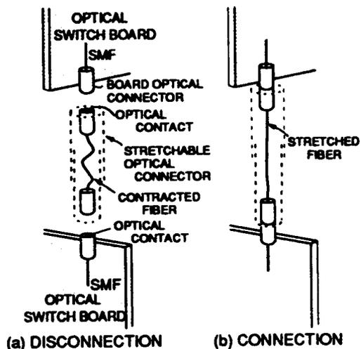
Fig.4 BOARD-TO-BOARD OPTICAL CONNECTOR
