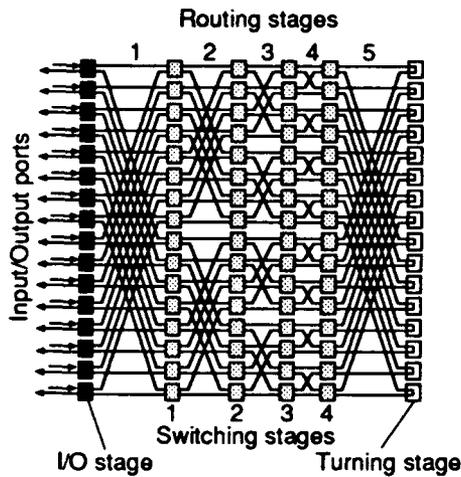
Fig.1 Network configuration of 16x16 turnover-type Benes network.
