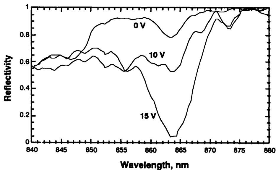
Fig. 3. DC spectra of finished  $16\ \mu\text{m} \times 20\ \mu\text{m}$  device
