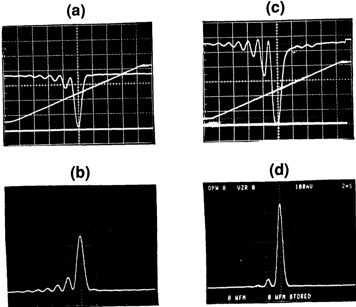
**Fig. 5.** Left: one-stage transmissions for 1559 nm source and 3 MHz RF sweep, equivalent to a 27 nm wavelength scan. (a) bar state and (b) cross state. Right: dilated switch in the (c) cross state and (d) bar state.
