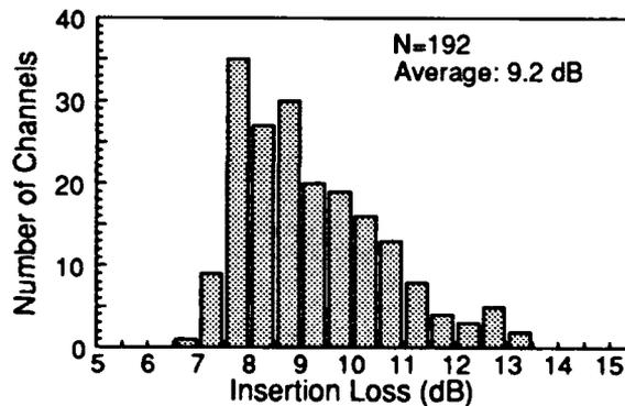
Fig.6 Optical insertion loss histogram for the fabricated 64x64 optical switch.
