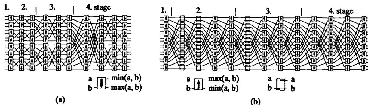
Fig.1 Bitonic sorting network proposed by
