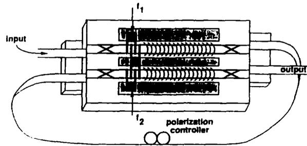
**Fig. 4.** Schematic of the experimental pair of devices and their connection to form a dilated 1x2 cross state demonstration.
