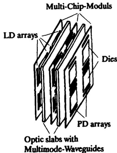
Fig. 5 Design concept of a 3-D optoelectronic MIN
