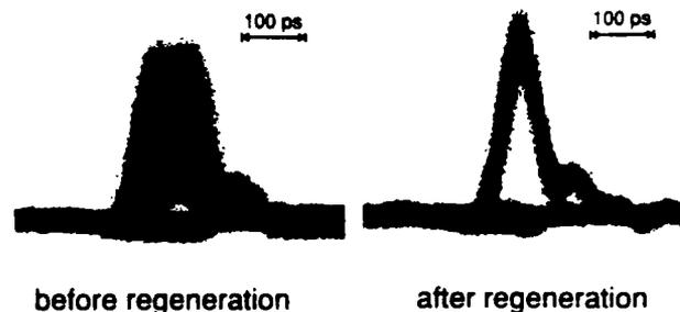
**Fig. 3:** Eye diagrams of the data signal before and after regeneration
