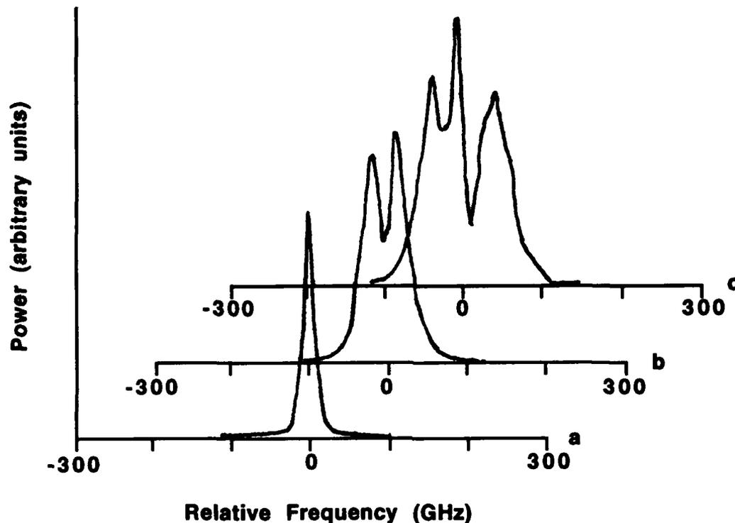
Fig. 1: Spectra of 21ps pulses after passing through active ridge waveguides in TE polarisation.
