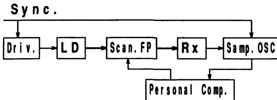
Fig. 5 Optical frequency transient response measurement system.
