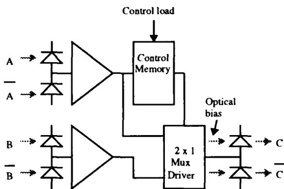
Fig. 1. Embedded control 2 x 1 node
