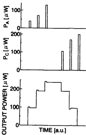
**Fig.3** Latch and erase functions in tetrastable states.
