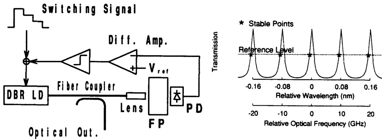
(a) Block diagram for the proposed control scheme.
