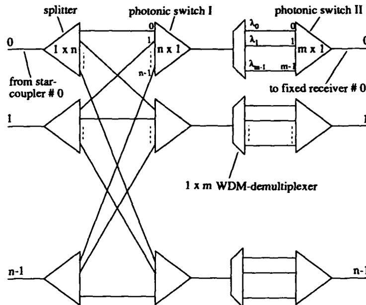
Figure 2: Wavelength Selective Switch (WSS) composed of splitters, WDM-demultiplexers and photonic switches.
