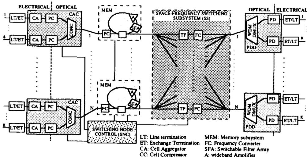
Fig.1: ATM DXC global architecture.
