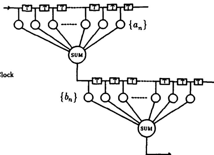
Figure 2: Basic structure of variable optical delay line
