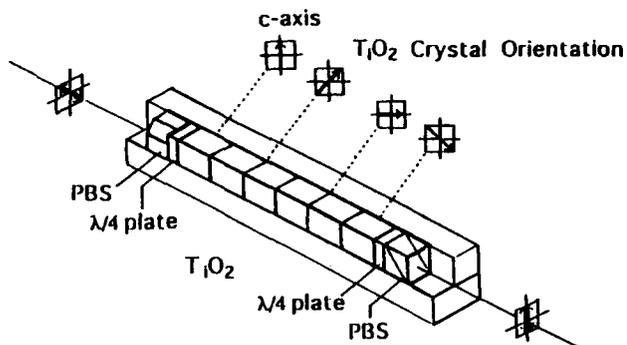
Figure 6: Basic structure of Chebyshev polynomials filter
