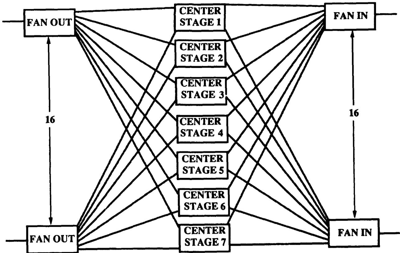
Figure 2. 16x16 Strictly Non-Blocking Extended Generalized Shuffle Network
