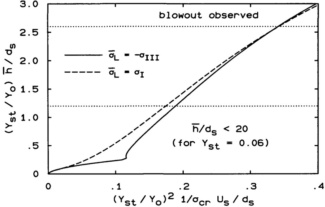
FIG. 3.1 Non-dimensional liftoff height *vs.* velocity as predicted by the strain-rate model, when  $\sigma_L$  is approximated by the largest principal compressive ( $-\bar{\sigma}_{III}$ ) or extensive ( $\bar{\sigma}_I$ ) strain rate of the mean flow field.
