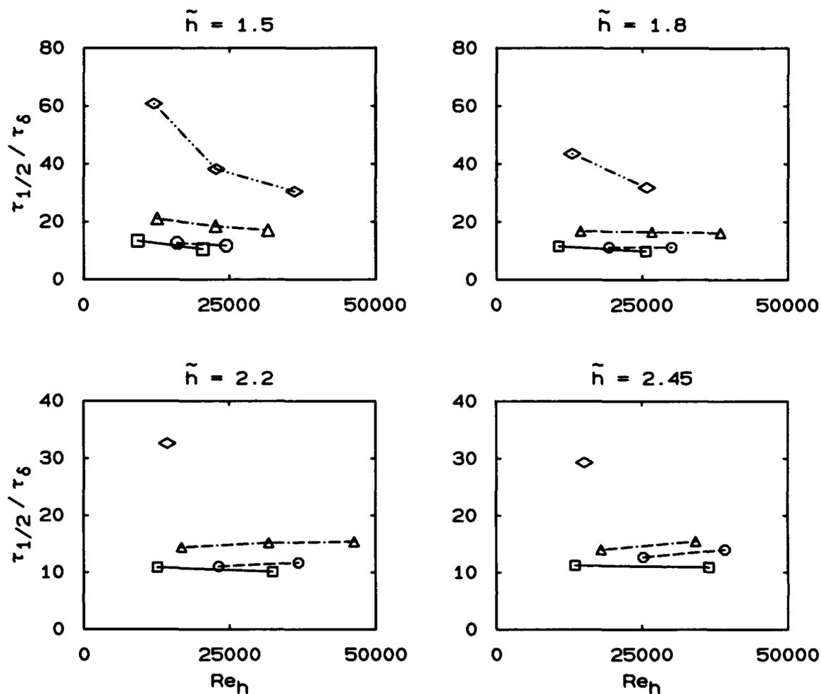
FIG. 4.9 Variation of  $\tau_{1/2}/\tau_\delta$  with  $Re_h$  and fuel type at four values of  $\tilde{h} = 1.5, 1.8, 2.2,$  and  $2.45$ . See Fig. 4.8 for definitions of symbols. Note the different vertical axes of the top and bottom plots.
