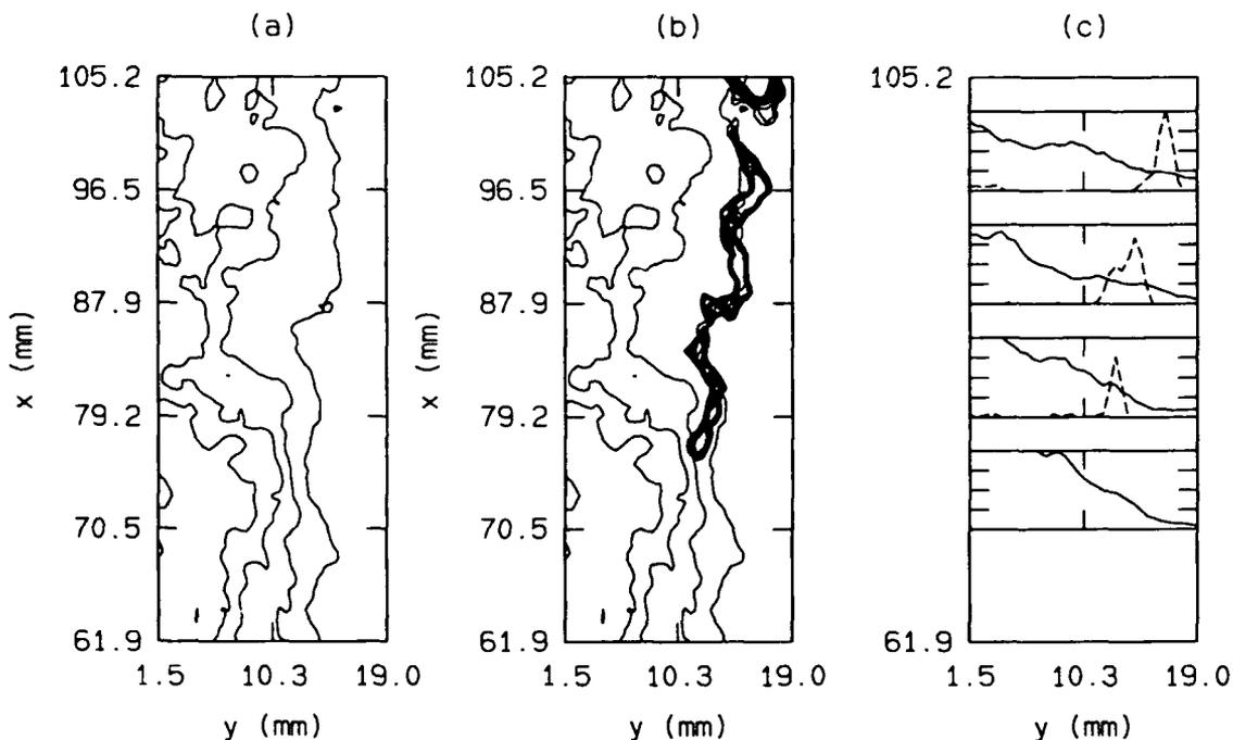
FIG. 5.3 Instantaneous shot illustrating relatively straight reaction zones. (a)  $[\text{CH}_4]$ , (b)  $[\text{CH}_4]$  and  $[\text{CH}]$ , (c) cuts across flame; solid line  $[\text{CH}_4]$ , vertical axis is 0, ..., 0.2; dashed line  $[\text{CH}]$ , vertical axis is 0, ..., 1. For contour levels see caption of Fig. 5.2.
