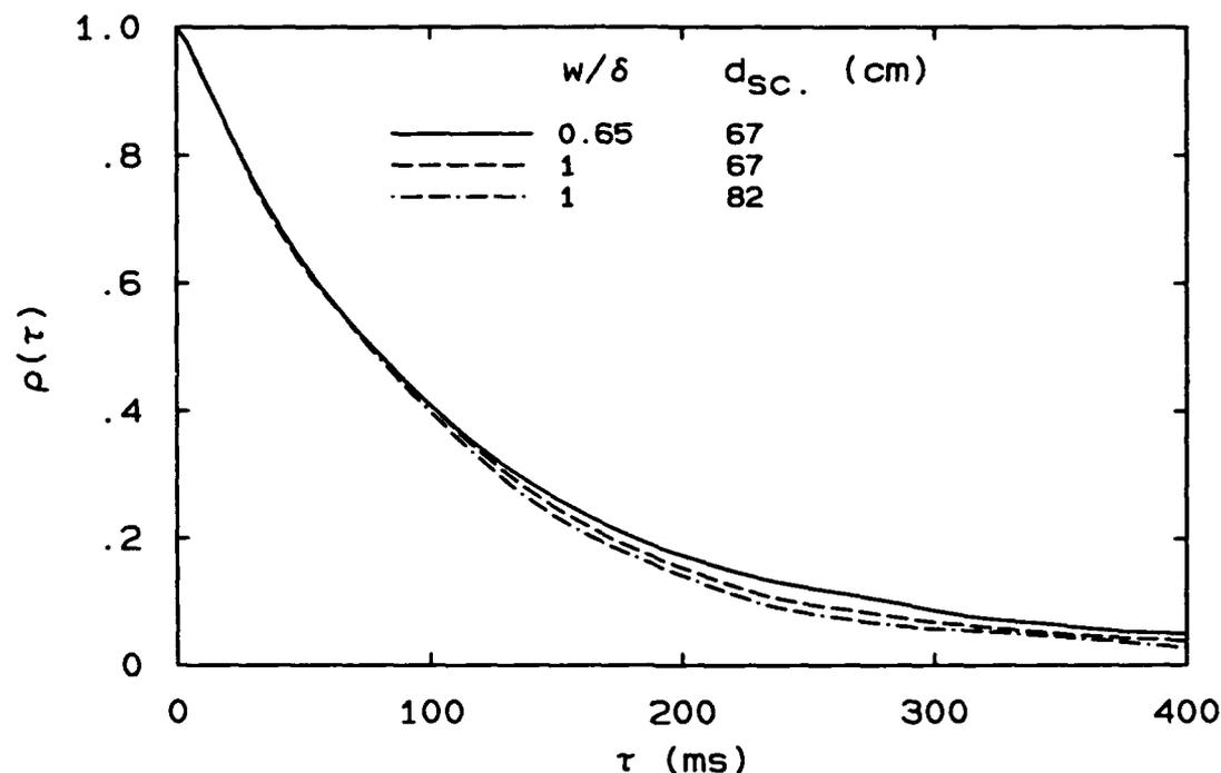
FIG. D.1 Autocorrelation of liftoff height. Natural gas,  $d = 6.25$  mm,  $U_s = 61$  m/s. Solid line: fraction of width imaged  $w/\delta = 0.65$ , dashed line:  $w/\delta = 1$ , dot-dash: same as dashed, except a larger screen diameter was used.
