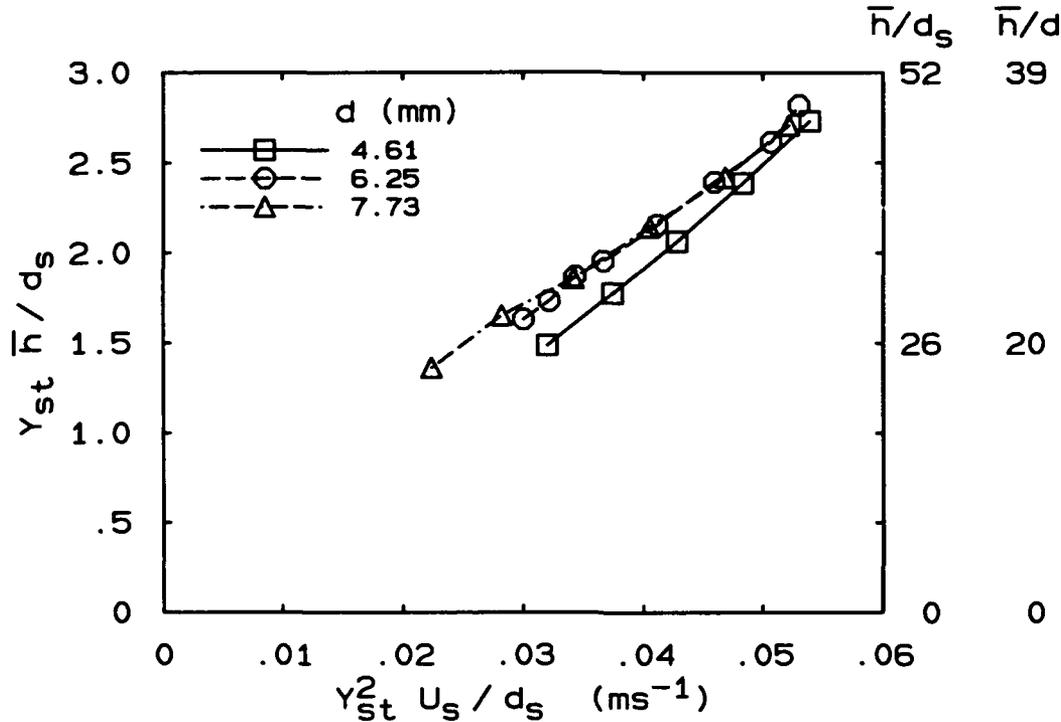
FIG. 3.4 Normalized mean liftoff heights *vs.* normalized velocity for natural gas. Values of  $\bar{h}/d_s$  and  $\bar{h}/d$  are shown along the right side of the graph.
