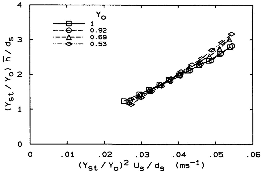
FIG. 3.10 Normalized liftoff height vs. normalized velocity for natural gas, for varying fuel mass fraction  $Y_o$  in the nozzle fluid.
