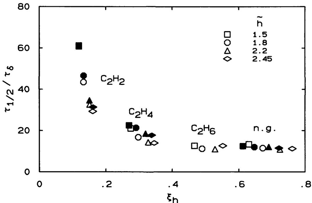
FIG. 4.13 Effect of nozzle orientation on scaled correlation time  $\tau_{1/2}/\tau_{\delta}$  vs. Richardson number  $\xi_h$ . Open symbols: vertical nozzles, filled symbols: horizontal nozzles.
