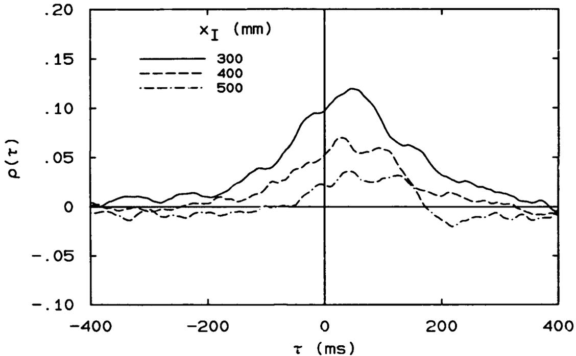
FIG. 4.22 Correlation of  $h$  and light intensity  $I$  vs. time. Natural gas,  $d = 6.25$  mm,  $U_s = 61$  m/s,  $\bar{h} = 181$  mm,  $x_I = 300, 400,$  and  $500$  mm.
