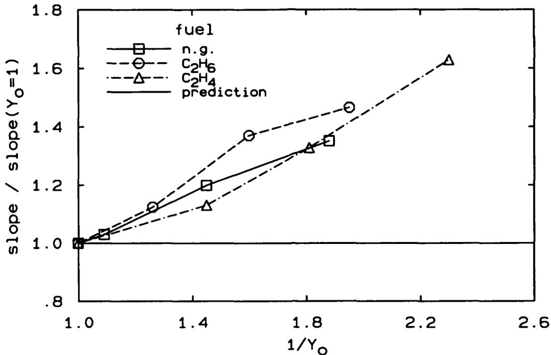
FIG. 3.13 Variation of the slope of the curve of  $(Y_{st}/Y_o)\bar{h}/d_s$  vs.  $(Y_{st}/Y_o)^2 U_s/d_s$  at  $(Y_{st}/Y_o)\bar{h}/d_s = 2.0$  with  $Y_o$ . The slopes have been normalized by the slope for  $Y_o = 1$ .
