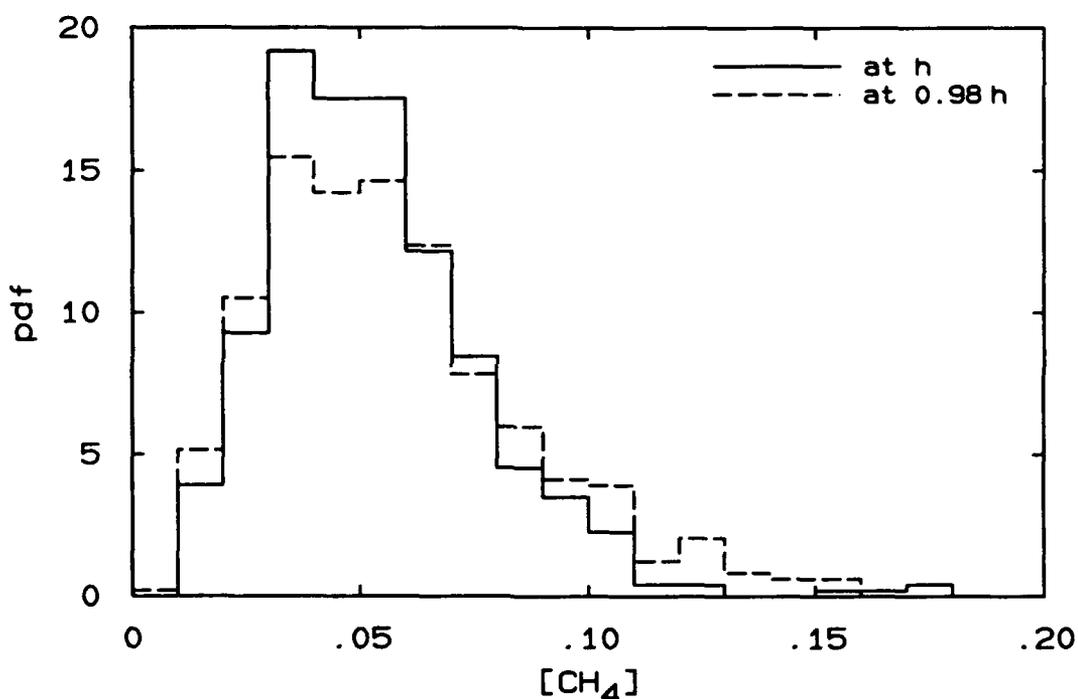
FIG. 5.10 Probability density function of  $[CH_4]$  at the flame base ( $x = h, y = y_h$ ), and at a location just upstream of the flame base ( $x = 0.98 h, y = y_h$ ).
