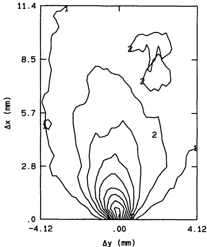
FIG. 5.7 Contours of probability of finding reaction ( $[CH] > 0.3$ ) at locations displaced from the liftoff location by  $\Delta x$  in the vertical direction and  $\Delta y$  in the horizontal direction. Nine contours are shown from 0.9 to 0.1; only the lowest two contour levels are labeled, 1: 0.1, 2: 0.2.
