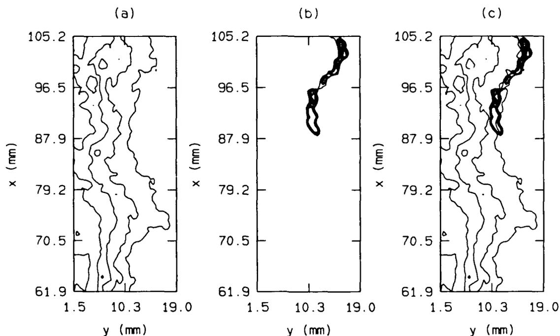
FIG. 5.2 Instantaneous shot illustrating curved reaction zones. Contour plots of (a)  $\text{CH}_4$  number density, (b)  $[\text{CH}]$  signal, and (c) the superposition of (a) and (b). The contour levels for  $[\text{CH}_4]$  are 0.05, 0.1, 0.15, 0.2, and 0.3. The levels for  $[\text{CH}]$  are 0.3, 0.34, 0.38, 0.42, 0.46, 0.50, 0.54, 0.58, 0.62, and 0.66.
