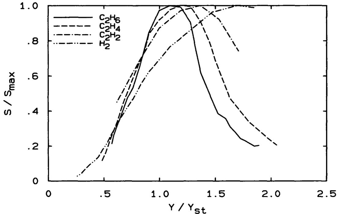
FIG. 4.27 Variation of laminar flame speed with mass fraction. Data for  $C_2H_6$ ,  $C_2H_4$ , and  $C_2H_2$  are from Egolfopoulos, Zhu, and Law (1991);  $H_2$  data are from Egolfopoulos and Law (1991).
