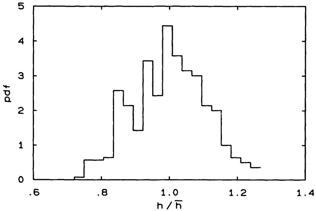
FIG. 5.8 Probability density function of liftoff height.
