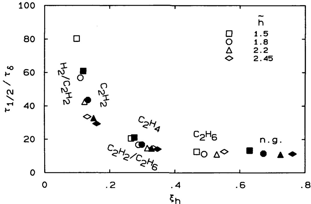
FIG. 4.14 Variation of normalized correlation time  $\tau_{1/2}/\tau_\delta$  with Richardson number  $\xi_h$ , for the conditions listed in Table 4.1 and for the 50% C<sub>2</sub>H<sub>2</sub> / 50% C<sub>2</sub>H<sub>6</sub> and 50% H<sub>2</sub> / 50% C<sub>2</sub>H<sub>2</sub> mixtures listed in Table 4.5. Filled symbols: n.g., C<sub>2</sub>H<sub>4</sub>, and C<sub>2</sub>H<sub>2</sub>.
