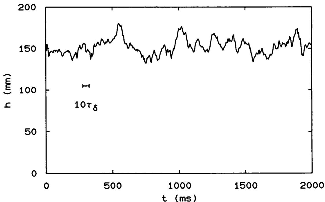
FIG. 4.5 Liftoff height  $h$  vs. time.  $C_2H_6$ ,  $d = 3.88$  mm,  $U_s = 88$  m/s,  $\bar{h} = 151$  mm.
