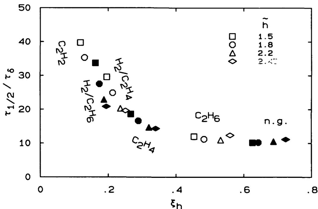
FIG. 4.15 Variation of normalized correlation time  $\tau_{1/2}/\tau_\delta$  with Richardson number  $\xi_h$ , comparing C<sub>2</sub>H<sub>2</sub> flames with mixtures of H<sub>2</sub> with C<sub>2</sub>H<sub>6</sub> and C<sub>2</sub>H<sub>4</sub>.  $Re_h = 22,000$ . Filled symbols: n.g., C<sub>2</sub>H<sub>4</sub>, 86% H<sub>2</sub> / 14% C<sub>2</sub>H<sub>6</sub>.
