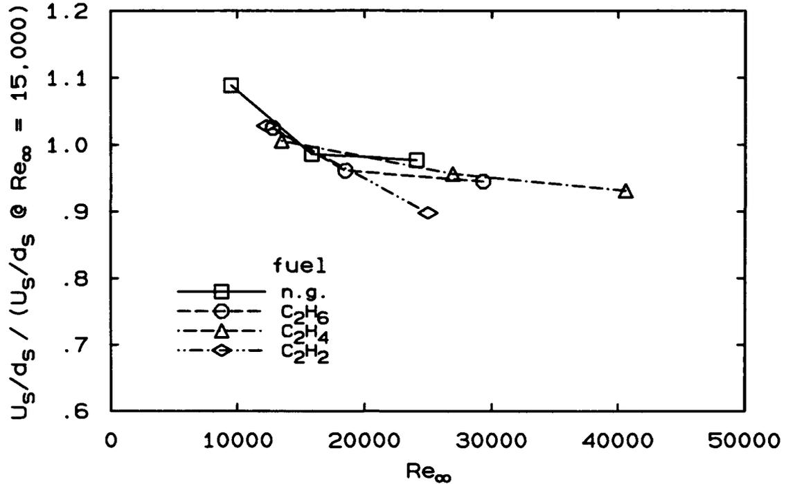
FIG. 3.8 Normalized velocity  $Y_{st}^2 U_s / d_s$  at  $Y_{st} \bar{h} / d_s = 2.0$  vs. Reynolds number  $Re_\infty$ , for all four fuels. The curves have been normalized to pass through the point (15,000, 1) to allow all fuels to be displayed on one plot.
