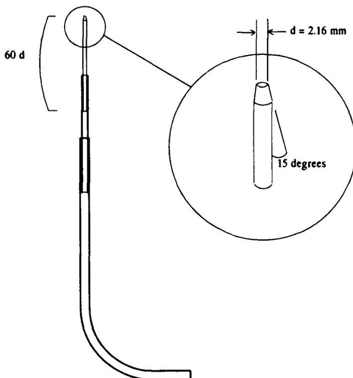
FIG. 2.1 Design of the 2.16 mm nozzle. Brass tubes with outer diameters of 9.5 mm, 6.4 mm, and 3.2 mm are soldered together as shown, reaching a final inner diameter of 2.16 mm.
