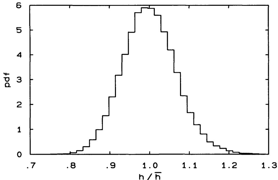
FIG. 4.1 Probability density function (pdf) of liftoff height.  $C_2H_6$ ,  $d_s = 3.88$  mm,  $U_s = 88$  m/s,  $\bar{h} = 151$  mm.
