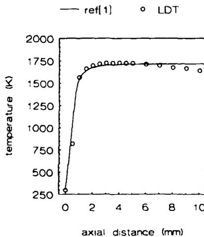
Figure 5: gas temperature as function of  $x$ ;  $r = 0$  mm
