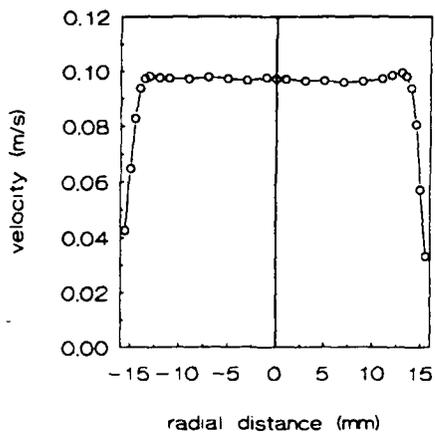
Figure 2: axial unburnt gas velocity as function of  $r$ ;  $x = 3$  mm
