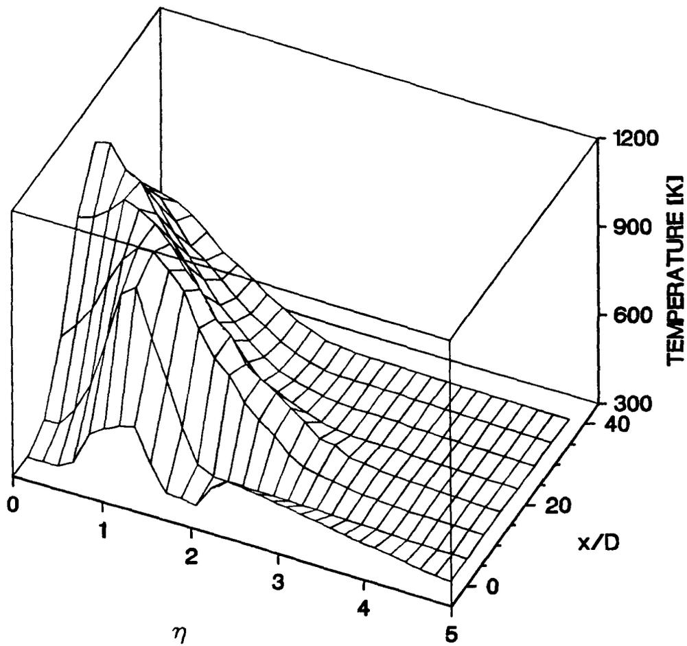
Figure 4: Favre averaged temperatures versus  $\eta$  and versus  $x/D$  in a three dimensional plot.
