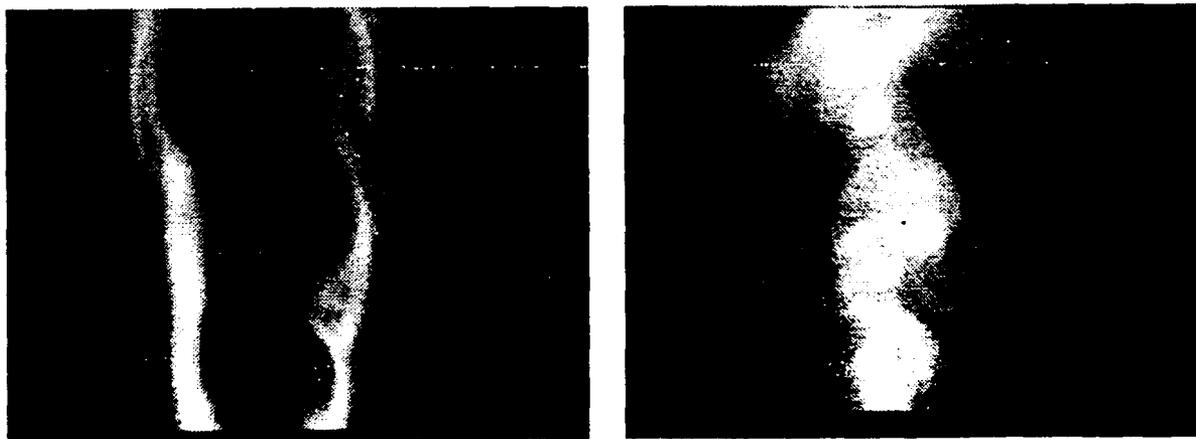
Fig. 1: Simultaneous single-shot two-dimensional fluorescence signal distribution of OH (left) and doped NO (right) in a turbulent H<sub>2</sub>/air diffusion flame
