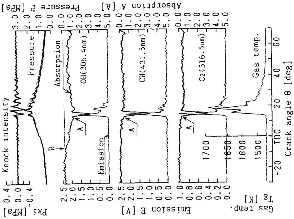
Fig.4 Normal combustion with n-heptane (0 RON)
