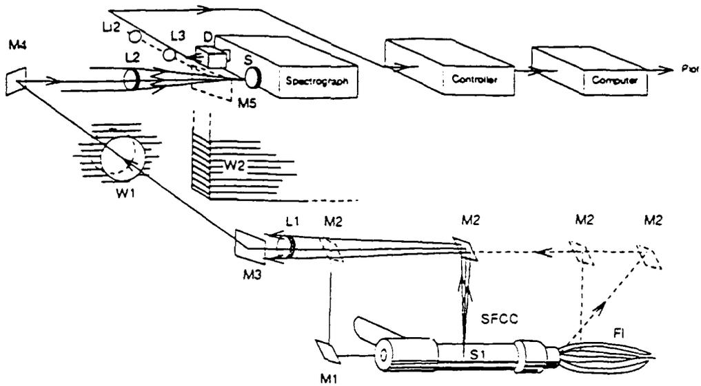
Figure 1 Optical equipment for spectrographic measurements
