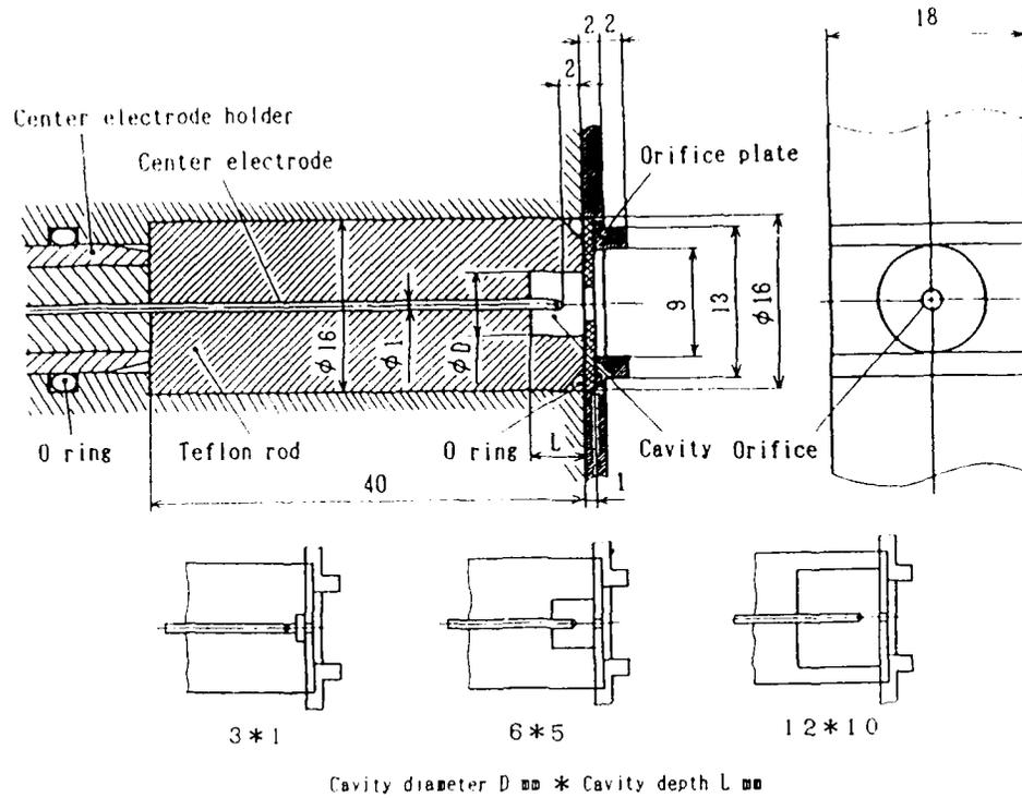
Fig.1 Cross section of plasma jet igniter and three kinds of cavity. Three different cavity are 3\*1, 6\*5 and 12\*10. Symbol of 3\*1 denotes the cavity diameter D of 3 mm and the cavity depth L of 1 mm. Each volume is about 7.1, 141.4 and 1131.0 mm<sup>3</sup>.
