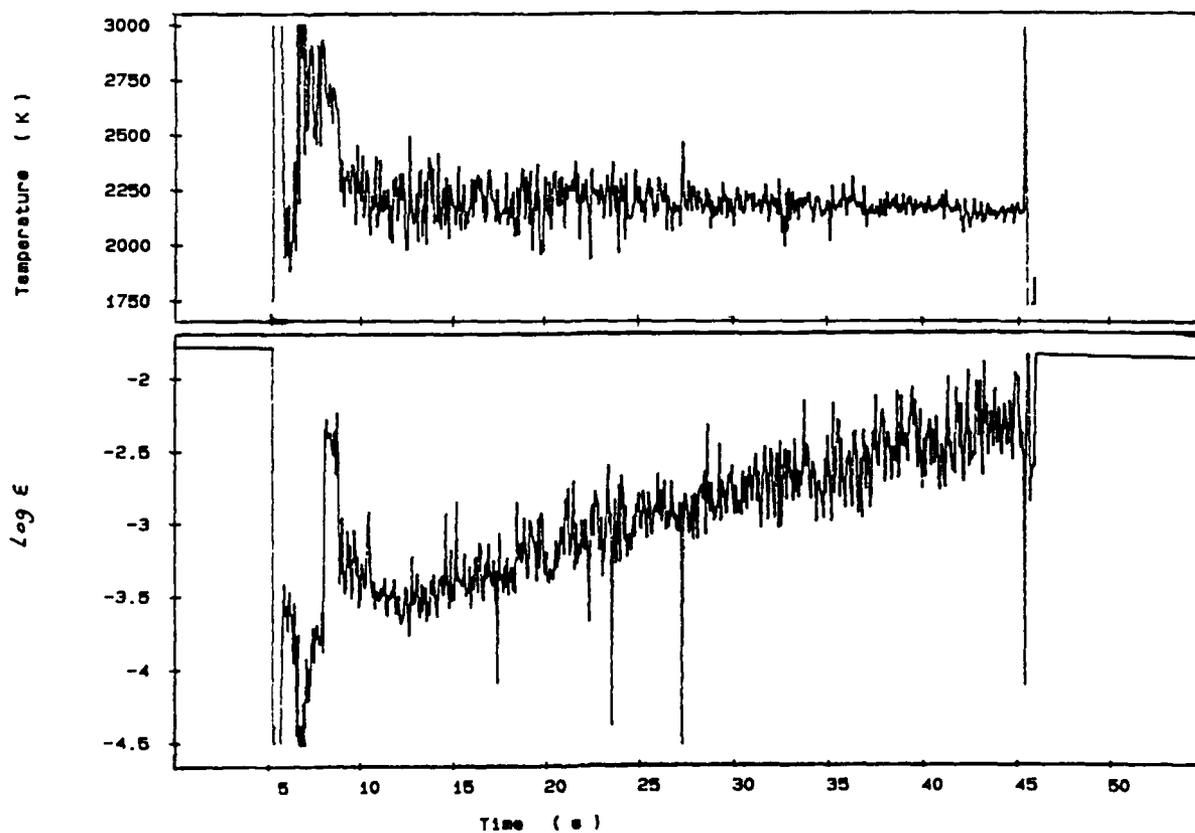
Figure 5 Two-colour temperature (top) and emissivity (bottom)
