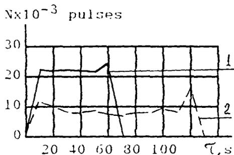
Fig. 2. Plot of registrations of AE signal intensity under explosive material combustion in a chamber with holes: 1 - 3 mm  $\phi$ , 2 - 4 mm  $\phi$ ;
