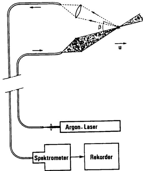
Fig. 1 Optical arrangement for flow velocity measurements
