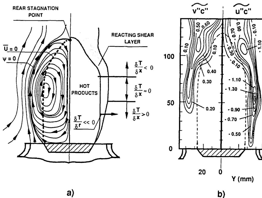
Figure 4. Bluff-body stabilized flame characteristics:
