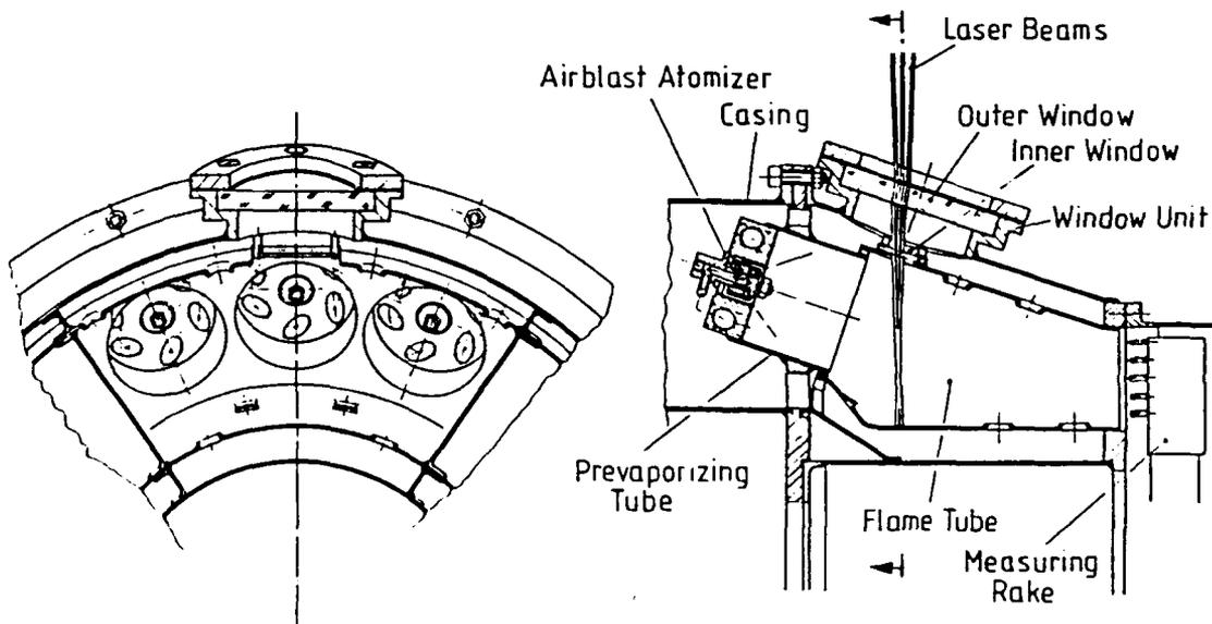
Figure 1. Combustor segment with window unit
