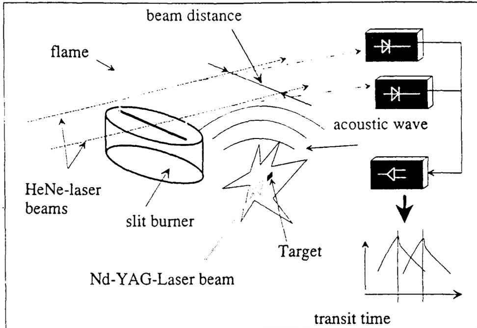
Fig.1 Temperature measurement by opto-acoustic laser beam deflection
