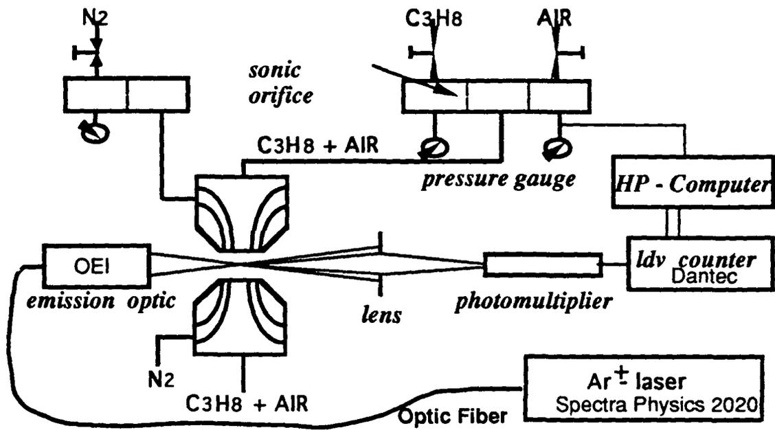
Fig.2. Sketch of the experimental set-up including the LDA system, burners and electronic equipment.
