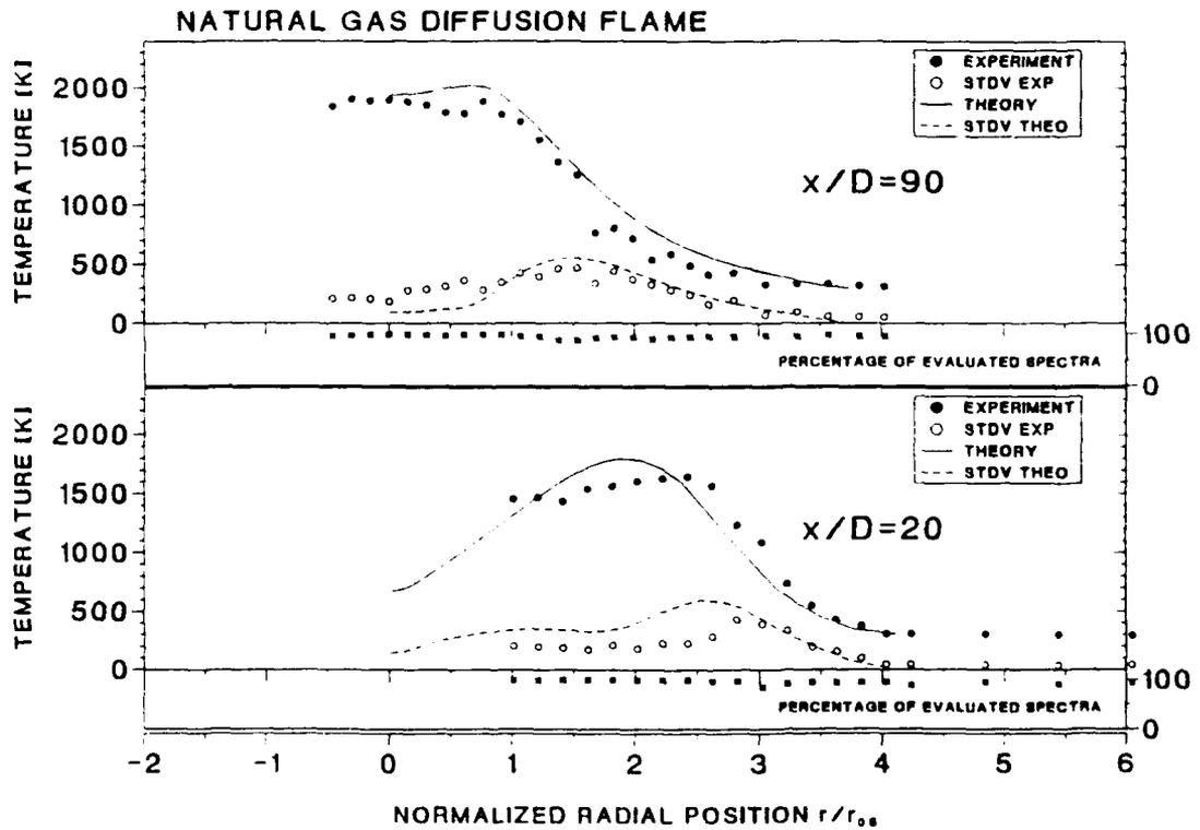
FIG. 2: Experimental and numerical simulation values of mean temperature and standard deviation of mean temperature versus the normalized flame radius at the downstream levels  $x/D = 20$  and  $90$ . Nozzle diameter  $D = 4.0\text{mm}$ .
