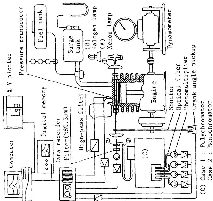
Fig.2 Configuration of test equipment A
