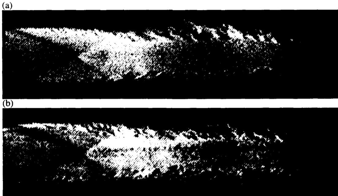
Figure 2. Reacting supersonic coaxial jets. High-temperature fuel-rich center jet is seeded with aluminum oxide particles. Cold oxygen-rich outer jet is unseeded. (a) circular nozzle with lip thickness  $t/D=0.09$ , (b)  $t/D=0.22$ .
