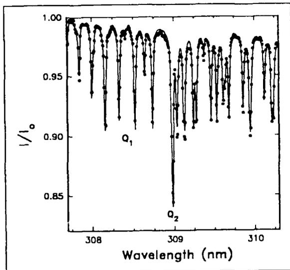
OH Absorption Spectrum Taken in a Lean CH<sub>4</sub>/N<sub>2</sub>O Flame.
