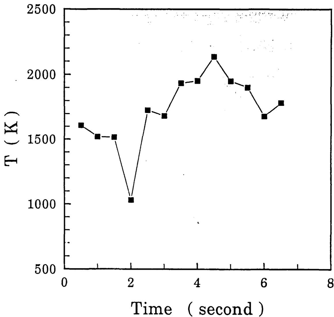
Temperature Variation of the Combustion of Sample A.
