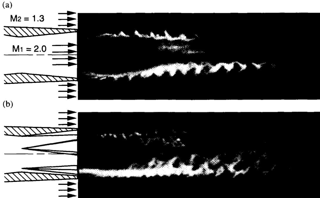
Figure 1. Planar Mie scattering images of supersonic coaxial air jets. The center jet is seeded with ethanol vapor and the outer jet is unseeded. (a) circular nozzle, (b) nozzle with five swept ramps on the expansion side.
