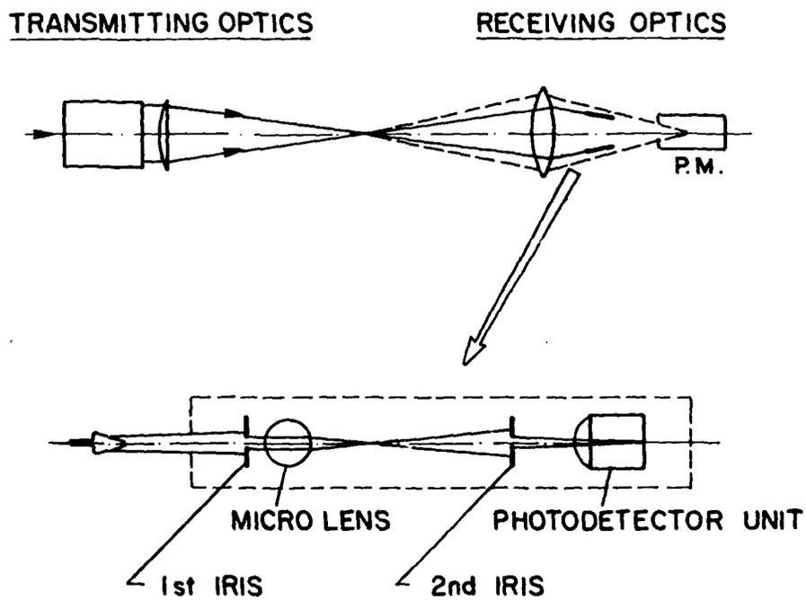
Fig. 2. LDA flow speed and particles size measurement<sup>21</sup>.
