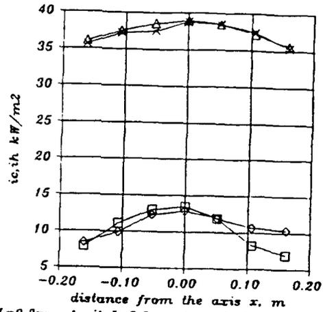
Fig. 2. Measured values of radiation intensity with cold- and hot background.
