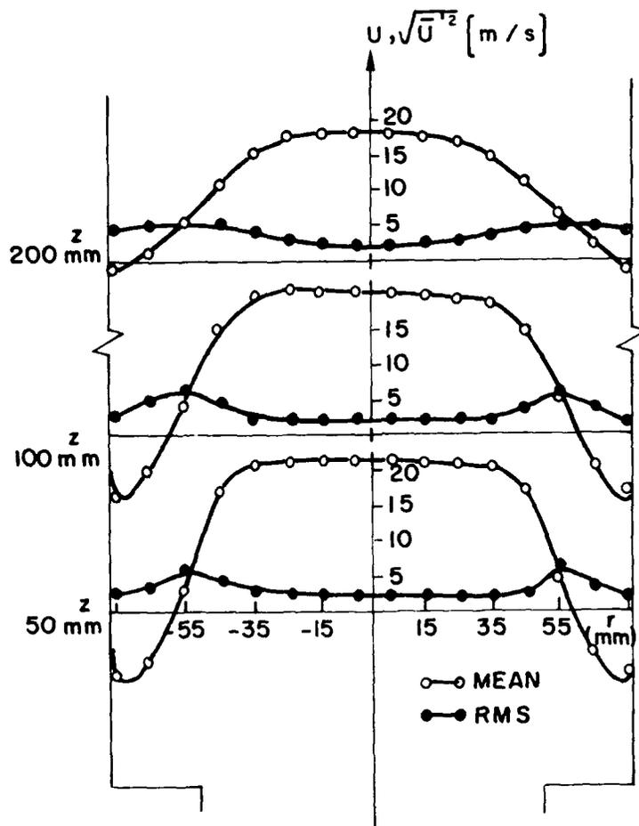
Fig. 3. Mean and r.m.s. velocity measurement by LDA<sup>22</sup>.
