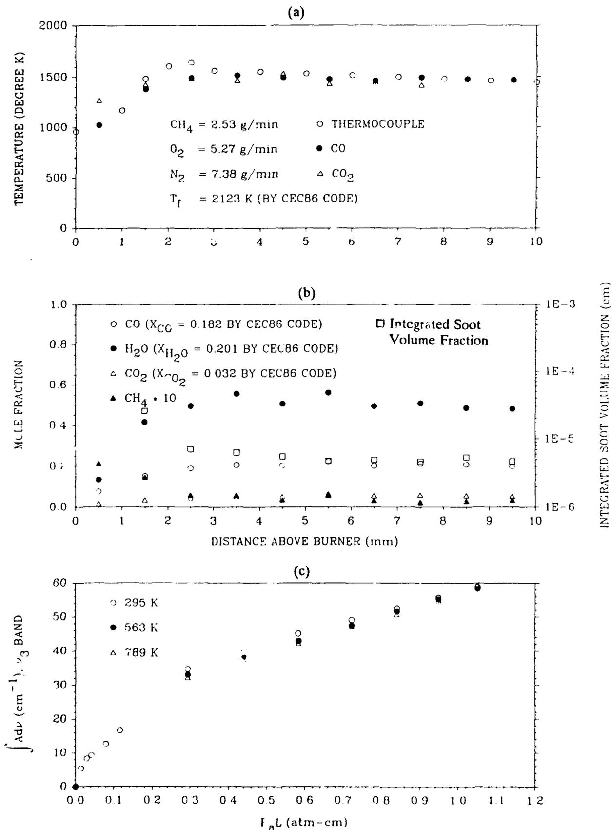
Fig. 1 Measured profiles of temperature, absolute species mole fractions, and integrated soot volume fraction in a premixed CH<sub>4</sub>/air flame with an equivalence ratio  $\phi = 1.94$ , as well as calibration data between integrated absorbance and partial pressure of CH<sub>4</sub>.
