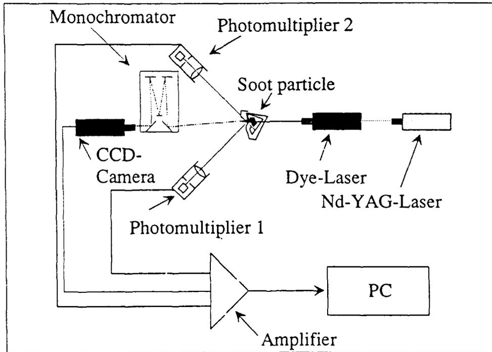
Fig. 2: Scattering light experiment for particle measurement
