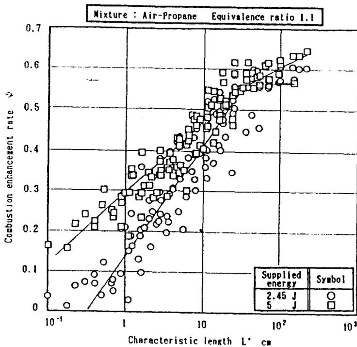
Fig.4 Combustion enhancement rate  $\phi$  as a function of characteristic length  $L^*$ . Air-propane mixture equivalent ratio:1.1. Here the combustion enhancement rate  $\phi$  is defined by the ratio of the burning time of the plasma jet ignition  $\tau_{pl}$  and that of the conventional ignition  $\tau_{con}$ .  $\phi$  is expressed by the equation;  $\phi = 1 - \tau_{pl} / \tau_{con}$ .
