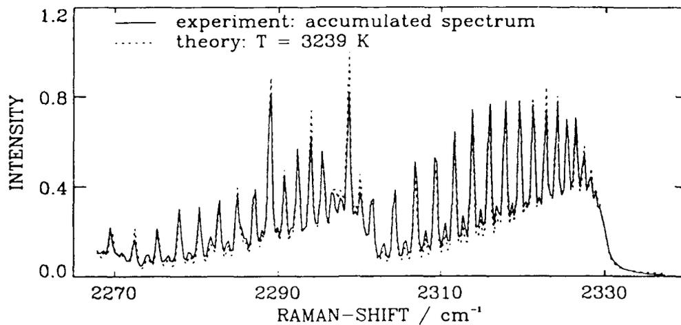
Fig.1: Temperature fit to an experimental nitrogen spectrum consisting of 45 accumulated single shots.
