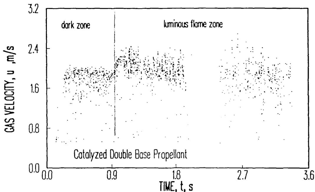
Fig.1 Double Base flame structure by LDA technique.
