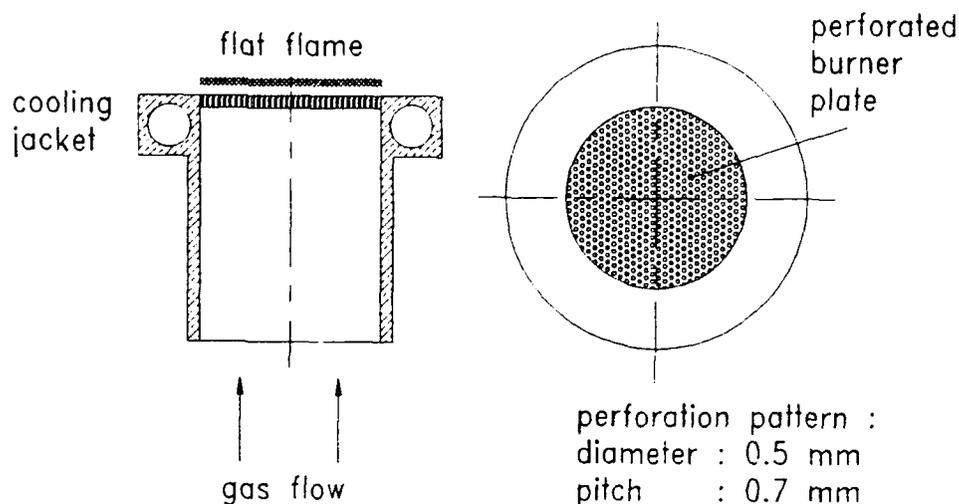
Figure 1: flat flame burner
