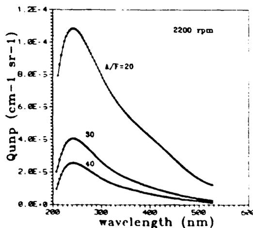
Fig.2 Spectral scattering coefficients at  $90^\circ$  for A/F
