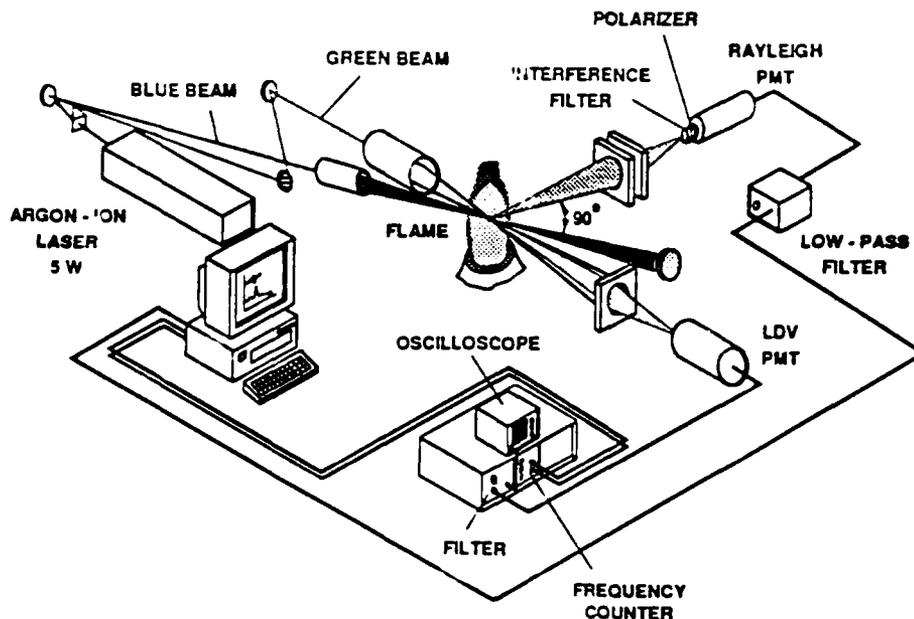
Figure 1. Experimental apparatus developed for the LDV-Rayleigh simultaneous measurements
