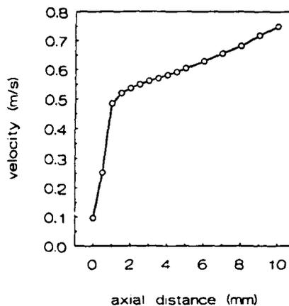
Figure 3: axial burnt gas velocity as function of  $x$ ;  $r = 0$  mm
