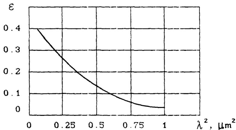
The dependence of spectral emissivity coefficient  $\epsilon$  on  $\lambda^2$  for MgO particles
