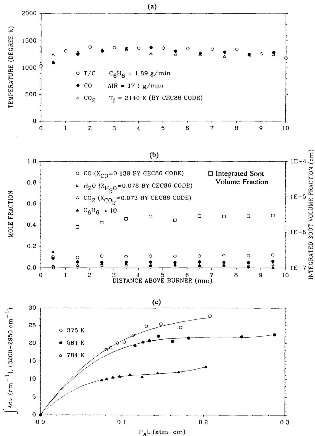
Fig. 2 Measured profiles of temperature, absolute species mole fractions, and integrated soot volume fraction in a premixed  $C_6H_6$ /air flame with an equivalence ratio  $\phi = 1.47$ , as well as calibration data between integrated absorbance and partial pressure of  $C_6H_6$ .
