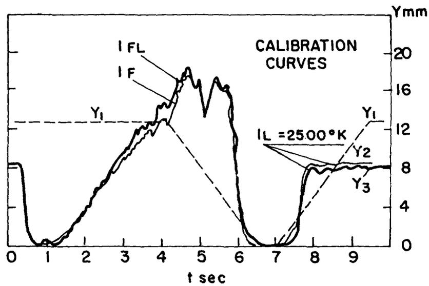
Fig. 1. Experimental radiation curve for polyester-oxygen system, utilizing the line reversal technique<sup>2</sup>.
