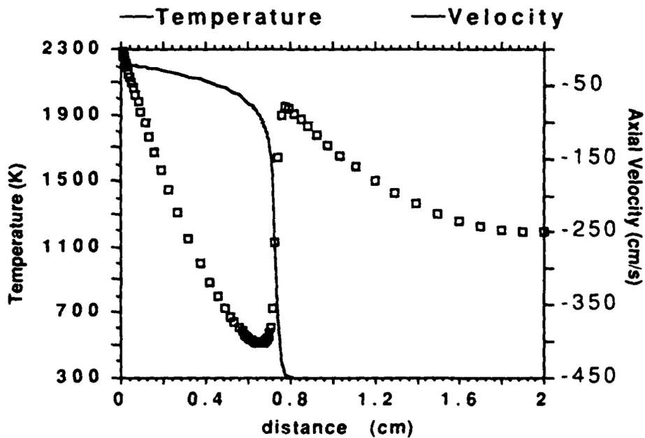
Fig.3. Numerical temperature and axial velocity profiles,  $\phi = 1$ ,  $V_0 = 2.5$  m/s.
