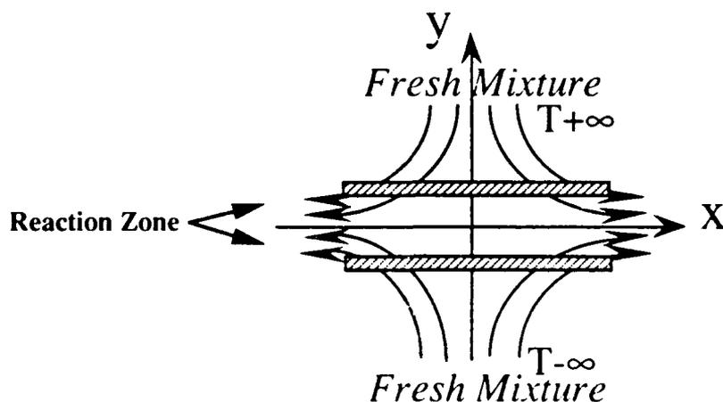
Fig.1. Strained premixed flames formed by counterflow mixtures.
