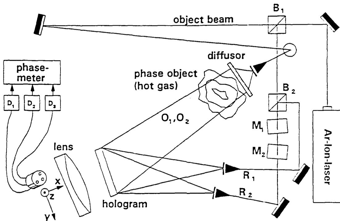
Fig. 1: Concept of the optical set up for heterodyne holographic interferometry
