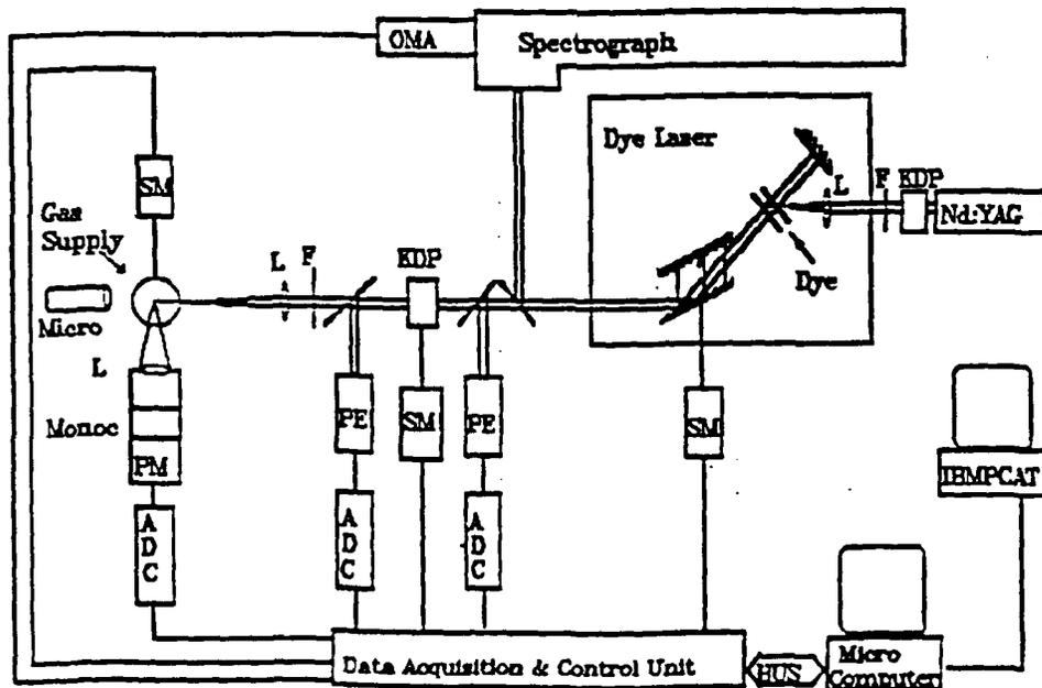
Fig.1. The schematic of the experimental rig.
