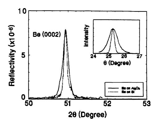
Figure 1. Zero to 20 diffraction and rocking curves (inset) for epitaxial beryllium on silicon and  $Al_2O_3$ . Analyses of the 0-20 spectra yield coherence lengths nearly equal to the film thicknesses.
