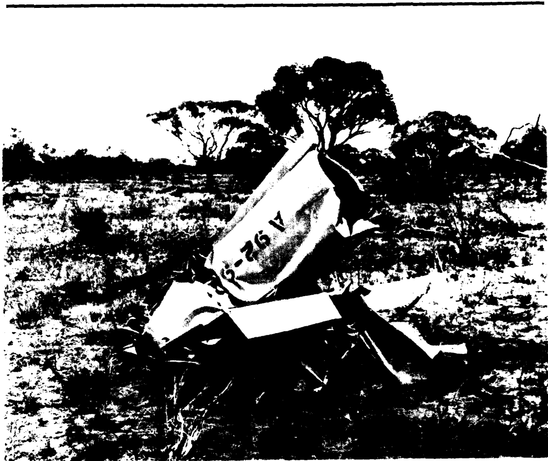
Fig. 33 Tail unit of A92-90 showing damaged elevators with mass balances still attached
