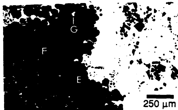
Figure 7 Backscattered electron image of the oxide on NiAl/20 TiB_2 exposed at 1200°C for 25 hours; note the three distinct phases.
