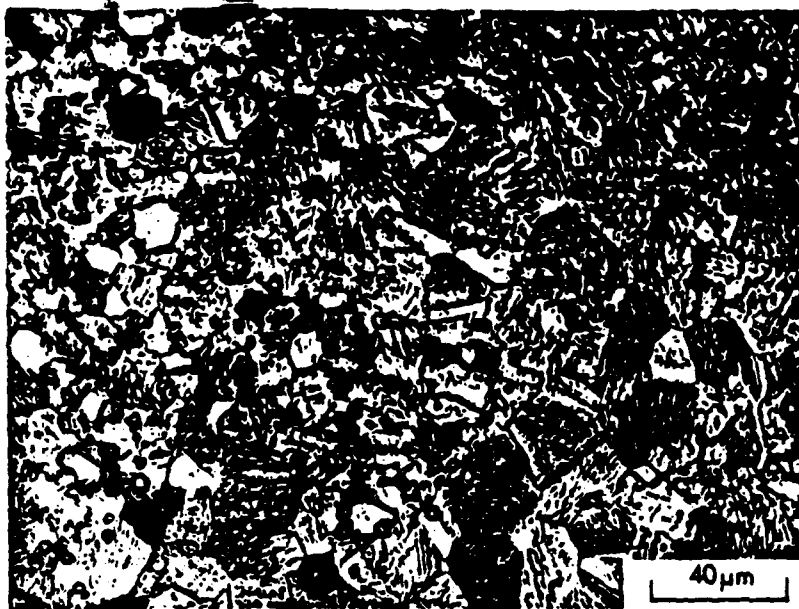
Fig. 17 Optical micrograph of TiAl fabricated by a hybrid reactive sintering and reactive hot isostatic compaction process, using elemental powders and a maximum temperature of 1350°C and 145 MPa pressure. HIP TiAl (60 wt.% Ti, reactd millod, HIP) cycle = 1350 C, 1h, 145 MPa
