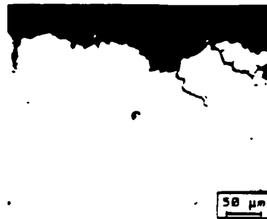
Figure 8. Transverse optical fractograph of fatigue crack in IC 221 tested at 800°C/0.2 Hz.
