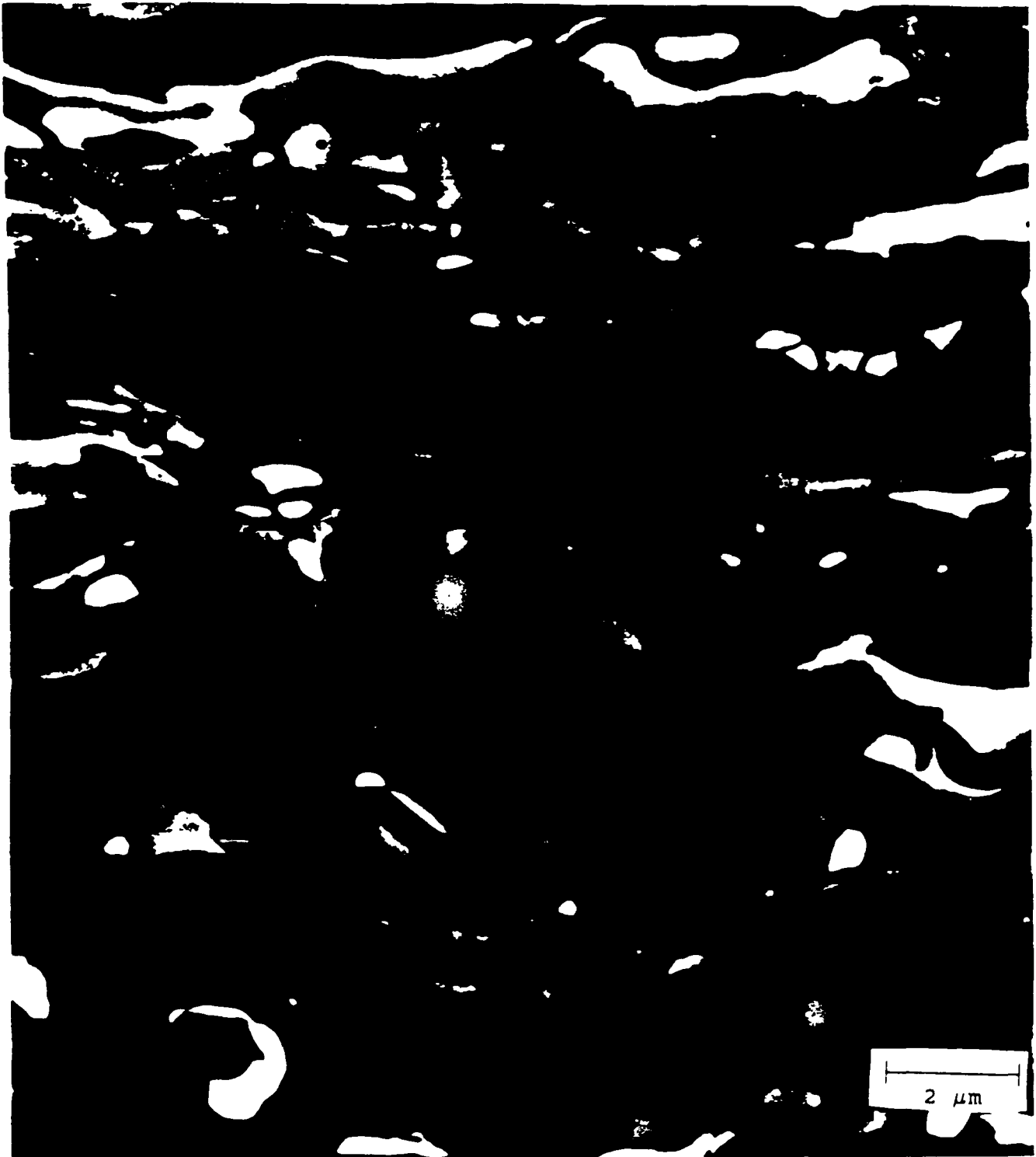
Fig. 7. Higher magnification view of as-deposited laminate in SEM backscatter mode.
