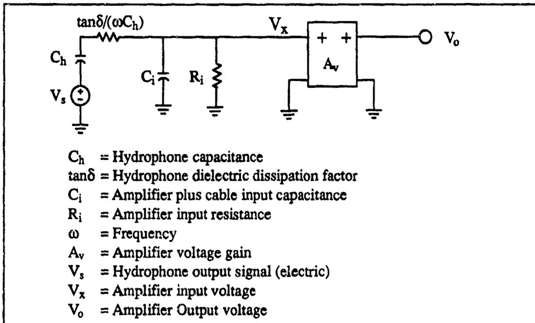
**Figure A-1. Hydrophone/Cable/Amplifier Model**
