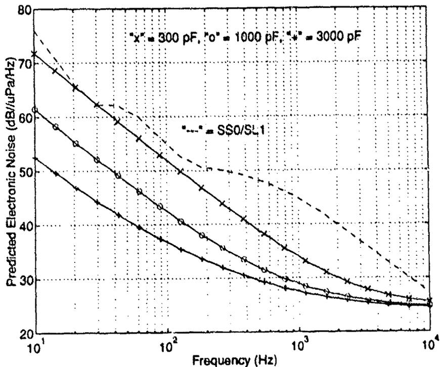
**Figure 6. Predicted Noise Versus Hydrophone Capacitance**
