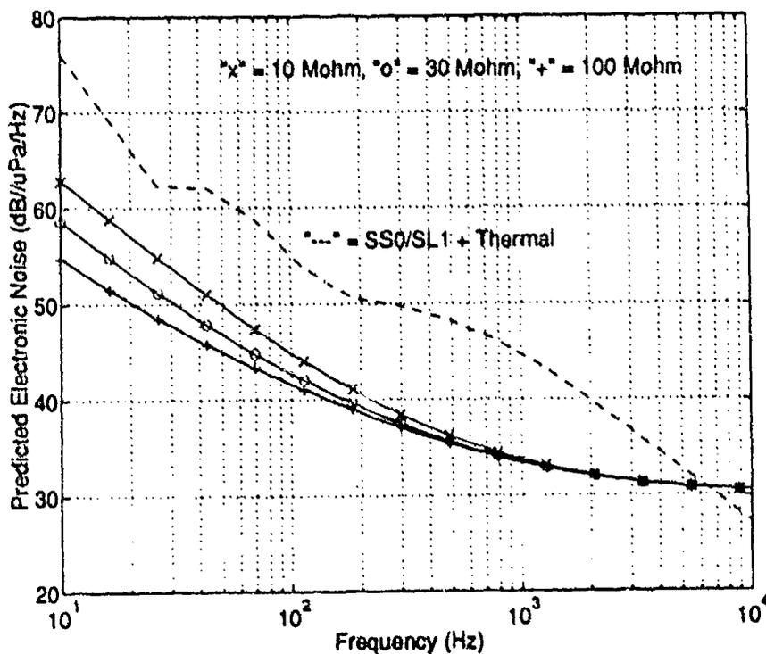
**Figure 5. Predicted Noise Versus Amplifier Input Resistance**
