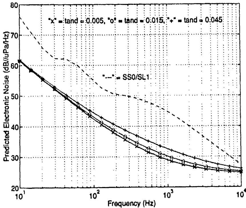
**Figure 7. Predicted Noise Versus Hydrophone Dielectric Loss**
