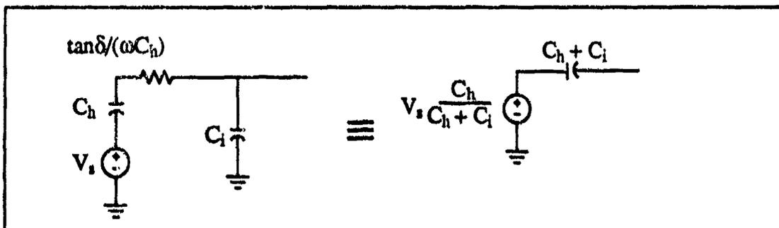
**Figure A-2. Hydrophone/Cable Thévenin Equivalent Circuit ( $\tan\delta \ll 1$ )**
