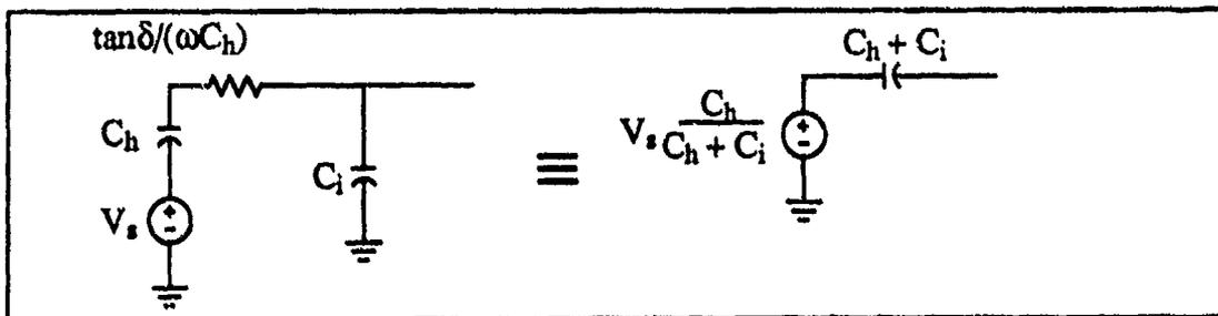
**Figure B-2. Hydrophone/Cable Thévenin Equivalent Circuit ( $\tan\delta < 1$ )**
