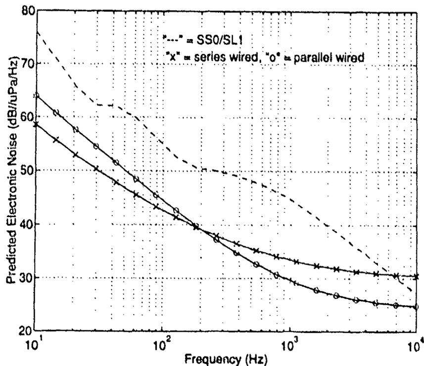
**Figure 4. Predicted Noise Versus Hydrophone Wiring Configuration**
