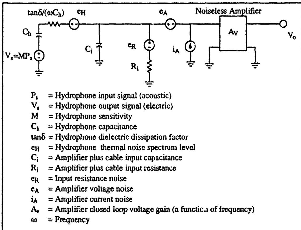
**Figure 2. Hydrophone/Cable/Non-inverting Amplifier Noise Model**
