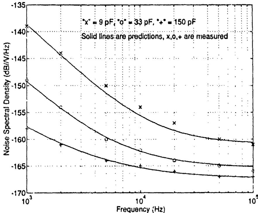
**Figure 11. Measured and Predicted Noise Versus Hydrophone Capacitance**
