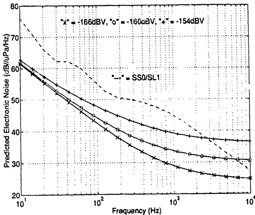
Figure 8. Predicted Noise Versus Amplifier Voltage Noise
