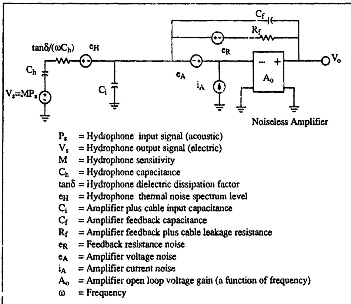
**Figure 3. Hydrophone/Cable/Amplifier Noise Model**
