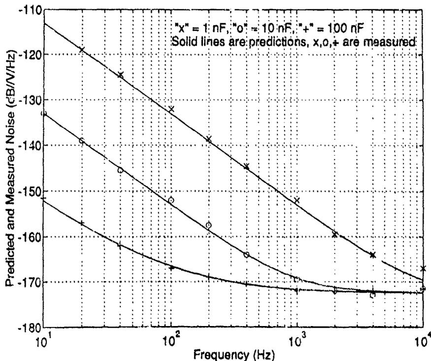
**Figure 10. Measured and Predicted Noise Versus Hydrophone Capacitance**
