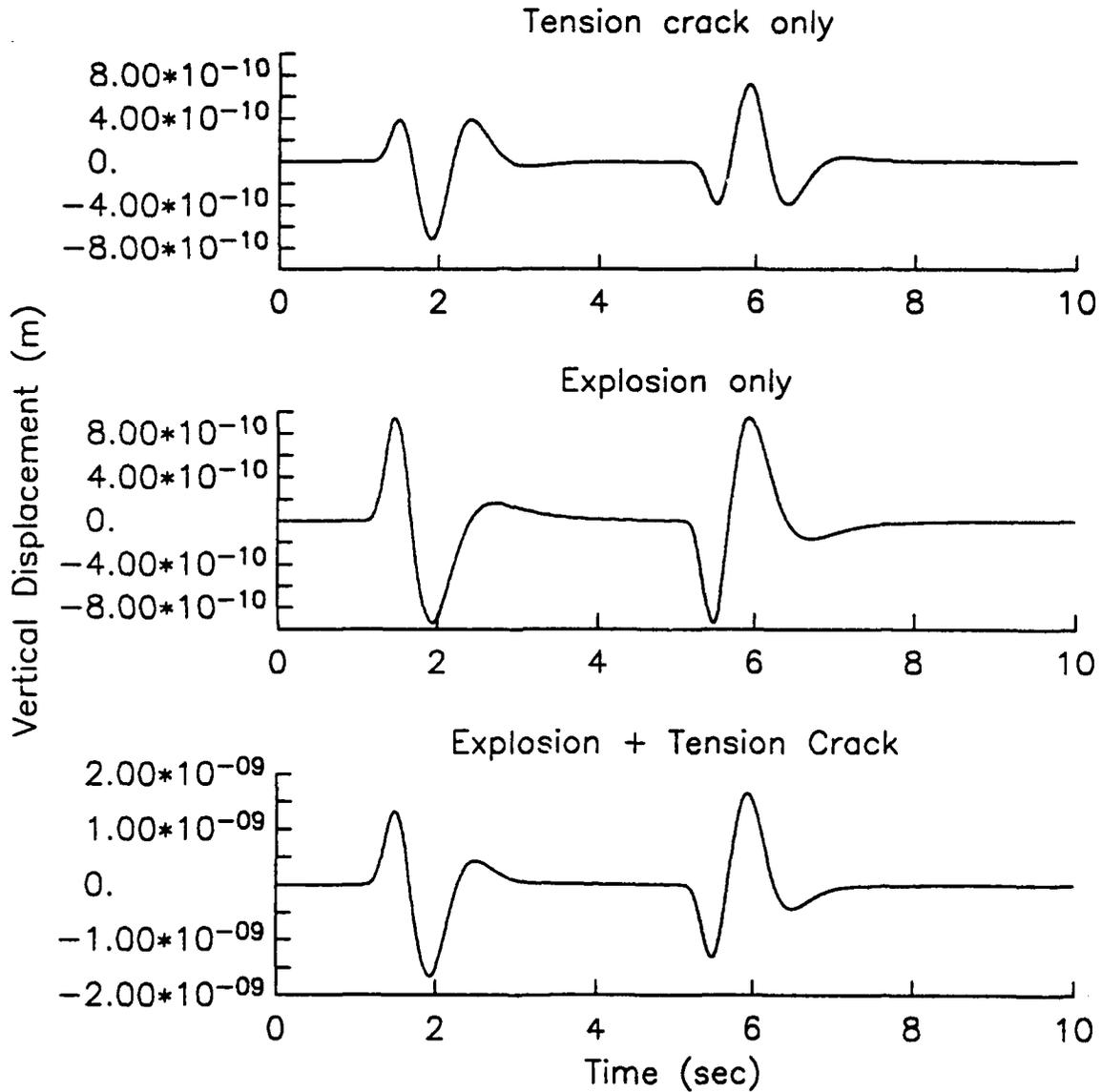
Figure 31. Teleseismic P wave synthetic seismograms of the quarry blast filtered with a short period SRO instrument response showing the contributions of the spall phase alone (top), of the explosive charges (middle) and the sum (bottom).
