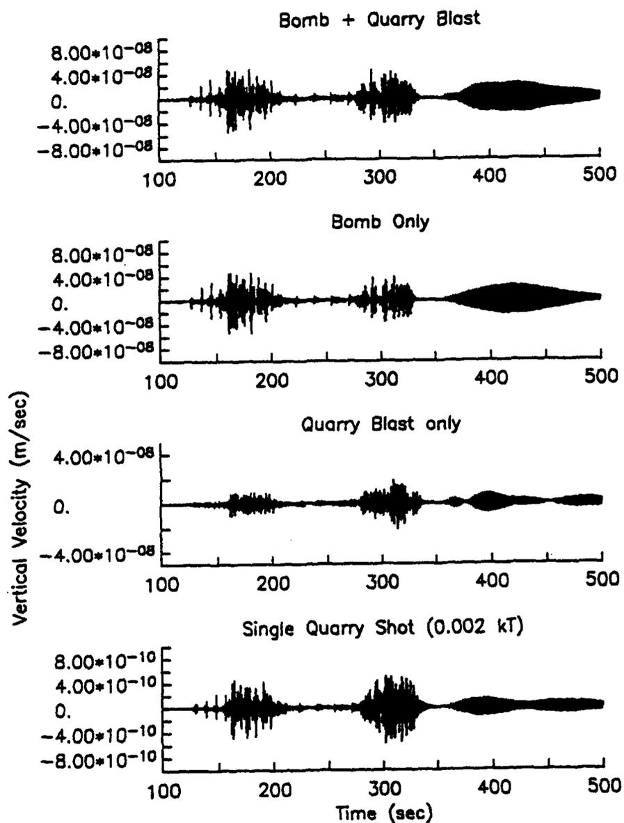
Figure 28. Regional narrow band synthetic seismograms (0.75 to 5.0 Hz): from top to bottom; the sum of the quarry blast simulation plus the tamped 1 KT explosion, the tamped 1 KT explosion alone, the quarry blast simulation alone, a single hole in the quarry blast.
