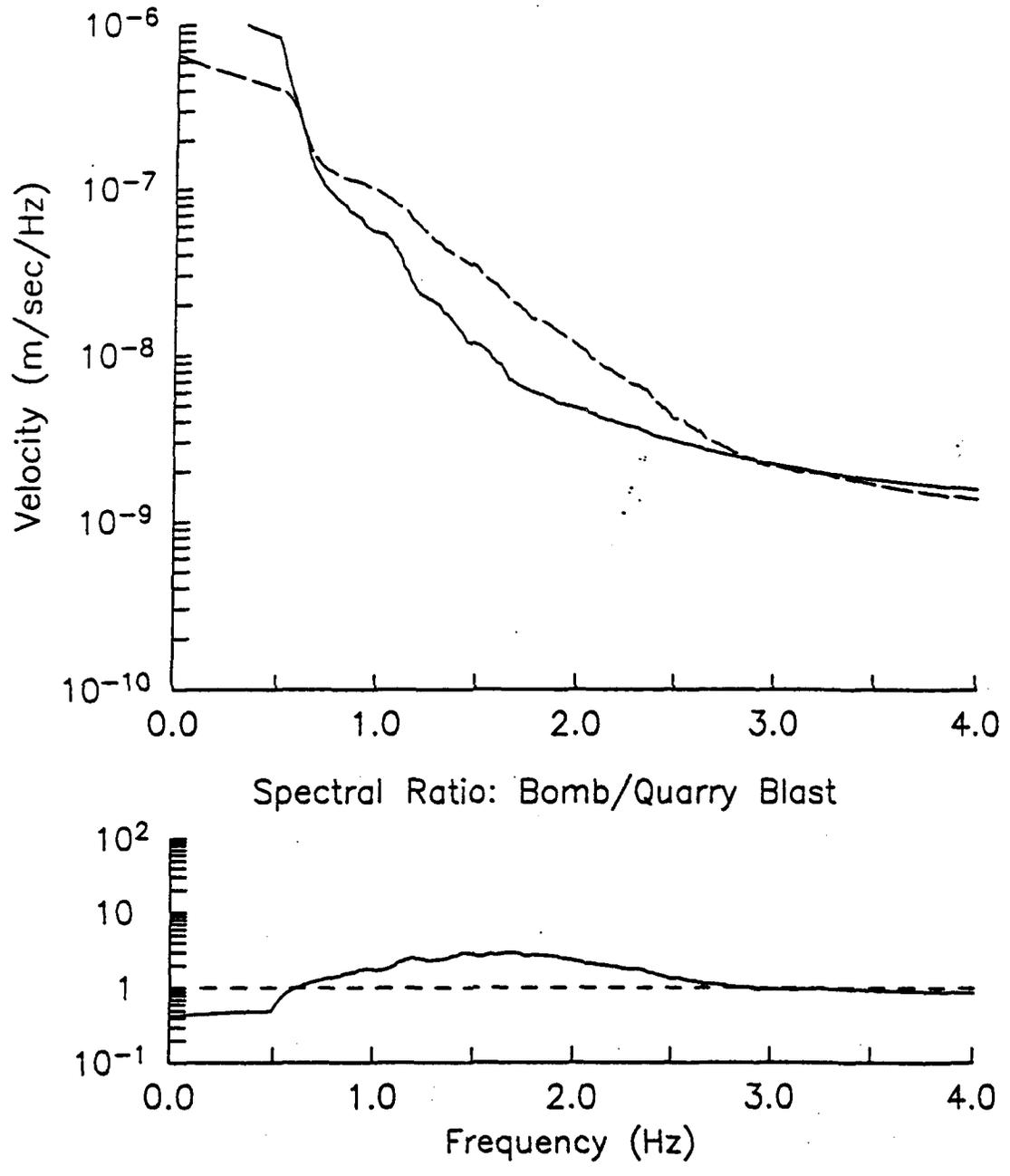
Figure 22. (top) Smoothed Lg spectra from the quarry blast (solid line) and the 1 KT bomb (dashed line). (bottom) Ratio of top spectra.
