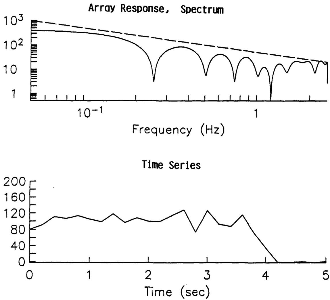
Figure 20. The response of the shot array for the 20x25 quarry: rows fired at 0.2 sec intervals with a 0.25 sec standard deviation in firing times. Dashed line on spectrum shows a line with slope  $f^{-1}$ .
