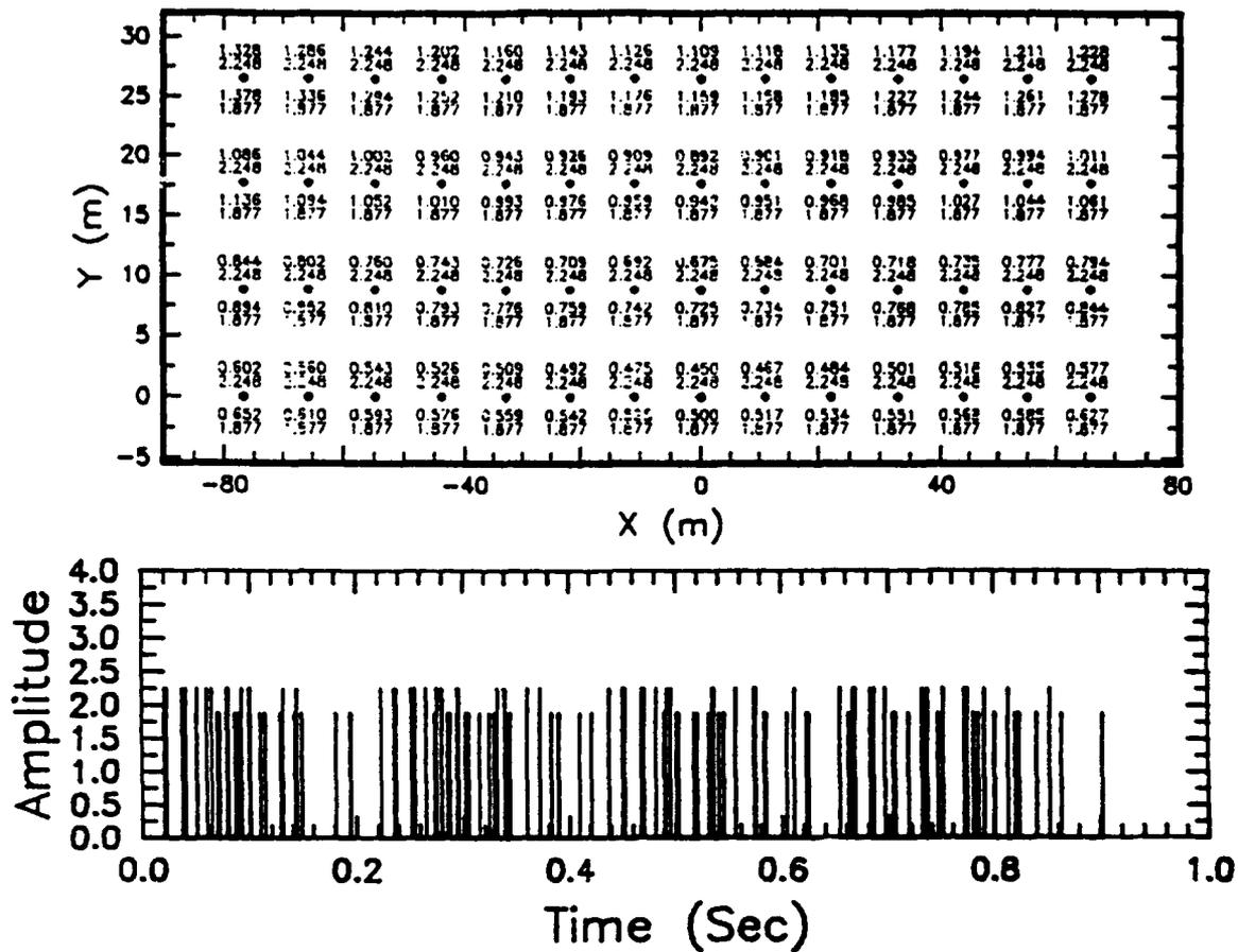
Figure 3. Example of a 0.1 KT quarry blast shot layout from Chapman, *et al.* (1991). (Top) Shot locations; written above each shot location are the charge size (in thousands of lbs) over the delay time in msec. (Bottom) shot size versus time.
