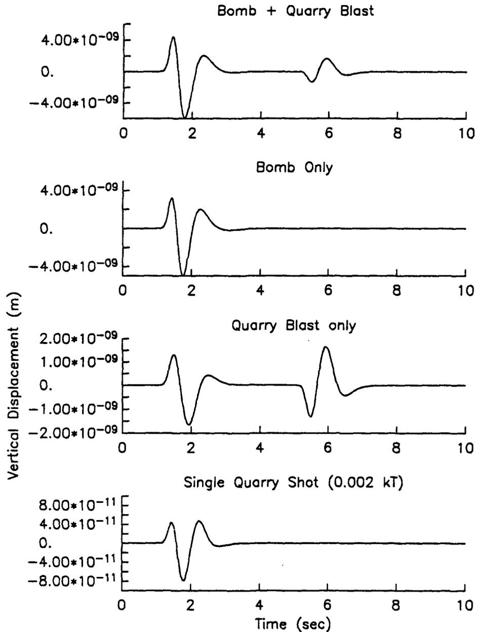
Figure 30. Teleseismic P wave synthetic seismograms filtered with a short period SRO instrument response: from top to bottom; the sum of the quarry blast simulation plus the tamped 1 KT explosion, the tamped 1 KT explosion alone, the quarry blast simulation alone, a single hole in the quarry blast.
