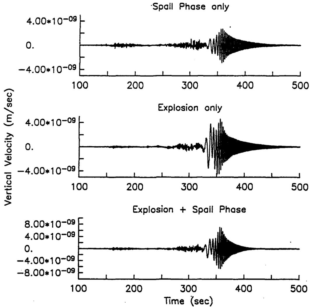
Figure 12. Regional broadband synthetic seismograms from a single shot: from top to bottom; the spall phase alone, the explosive charge alone and the sum of the spall phase and explosive charge.
