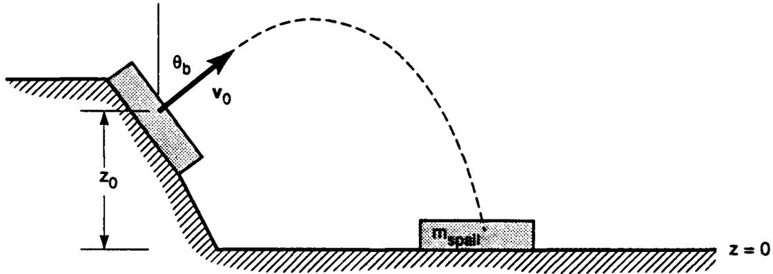
Figure 4. Schematic drawing showing movement of the spall mass.
