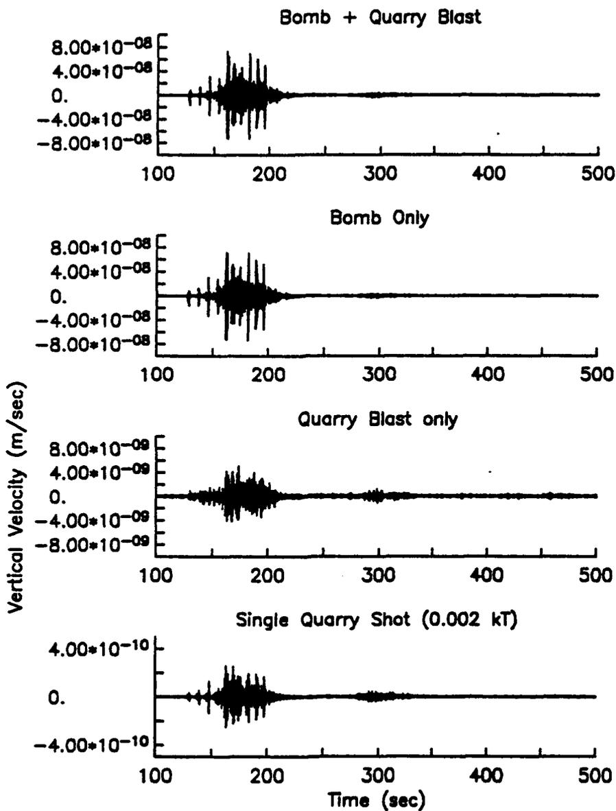
Figure 16. Regional narrow band vertical synthetic seismograms (2.0 to 5.0 Hz): from top to bottom; the sum of the quarry blast simulation plus the tamped 1 KT explosion, the tamped 1 KT explosion alone, the quarry blast simulation alone, a single hole in the quarry blast.
