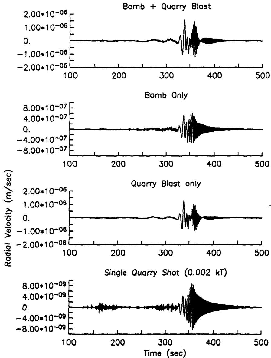
Figure 15. Regional synthetic radial seismograms (unfiltered): from top to bottom; the sum of the quarry blast simulation plus the tamped 1 KT explosion, the tamped 1 KT explosion alone, the quarry blast simulation alone, a single hole in the quarry blast (same as Figure 13, but for radial motions).
