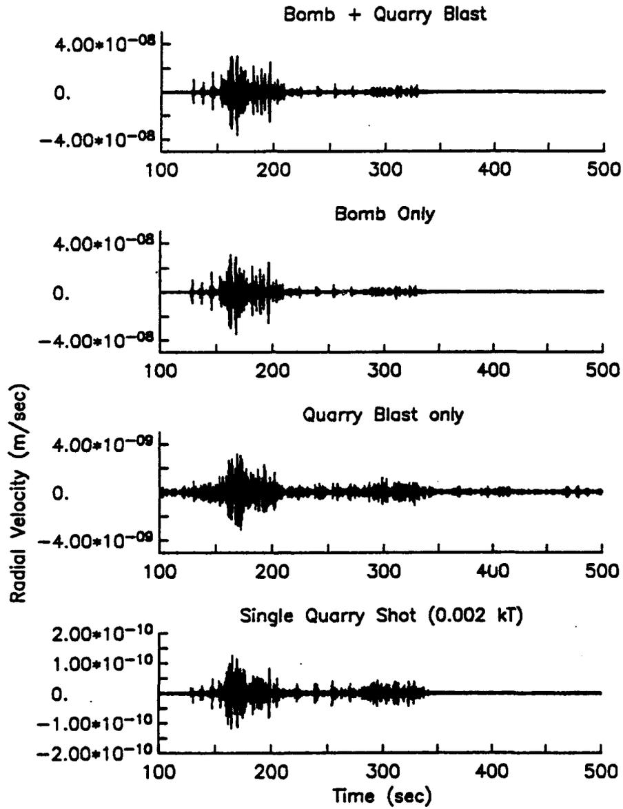
Figure 17. Regional narrow band radial synthetic seismograms (2.0 to 5.0 Hz): from top to bottom; the sum of the quarry blast simulation plus the tamped 1 KT explosion, the tamped 1 KT explosion alone, the quarry blast simulation alone, a single hole in the quarry blast (same as Figure 15, but for radial motions).
