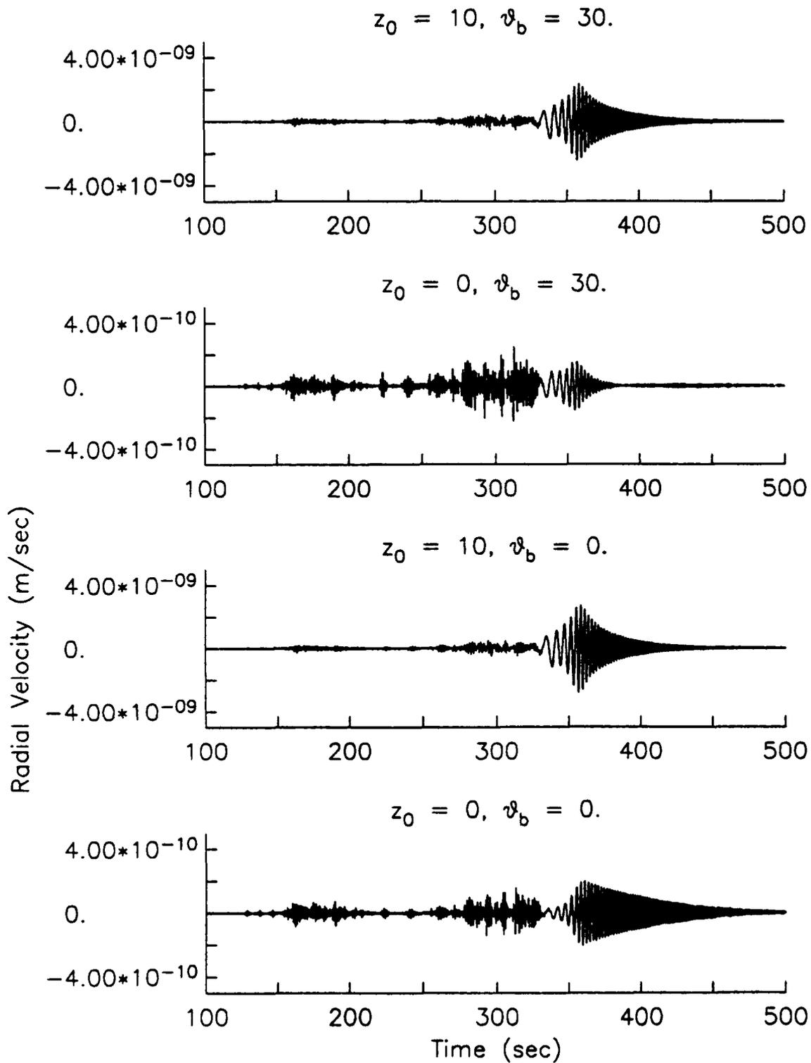
Figure 8. Contributions from the spall mechanism to regional synthetic vertical velocity seismograms at 1000 km (unfiltered) for values of initial height  $z_0$  and trajectory angle  $\vartheta_b$  (same as Figure 7, but for radial motions).
