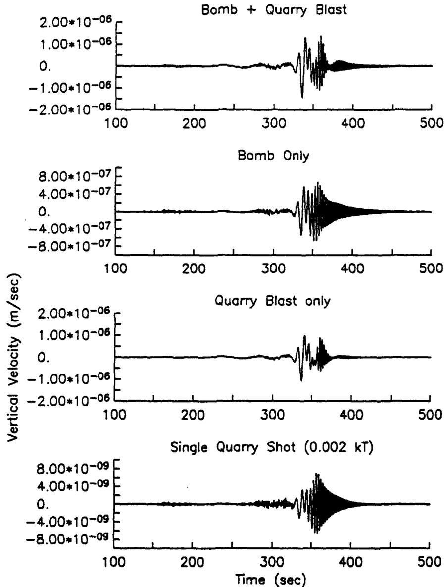
Figure 14. Regional synthetic vertical seismograms (unfiltered): from top to bottom; the sum of the quarry blast simulation plus the tamped 1 KT explosion, the tamped 1 KT explosion alone, the quarry blast simulation alone, a single hole in the quarry blast.
