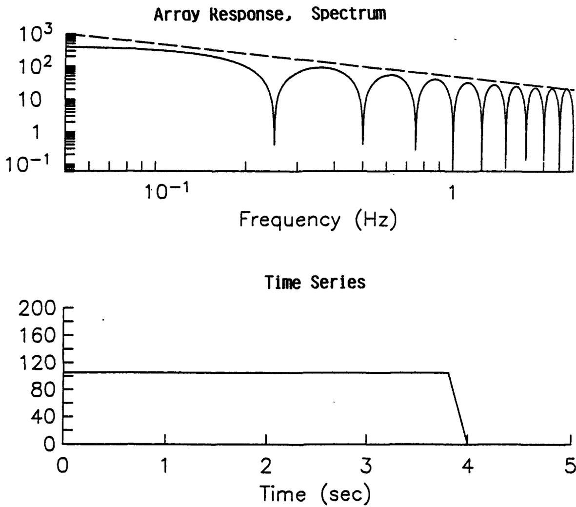
Figure 18. The response of the shot array for the 20x25 quarry: rows fired at 0.2 sec intervals. Dashed line on spectrum shows a line with slope  $f^{-1}$ .
