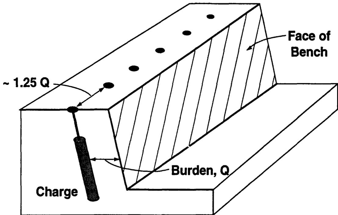
Figure 1. Schematic drawing of a row of charges at the face of a quarry blast.
