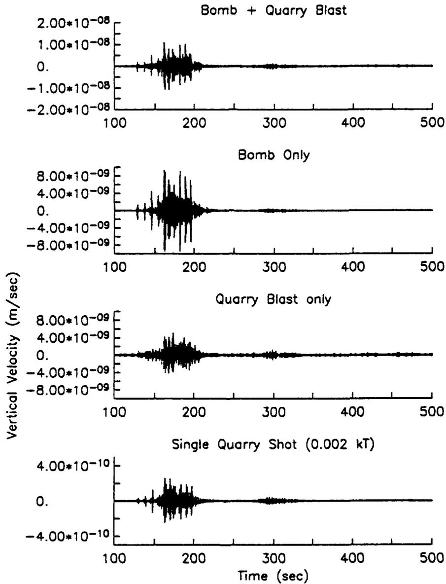
Figure 26. Regional narrow band vertical synthetic seismograms (2.0 to 5.0 Hz): from top to bottom; the sum of the quarry blast simulation plus the tamped 0.1 KT explosion, the tamped 0.1 KT explosion alone, the quarry blast simulation alone, a single hole in the quarry blast.
