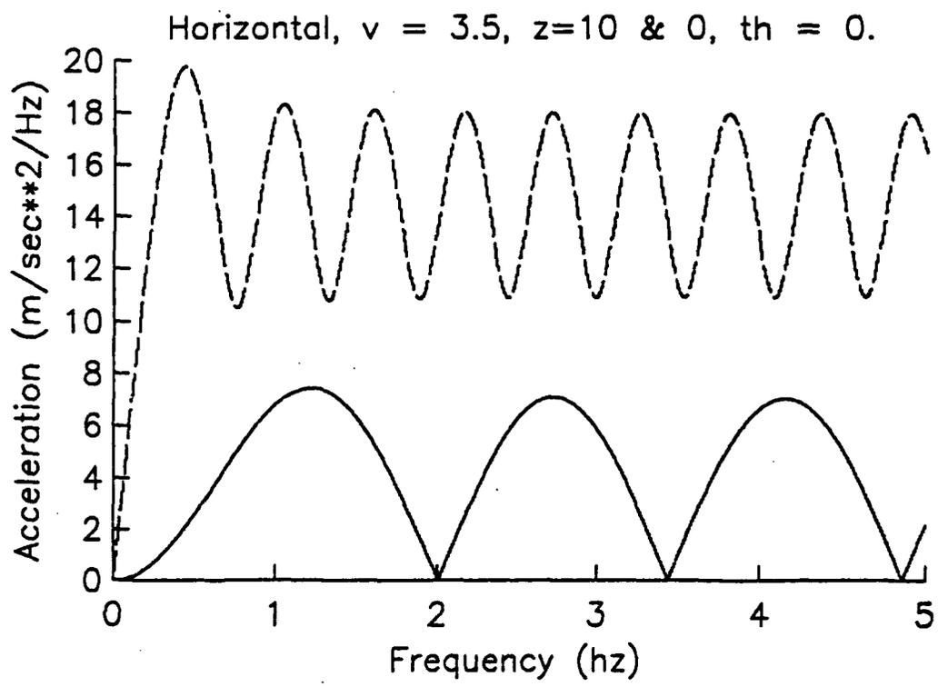
Figure 11. Spall source spectra for  $\theta_b = 0$ , with (top)  $z_0 = 10$ , and (bottom)  $z_0 = 0$ .
