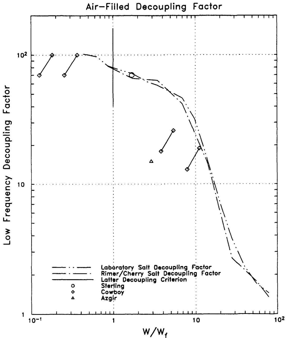
Figure 6. Decoupling factor for an explosion in an air-filled cavity in salt shown as a function of yield divided by the yield of a fully decoupled explosion from calculations by Stevens, *et al* (1991) for two different salt models. Also shown are data points for the Sterling explosion, the Cowboy HE tests, and the 3/29/76 Azgir test.
