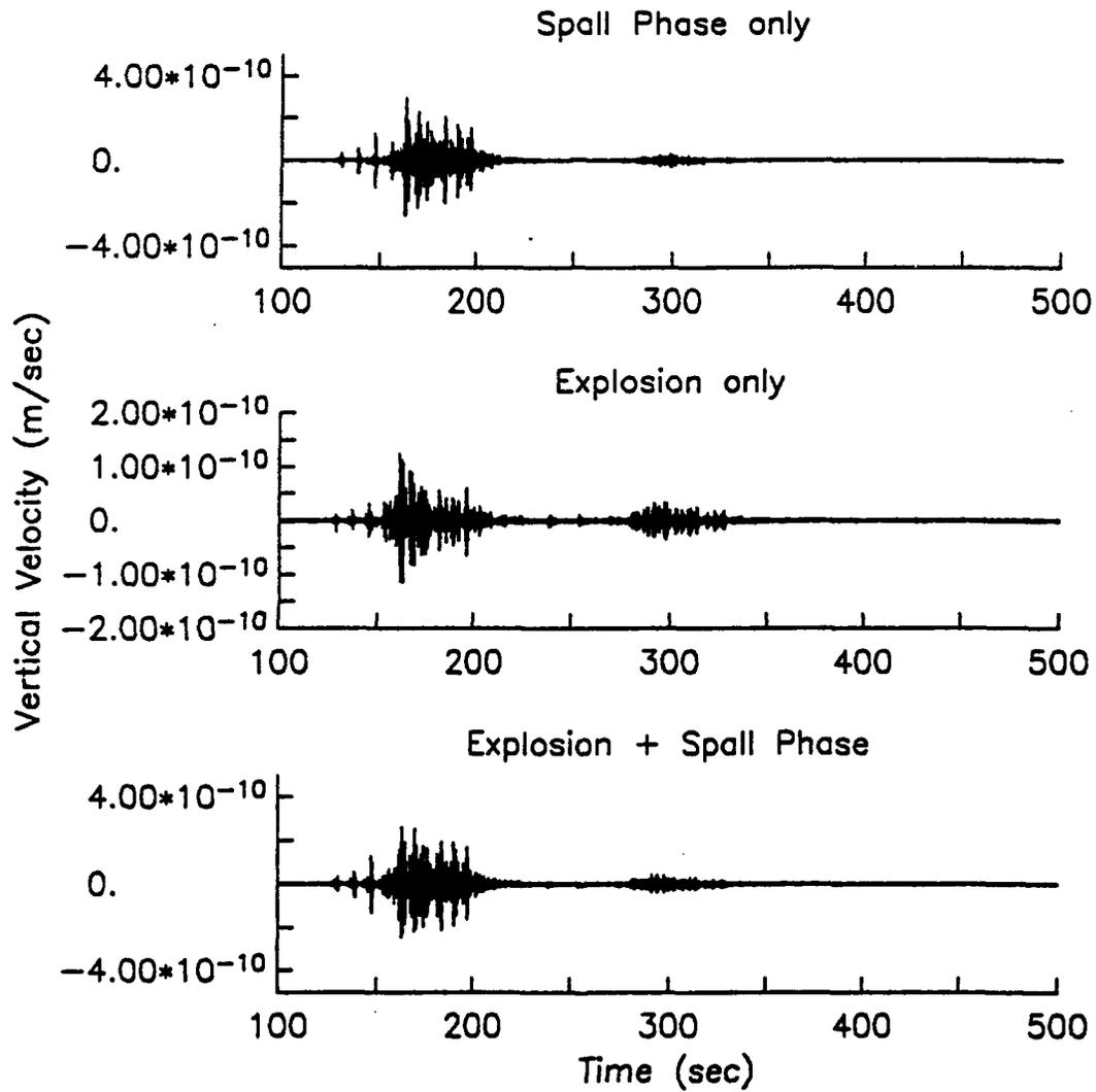
Figure 13. Regional narrow band synthetic seismograms (2.0 to 5.0 Hz) from a single shot: from top to bottom; the spall phase alone, the explosive charge alone and the sum of the spall phase and explosive charge.
