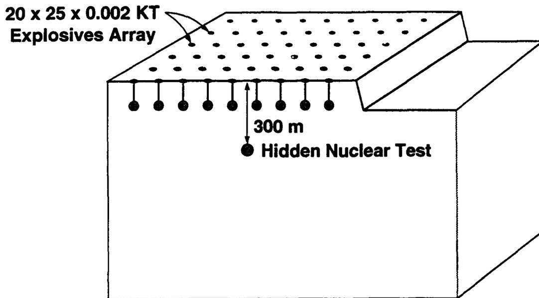
Figure 2. Schematic drawing of the quarry blast model. Calculations were performed for a 1 kiloton quarry blast over a clandestine nuclear test with yields of 0.1 and 1 kilotons. A 0.1 kiloton tamped explosion generates signals comparable to a fully decoupled 7 kiloton explosion or a smaller partially coupled explosion (see Section 2.4).
