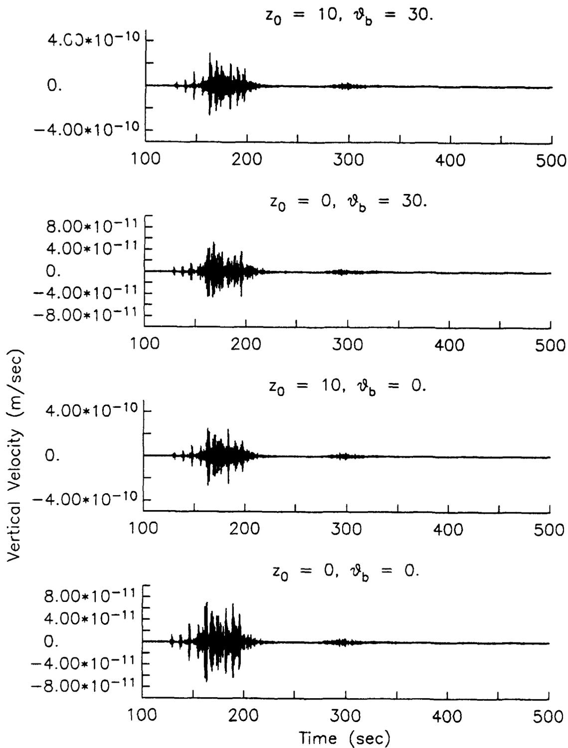
Figure 10. Contributions from the spall mechanism to regional synthetic vertical velocity seismograms at 1000 km (highpass filtered at 2 Hz) for values of initial height  $z_0 = 0, 5$  and 10 m and fixed trajectory angle  $\theta_b$ .
