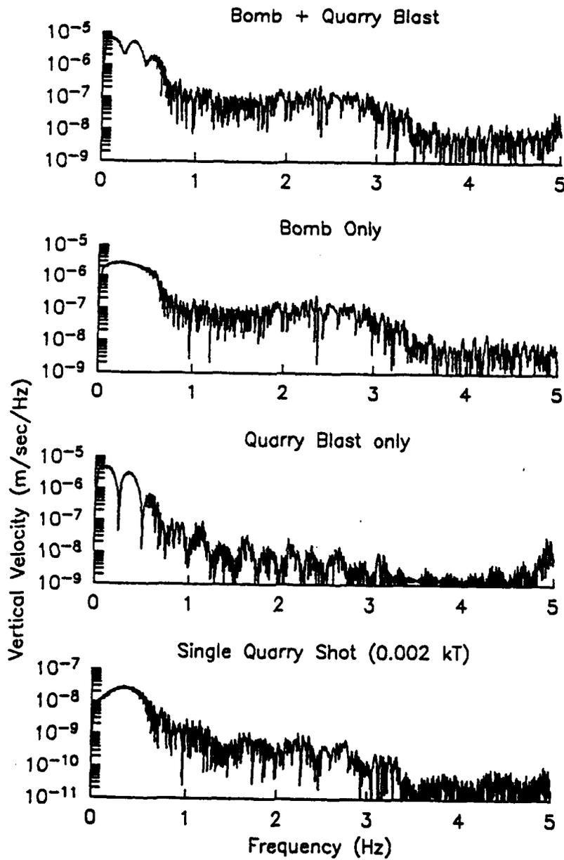
Figure 19. Vertical velocity spectra: from top to bottom; the sum of the quarry blast simulation plus the tamped 1 KT explosion, the tamped 1 KT explosion alone, the quarry blast simulation alone, a single hole in the quarry blast.
