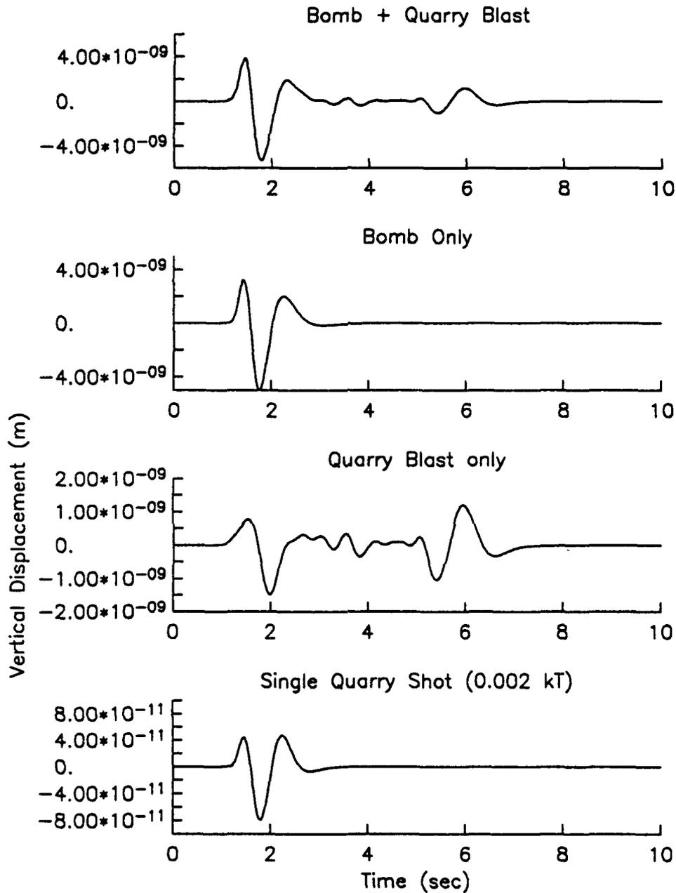
Figure 32. Teleseismic P wave synthetic seismograms filtered with a short period SRO instrument response with a 0.25 sec standard deviation in firing times. From top to bottom; the sum of the quarry blast simulation plus the tamped 1 KT explosion, the tamped 1 KT explosion alone, the quarry blast simulation alone, a single hole in the quarry blast.
