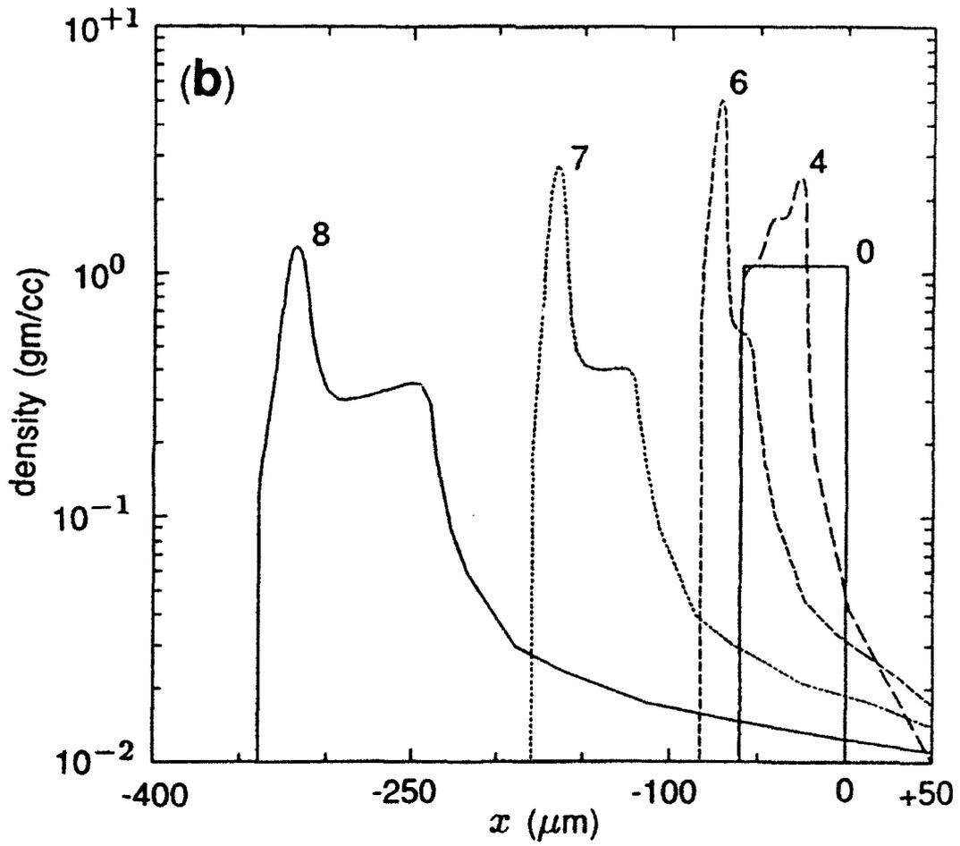
Fig.3 Evolution of the mass density at the listed times for case (b) with an EOS, CRE ionization dynamics, and radiation transfer.
