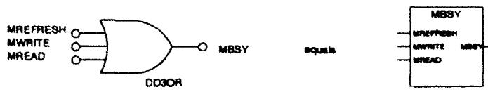
Figure 5.44 MBSY Schematic and Logical Equivalence
