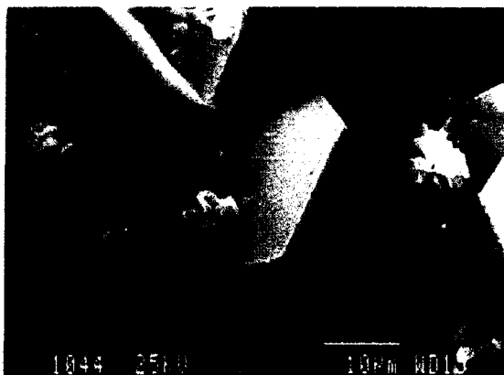
Figure 2: Scanning electron microscope picture of crystals of C_{60} (containing about 15% C_{70} ) as grown from a benzene solution. Pictures of pure C_{60} crystals, where the buckyballs assume fcc structure, look rather similar. At interstitial positions, solvent molecules are built into the lattice. The flat faces of the flake-like crystals are probably (111). (Photo by H.-U. Nissen, ETH Zürich).
