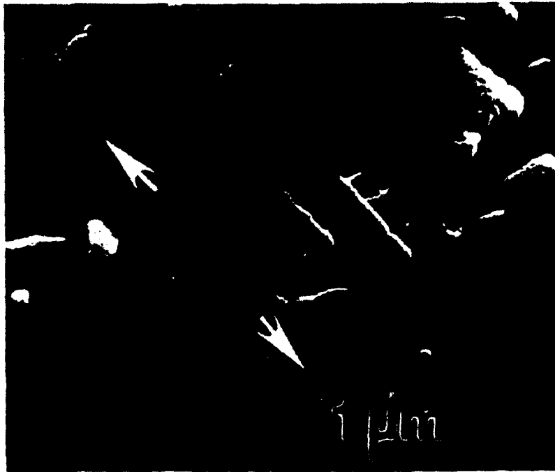
Figure 2. High resolution SEM image of the abalone shell exhibiting the sliding of the \text{CaCO}_3 layers.
