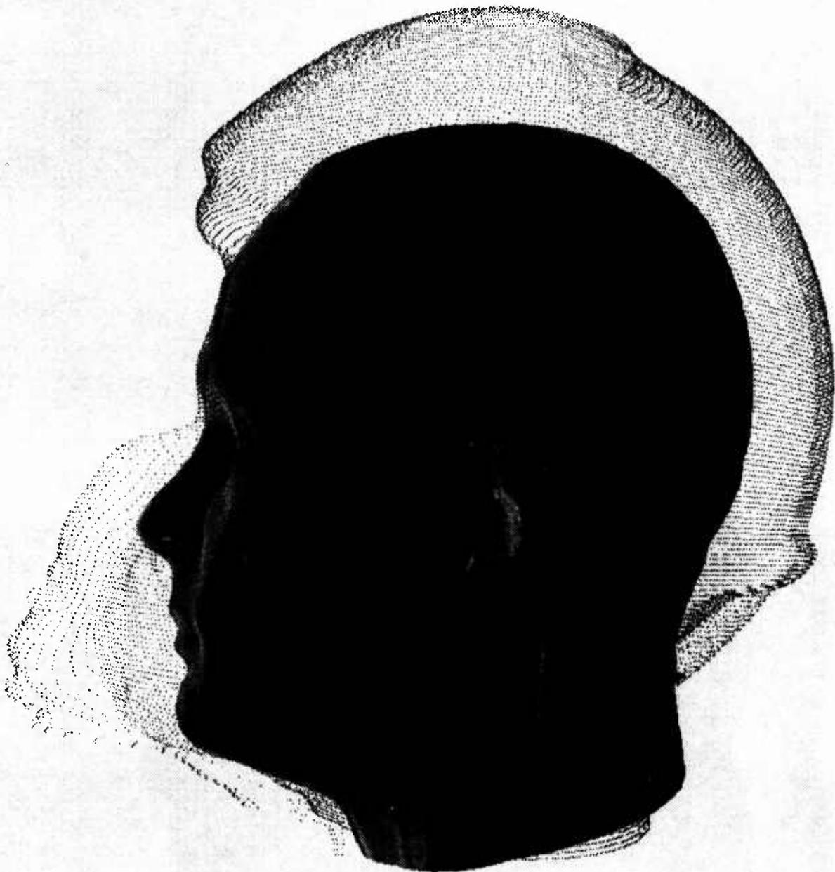
Figure 18. Surfaced scan within the HGU 55/P helmet.
