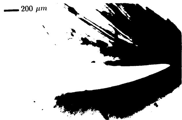
Fig. 9. Distortion of the topograph, possibly as a result of lattice rotation in the Si sample.
