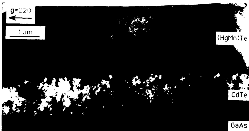
Fig. 6. Dislocation filtering using (HgMn)Te.
