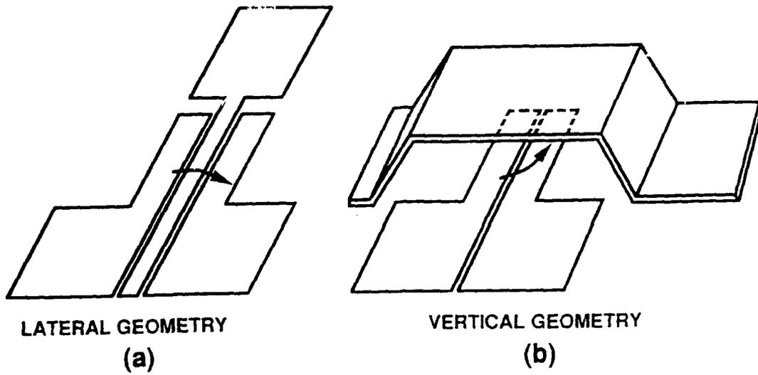
Fig. 8 Anode placement schemes
