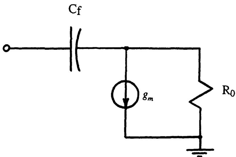
Fig. 4 Simple small-signal model
