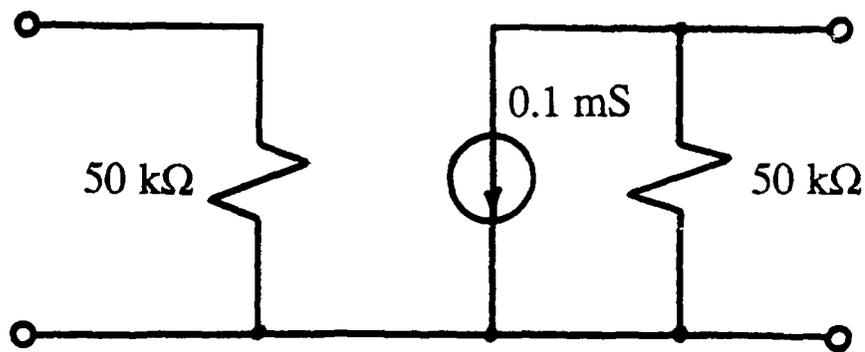
Fig. 9 Equivalent circuit illustrating poor impedance match
