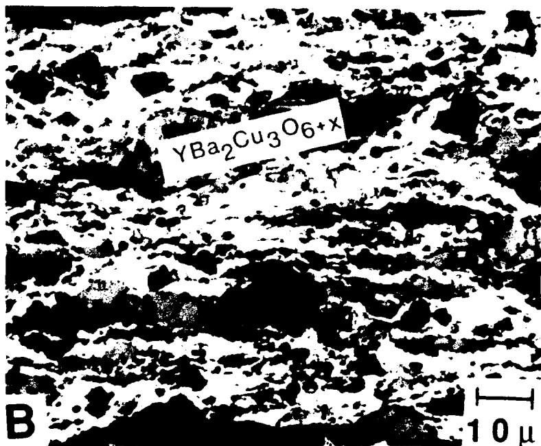
Figure 19. Typical microstructure representing two different regions of the polished surface of a long 60 wt.% aluminum / 40 wt.% \text{YBa}_2\text{Cu}_3\text{O}_{6+x} composite wire. Region (A) represents the uniform distribution of \text{YBa}_2\text{Cu}_3\text{O}_{6+x} and the region (B) represents aggregation of \text{YBa}_2\text{Cu}_3\text{O}_{6+x} particles.
