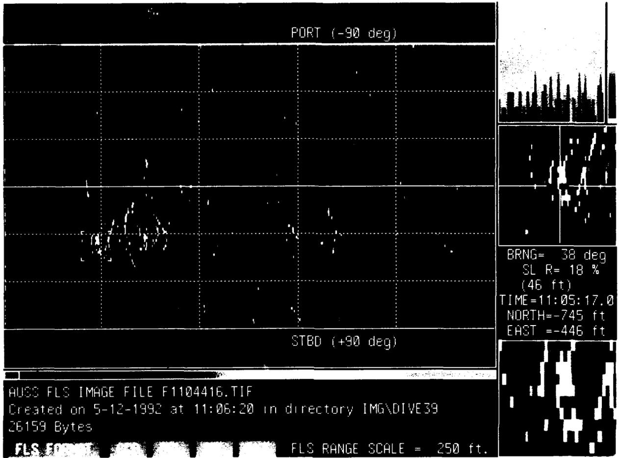
Figure 26. FLS image of wire rope.
