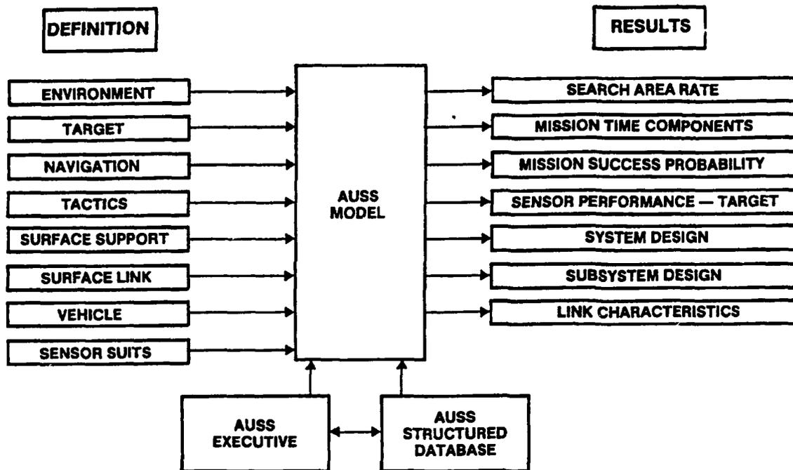
Figure 2. Input and output parameters of the AUSS computer model.
