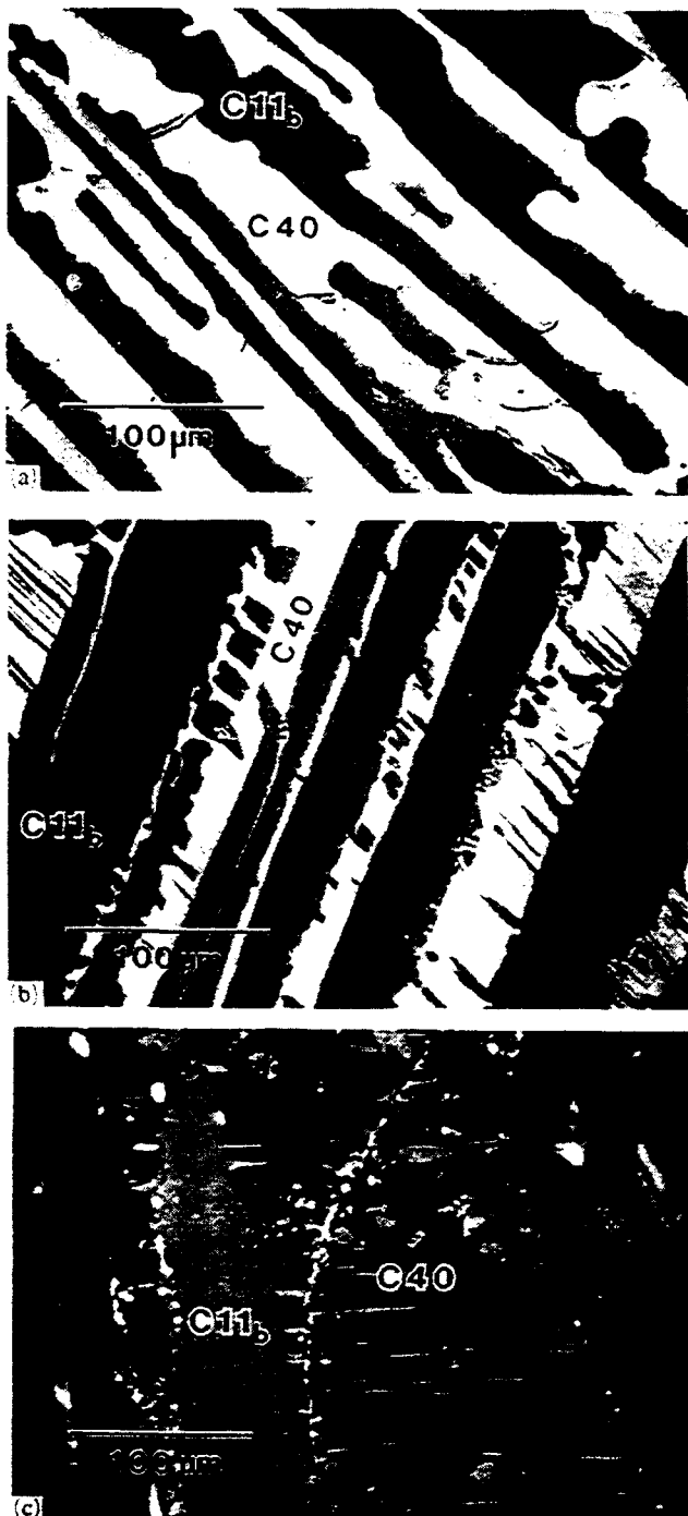
Fig. 15. Micrographs of \text{MoSi}_2 -10 mol.% \text{TaSi}_2 : (a) back-scattered scanning electron micrograph of as-cast material; (b) backscattered scanning electron micrograph of material which had been heat treated for 4 h at 1600 °C; (c) optical micrograph of material which had been heat treated for 110 h at 1300 °C.
