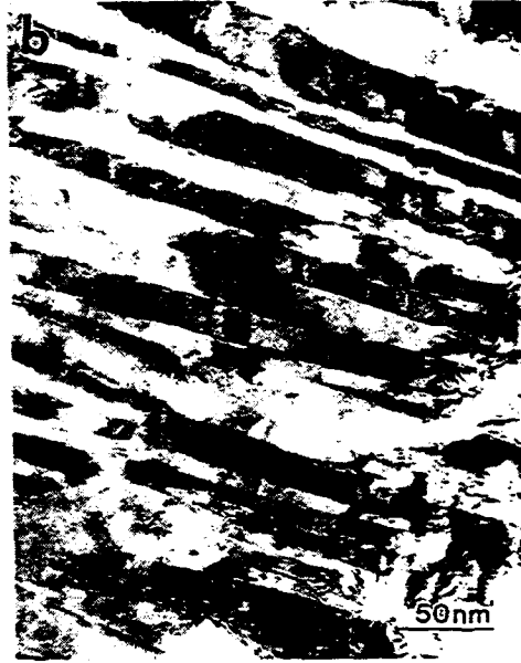
Fig.2 Martensite-type structure ( \mu\text{m} structural scale) observed for slow-cooled specimens. (a) Coarser and needle-like type for the \text{Ti}_5\text{Al}_2\text{Nb} alloy, and (b) much finer and plate-like type for the \text{Ti}_2\text{AlNb} alloy.
