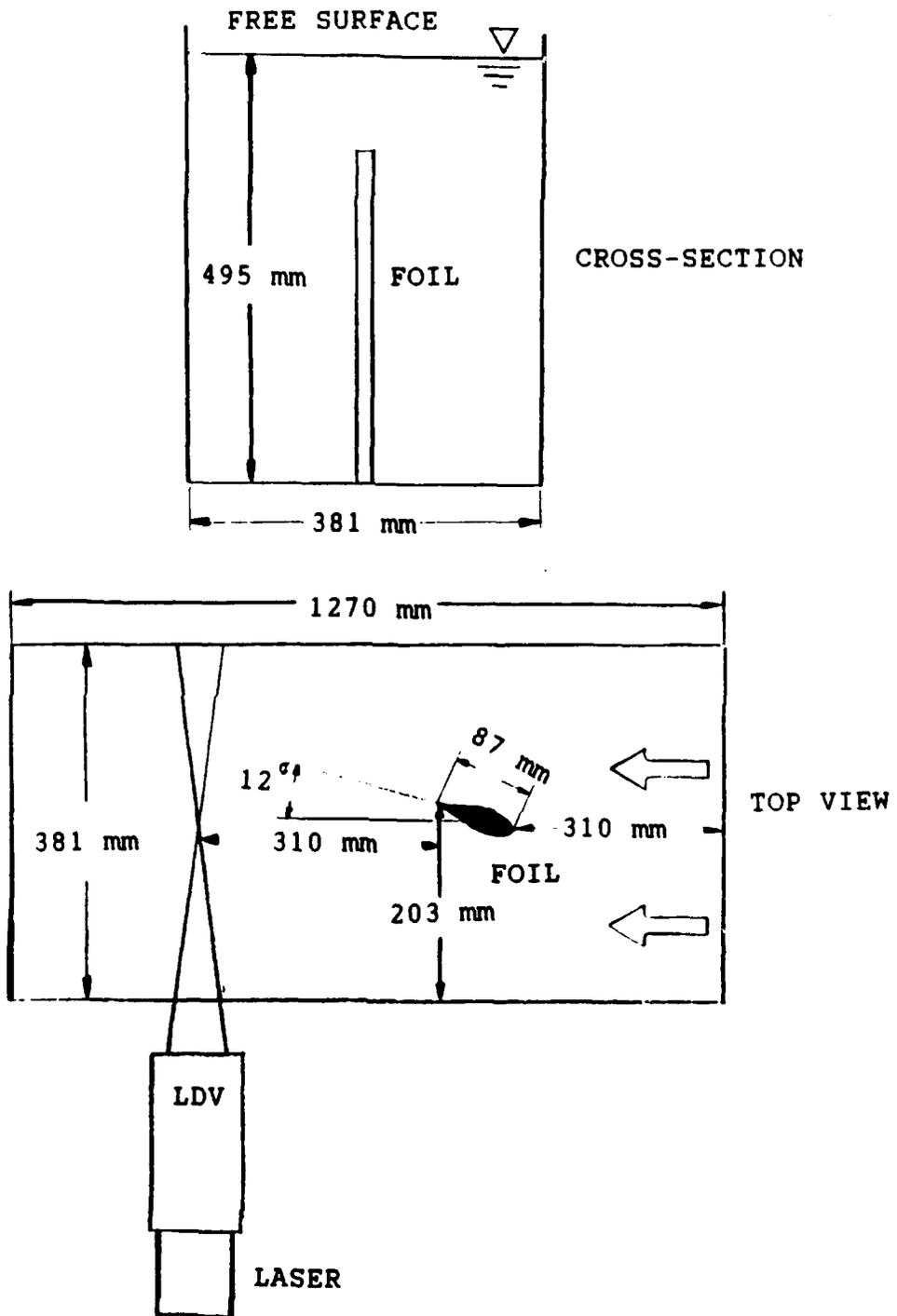
Figure 2. Schematic Drawing of the Test Section
