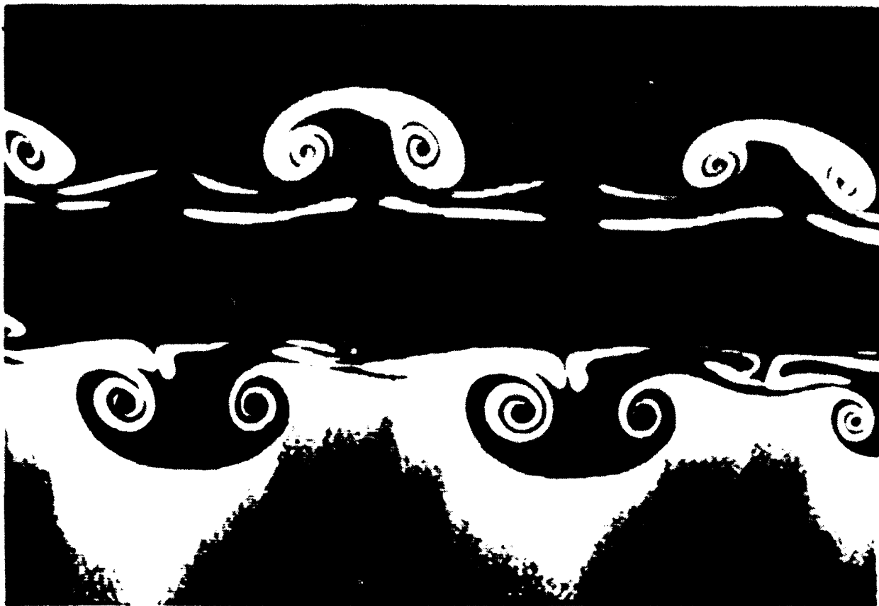
Fig 1a. Fluorescence dye visualization of streamwise ( in the flow direction) vortices which wind themselves around the Kelvin-Helmholtz billows. Unstratified case ( Ri=0.0 )
