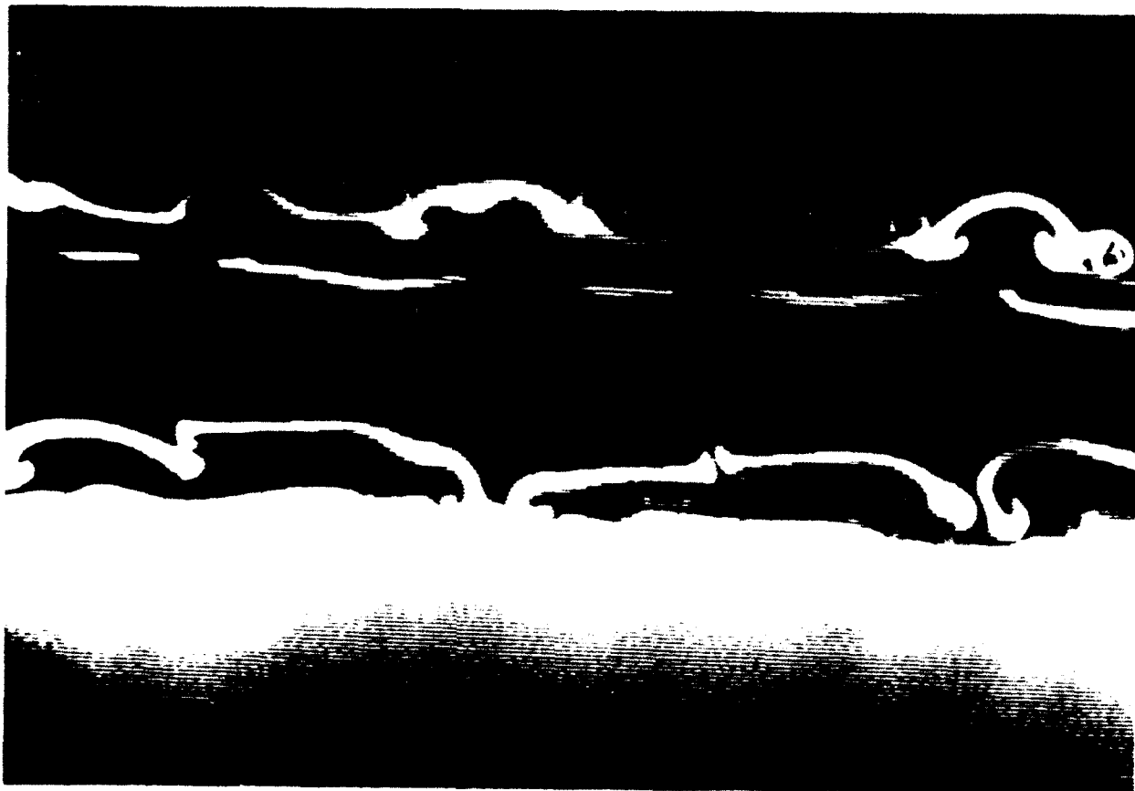
Fig 1b. Same as 1a except now Ri=0.04 . Note how streamwise vortices are compressed in the vertical direction compared with 1a.
