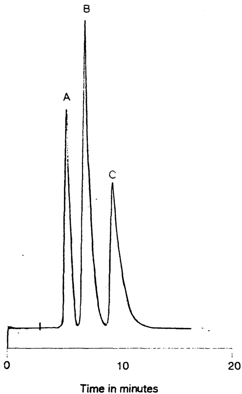
**Figure 4.** Normal-phase liquid chromatographic separation of basic compounds. Peaks: A = 2,4,6-trimethylaniline; B = 1-aminonaphthalene; C = 2-aminoanthracene. Column: 250 x 4.6 mm phosphorylated silica; mobile phase: 97% cyclohexane/3% 2-propanol; flow rate: 1 mL/min; detection: UV @ 254 nm.
