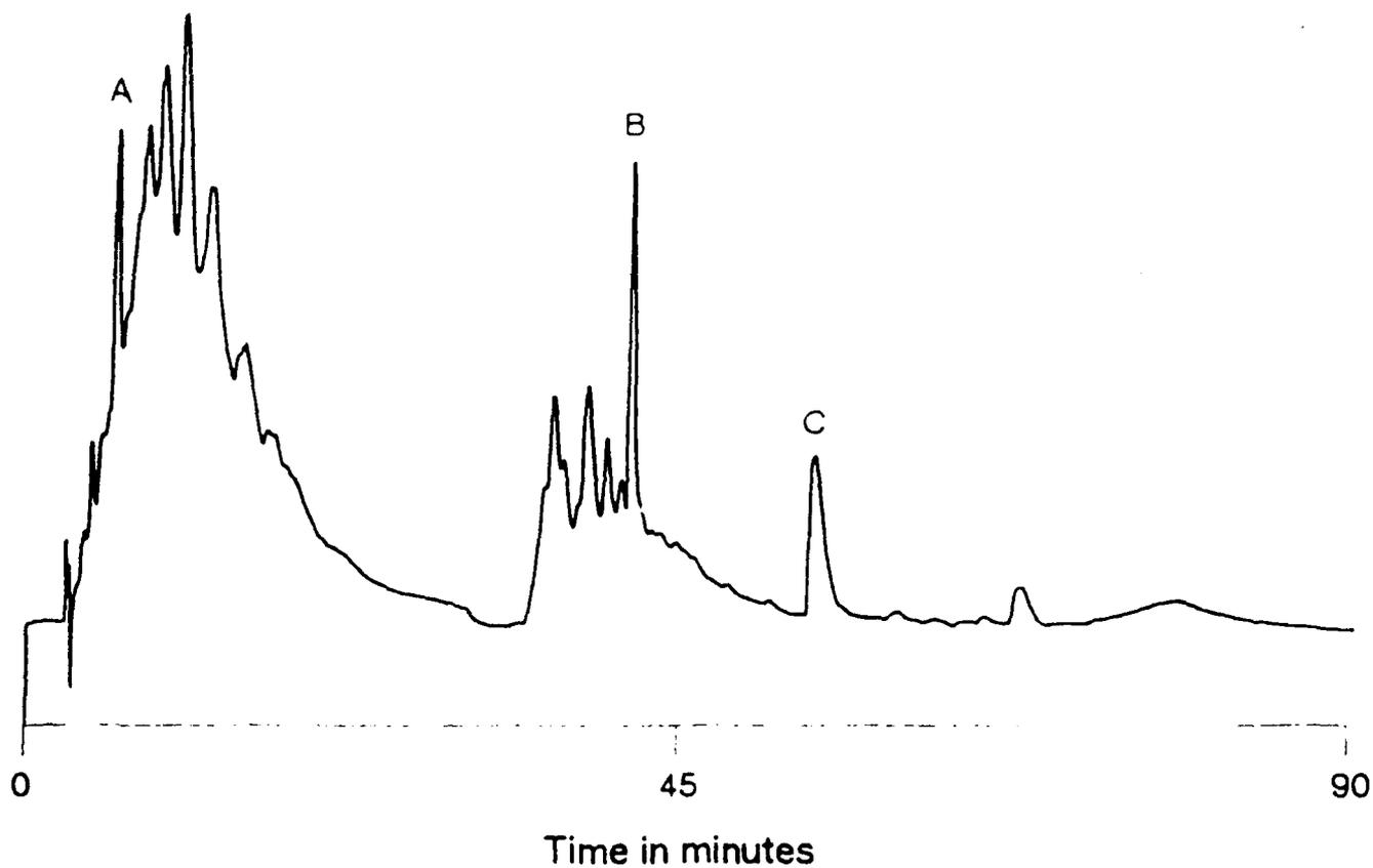
**Figure 3.** Normal-phase liquid chromatographic class fractionation of OLMECA crude oil spiked with naphthalene, carbazole, and 3-aminofluoranthene. Peaks: A = naphthalene; B = carbazole; C = 3-aminofluoranthene. Column: 250 x 4.6 mm phosphorylated silica; mobile phase: 100% cyclohexane from 0 min to 30 min, ramp to 40% cyclohexane/60% methylene chloride from 30 min to 60 min; flow rate: 1 mL/min from 0 min to 30 min, 2 mL/min from 30 min to 60 min; detection: UV @ 254 nm.
