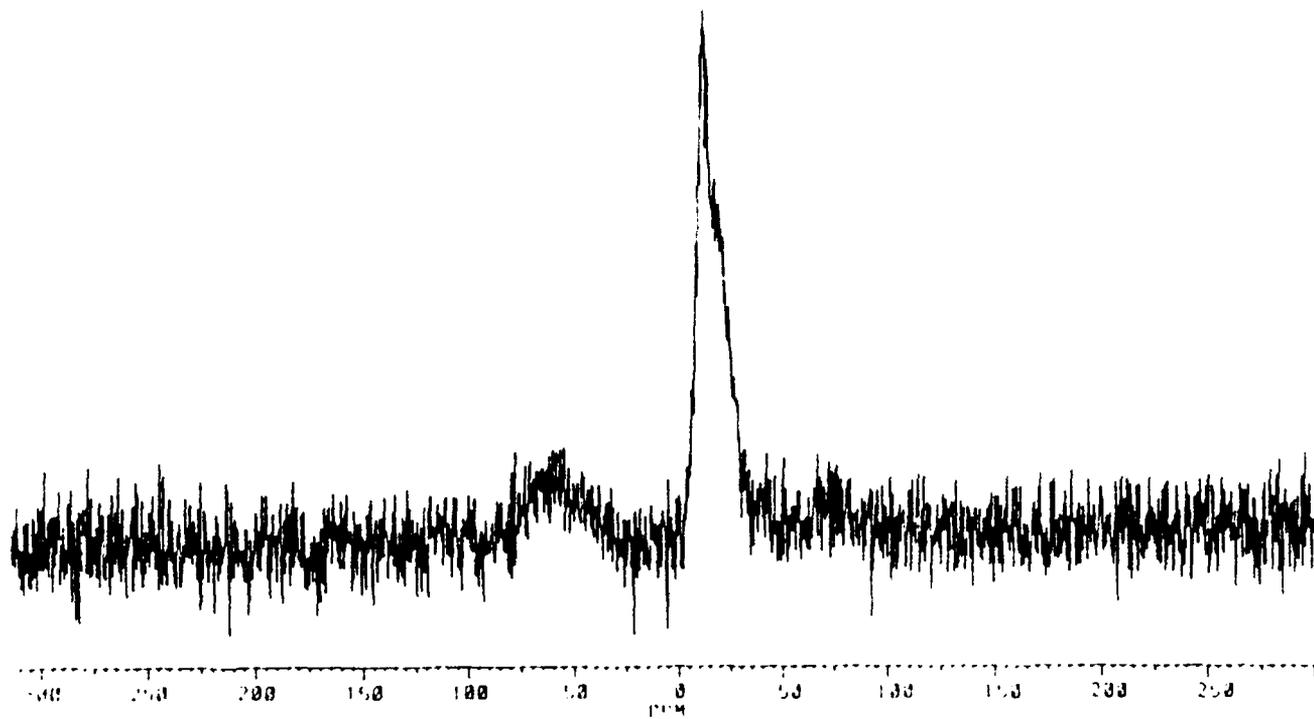
Figure 6. CP-MAS  $^{31}\text{P}$  NMR of Phosphorylated Zeolite Y.
