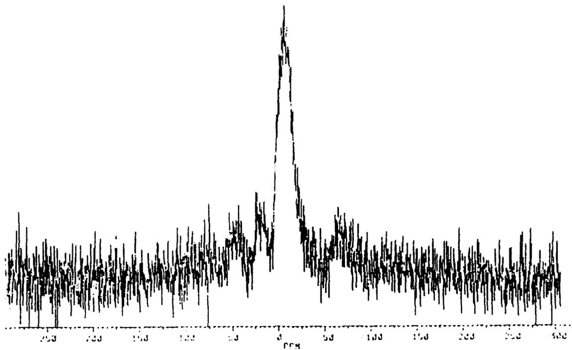
Figure 8. CP-MAS  $^{31}\text{P}$  NMR of Phosphorylated Alumina.
