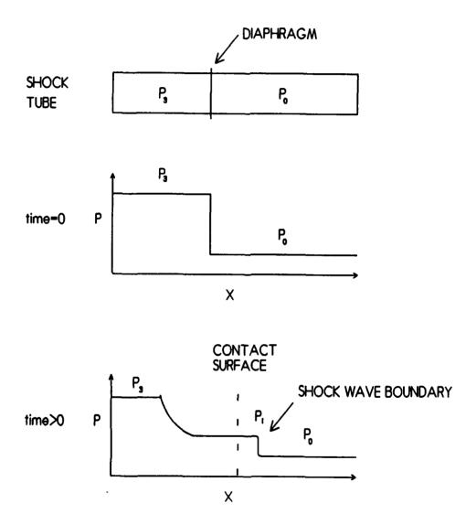
Figure 1. Illustration of Shock Tube Pressure Profiles before (time = 0) and after (time > 0) the Rupture of the Diaphragm.
