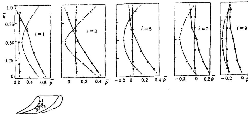
Fig. 5 Distribution along the blade height of static pressure coefficient of blade surface. i) straight blade, ii) inclined blade, iii) curved blade.
