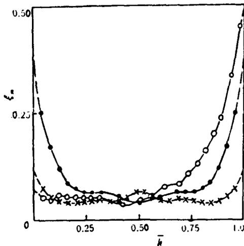
Fig. 2 Distribution along the blade height of the gap average of the energy loss coefficient. i). straight blade, ii). linear inclined blade, iii). curved blade ( $s=20^\circ$ ).
