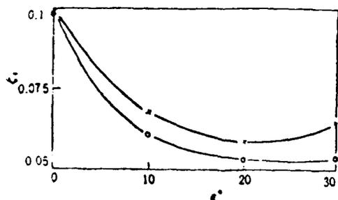
Fig. 7 Variation of total loss coefficient as a function of inclination angle. i) linear inclined blade, ii) curved blade.
