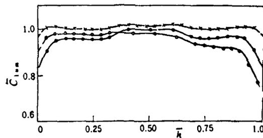
Fig. 10 Distribution along the blade height of the tangential velocity coefficient averaged along the gap.
