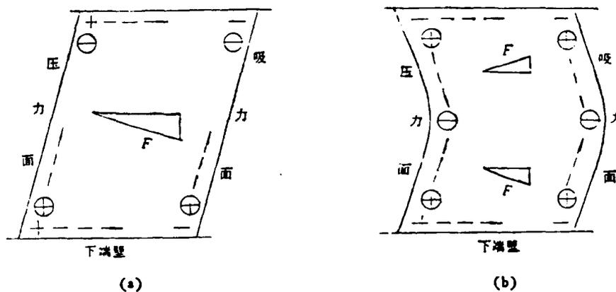
Fig. 4 Schematic diagram of pressure gradient formation along blade height. +, - indicate static pressure field formed by horizontal force component, arrow points to lower pressure from higher pressure.  $\oplus$ ,  $\ominus$  indicate static pressure field formed by vertical force component, the directions of arrows are the same. i). upper side wall, ii). lower side wall, iii) pressure side, iv) suction side.
