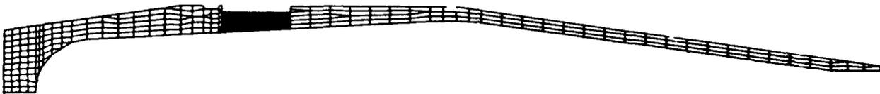
Figure 7. Plastic Zone in the Projectile at Maximum Rotating Band Pressure
