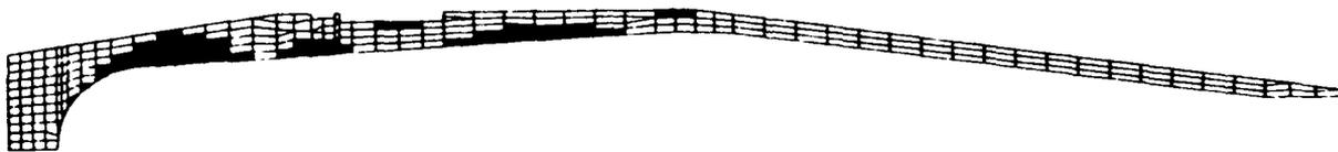
Figure 10. Plastic Zone in the Projectile at Maximum Propellant Gas Pressure and Maximum Setback Force
