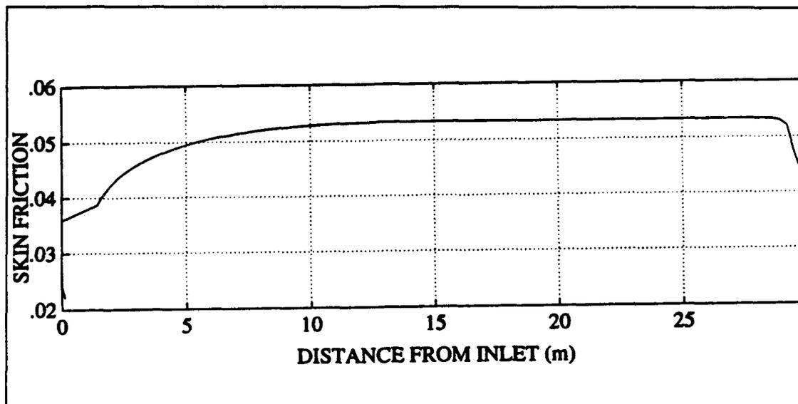
**Figure 4** - Skin Friction Coefficient for the bottom Wall of a Square Duct
