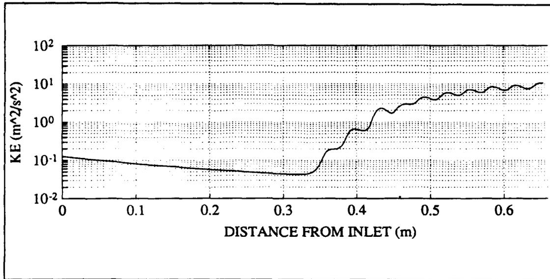
**Figure 17** - Turbulent Kinetic Energy for the Shortened Duct
