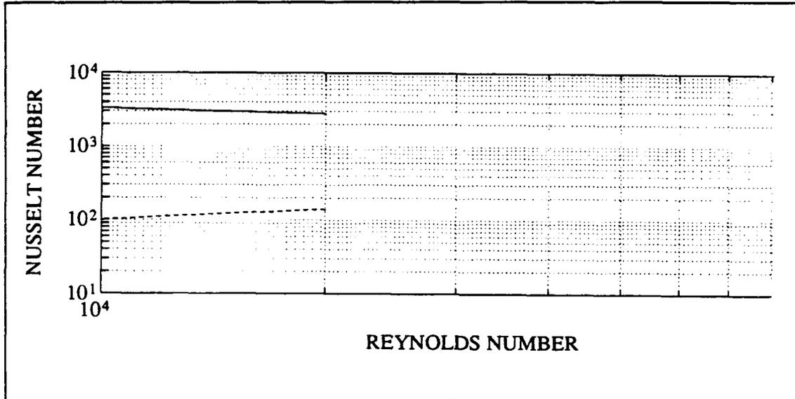
**Figure 33** - Nusselt Number vs Reynolds Number Using a Grid Stretching Value of 1.05
