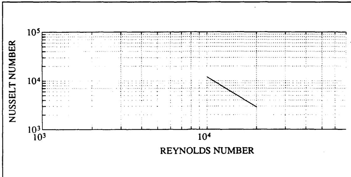
**Figure 31** - Nusselt Number vs Reynolds Number Using a Grid Stretching Factor of 1.10
