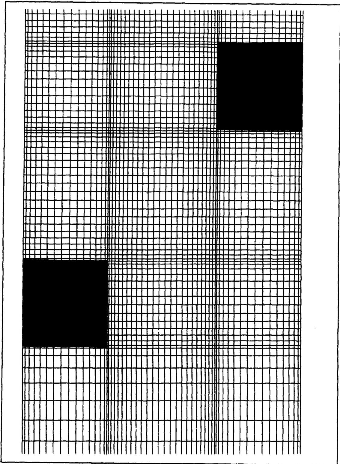
Figure 2 - Grid Using a 1.20 Stretching Factor
