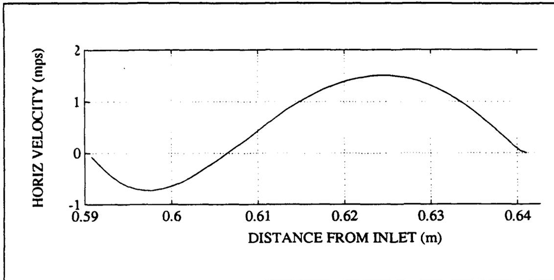
**Figure 18** - Horizontal Velocity Component Between Turbulators 8 and 10 Using a 1.20 Stretching Factor
