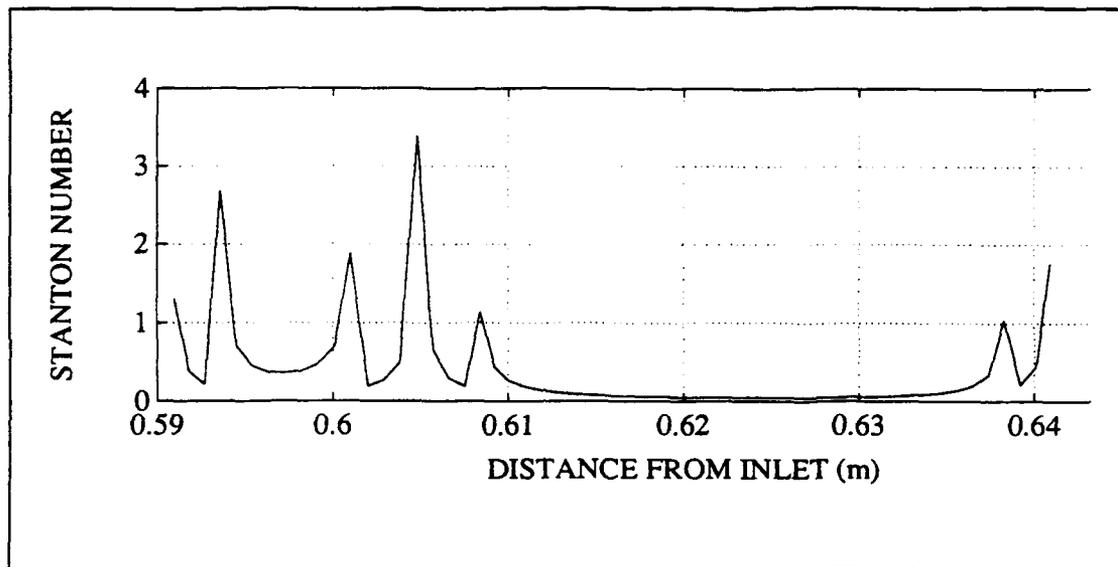
**Figure 23** - Stanton Number Between Turbulators 8 and 10 Using a 1.05 Stretching Factor
