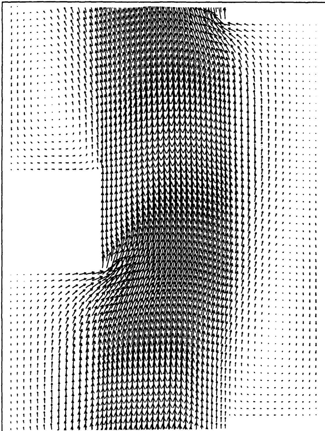
**Figure 11** - Velocity Vectors Between Turbulators 2 and 4
