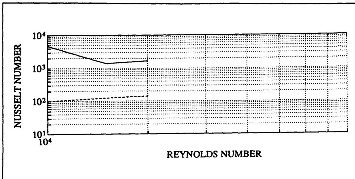
**Figure 30** - Nusselt Number vs Reynolds Number for a Uniformly Spaced Grid
