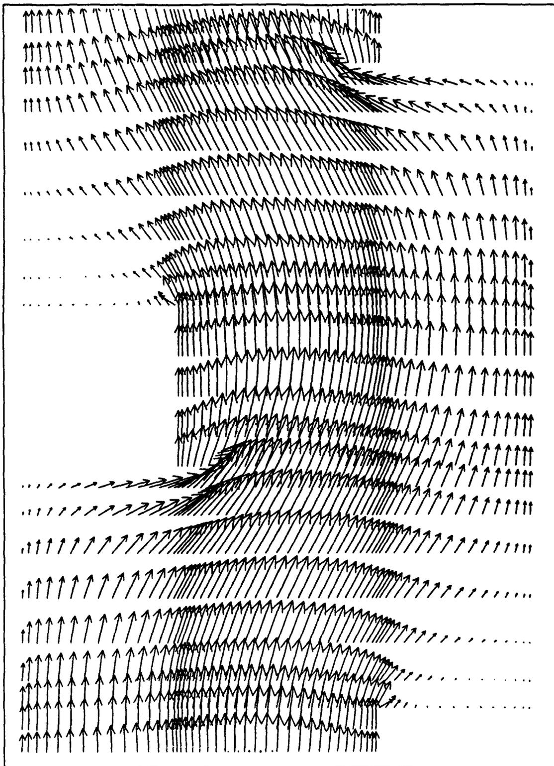
**Figure 7** - Velocity Vectors Between Turbulators 8 and 10
