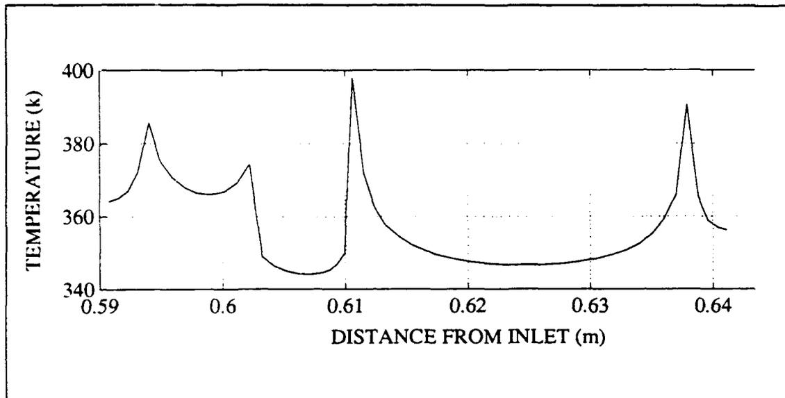
**Figure 21** - Temperature Between Turbulators 8 and 9 Using a 1.20 Stretching Factor
