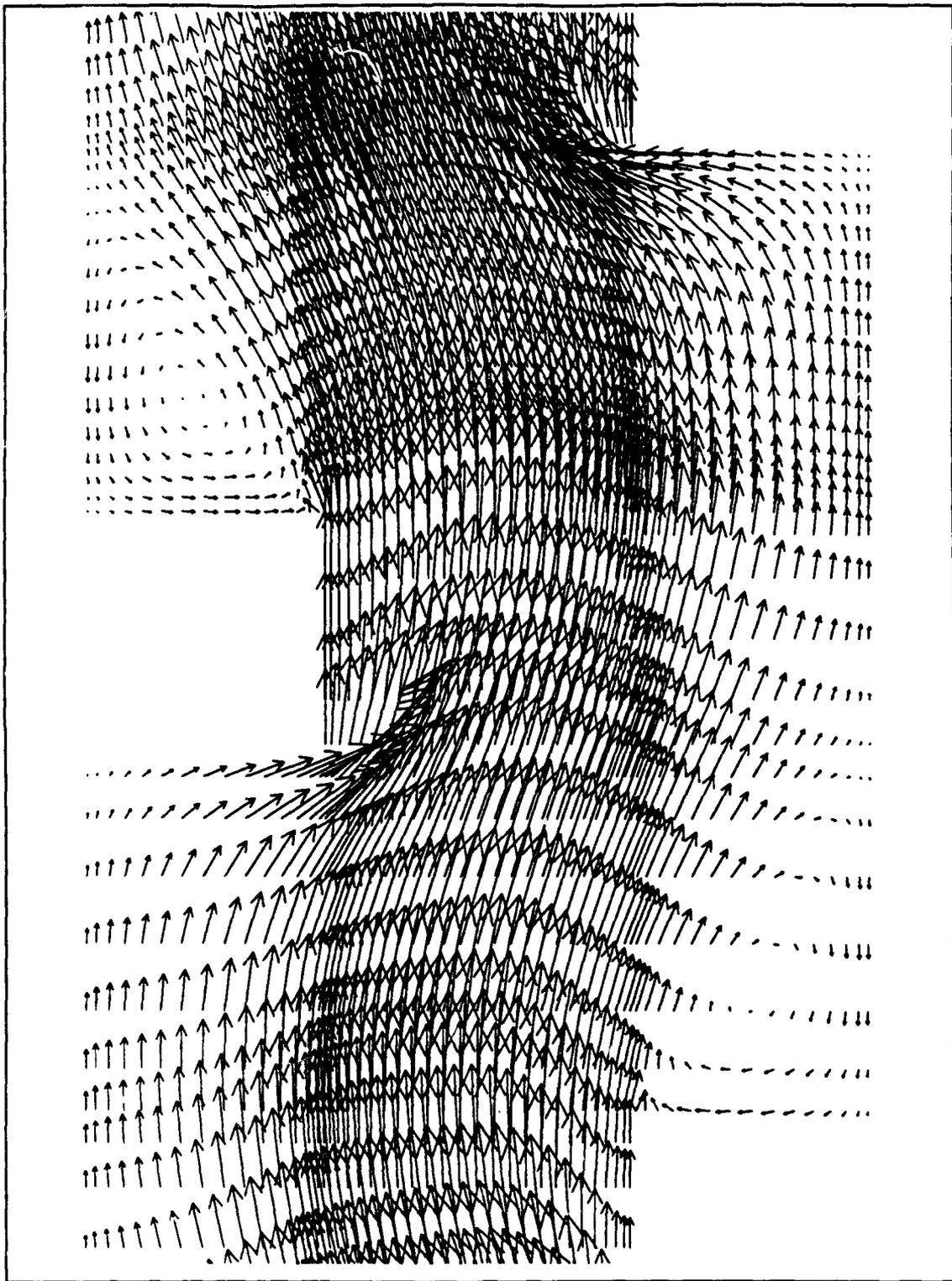
**Figure 6** - Velocity Vectors Between Turbulators 2 and 4
