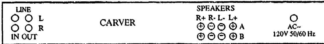
Figure 17 Carver Power Amplifier (Rear Panel)
