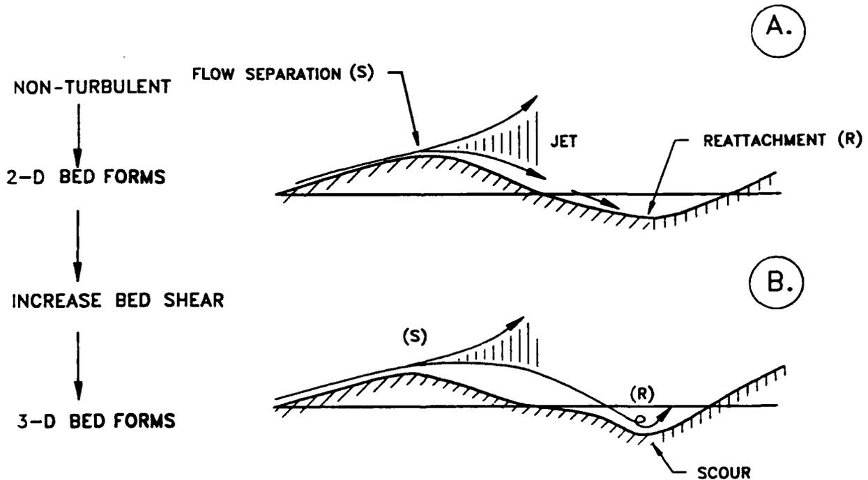
Figure 6. Jet current behavior over the brink of a ripple. In A, at low velocity, the current streamlines hug the bed form near the crest. In B, the flow jet separates at the brink of the bed form and reattaches at a point of scour in the downstream trough.
