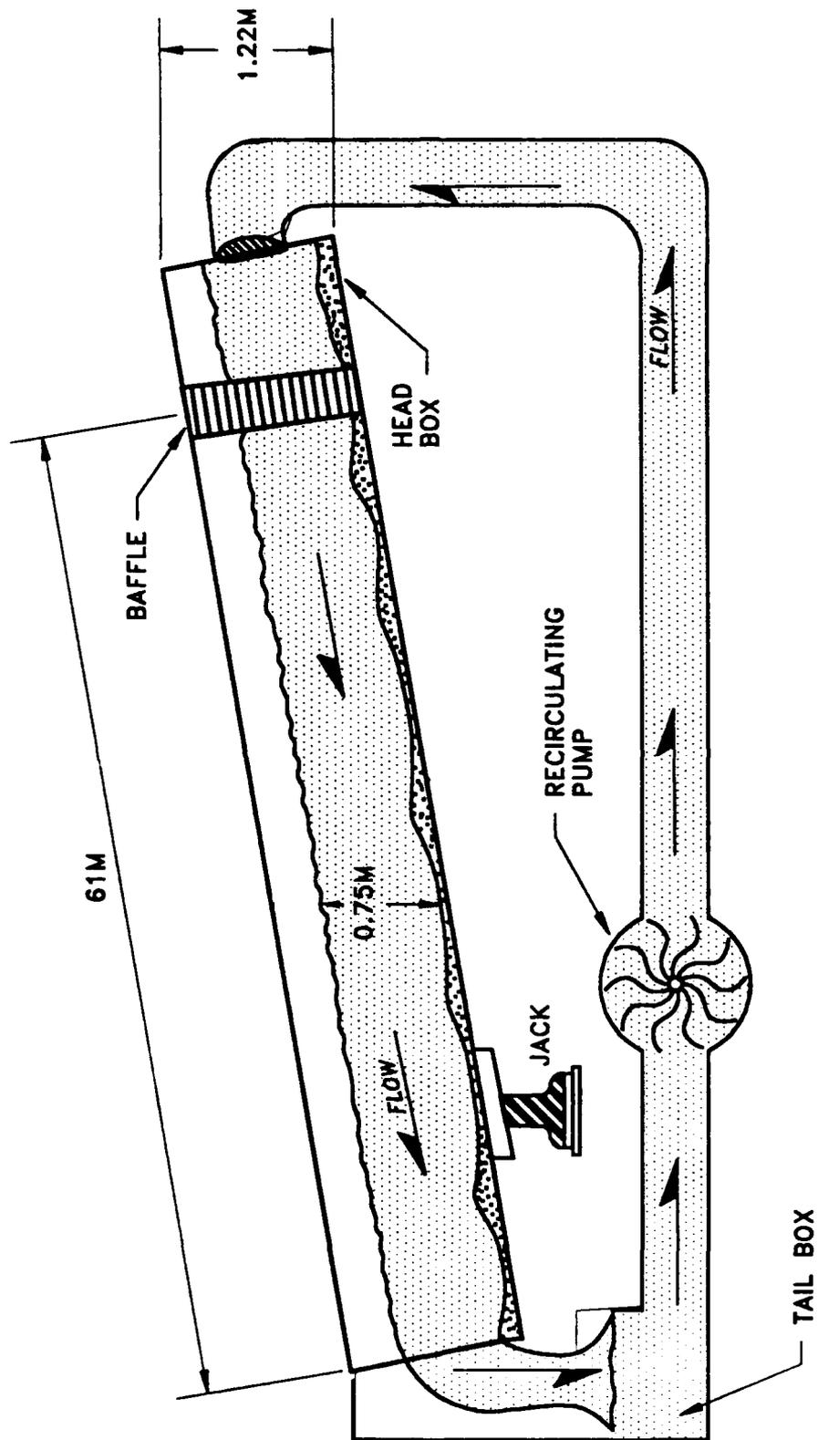
Figure 3. Flume diagram (modified from Harms 1969)
