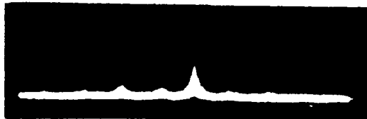
(3) bi-directional resonance with 2 m path imbalance
