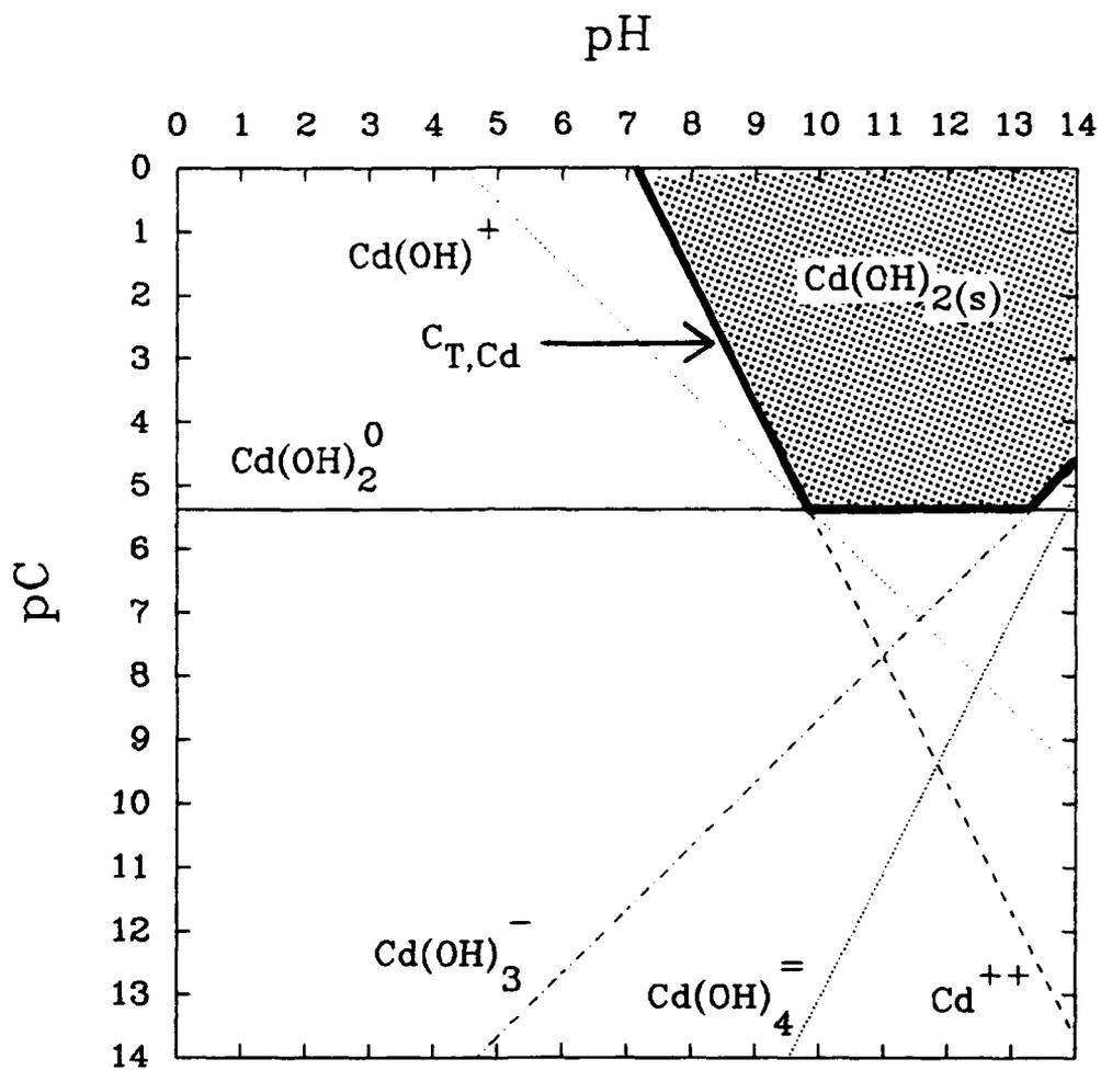
Figure 2-1. Solubility of total cadmium(II)  $C_{T,Cd}$  in water versus pH at 25°C.
