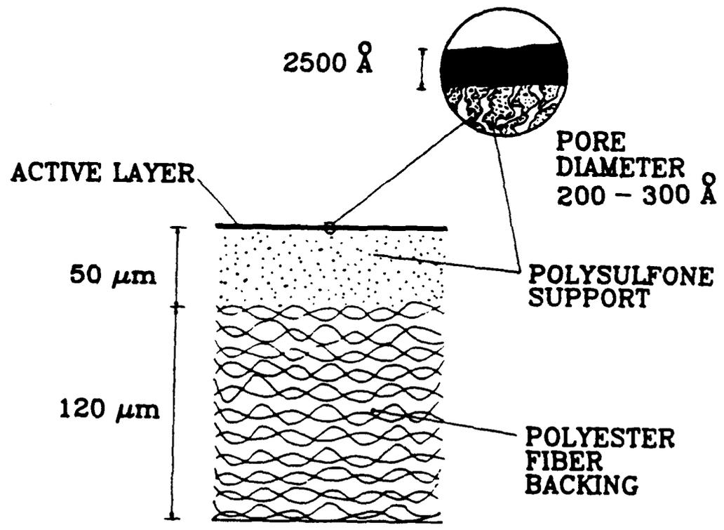
Figure 3-1. Schematic of thin-film composite FT-30 membrane.
