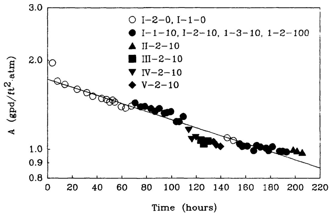
Figure 4-2. Effect of membrane compaction on  $A_{25}$ .
