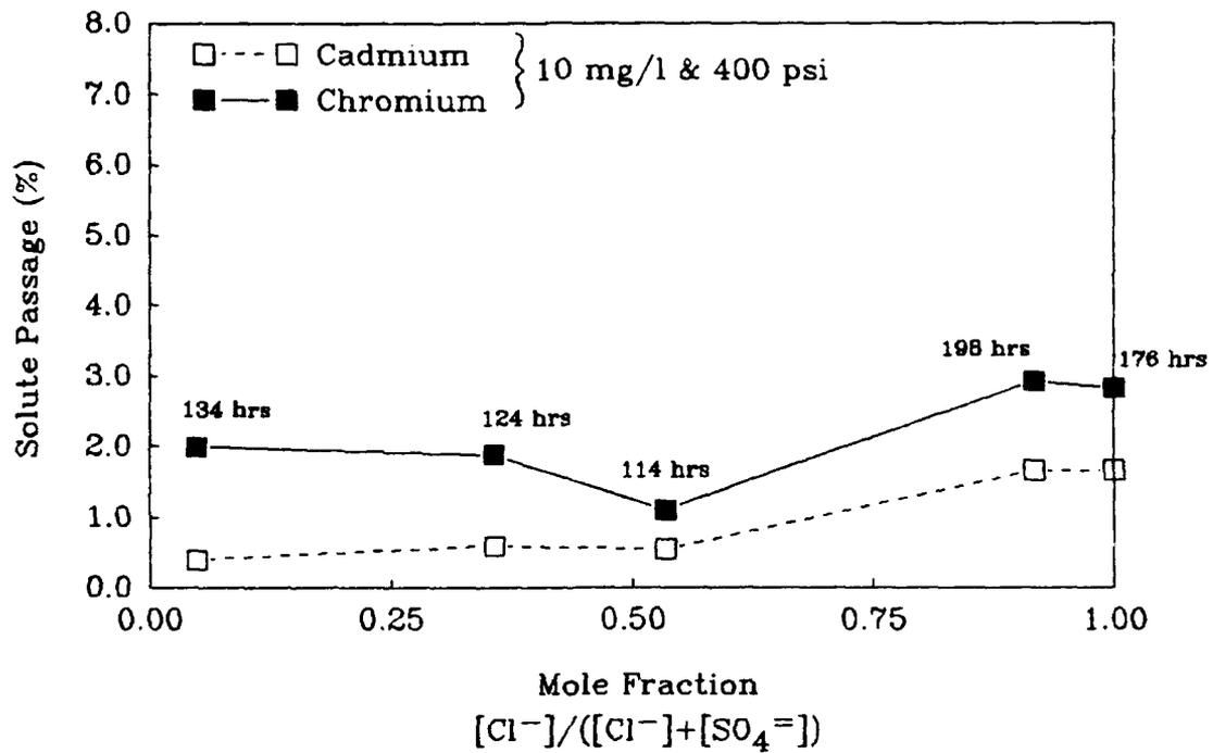
Figure 4-15. Observed solute passages for cadmium (II) and chromium (VI) corresponding to tests performed with feed solutions I-2-10, II-2-10, III-2-10, IV-2-10, and V-2-10 performed at the operating times indicated.
