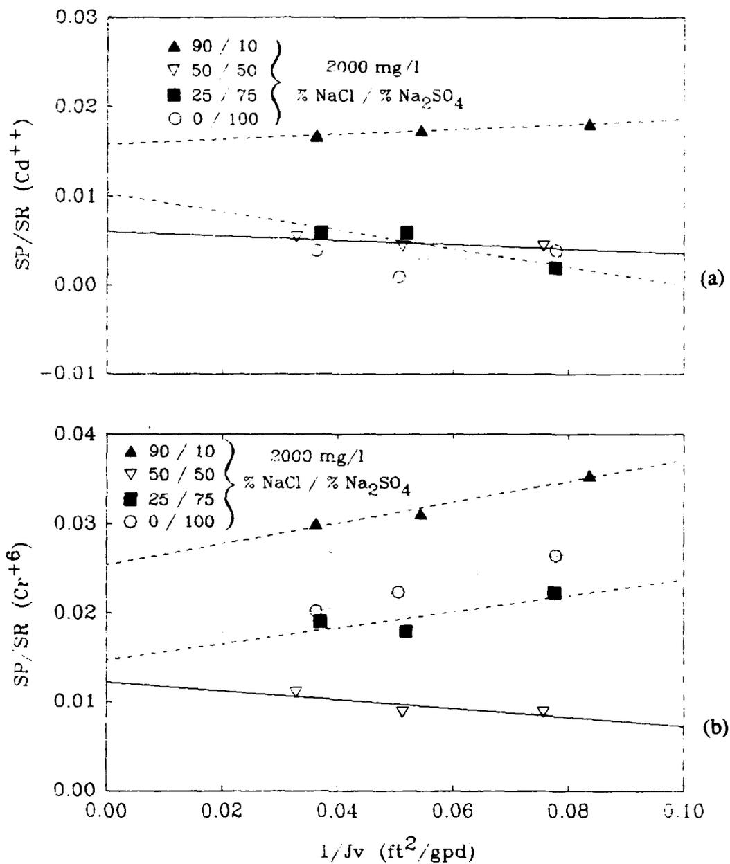
Figure 4-17. Linear plot of cadmium (II) (a) and chromium (VI) (b) permeation data corresponding to tests performed with feed solutions II-2-10, III-2-10, IV-2-10 and V-2-10, respectively.
