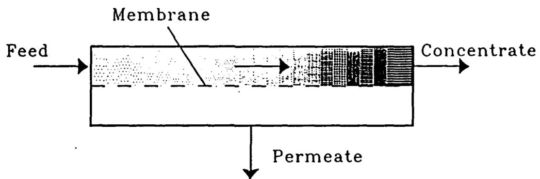
Figure 2-3. Schematic of RO unit.
