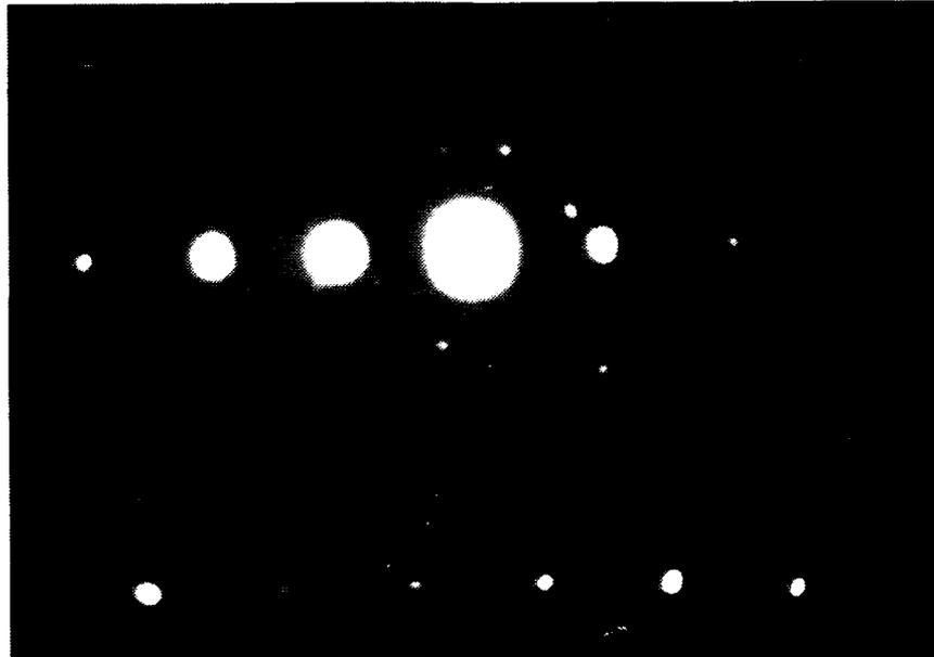
Figure 18. Diffraction Pattern Showing a [133] Crystallographic Zone Axis
