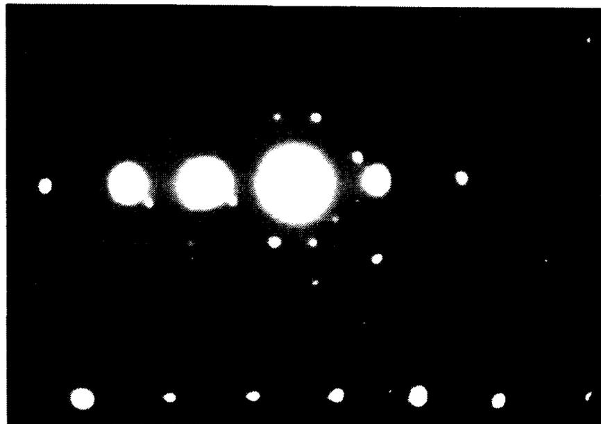
Figure 19. Diffraction Pattern Showing a [133] Crystallographic Zone Axis
