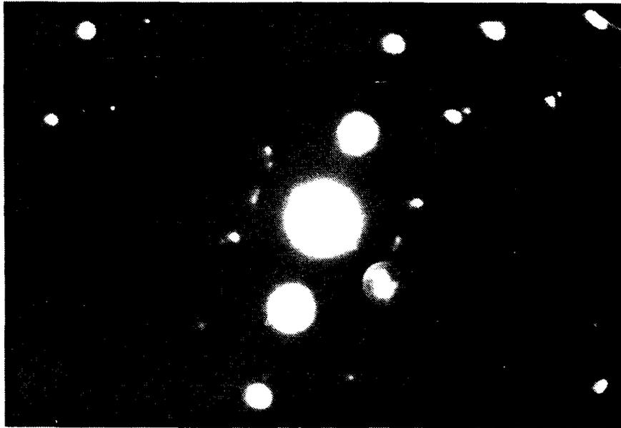
Figure 32. Diffraction Pattern of [111] Pole Showing Evidence of  $(FeM)_3C$  Type Carbide
