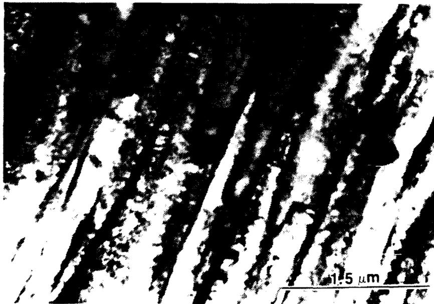
Figure 15. TEM Image Showing Lath Martensite and Retained Austenite at Lath Boundaries
