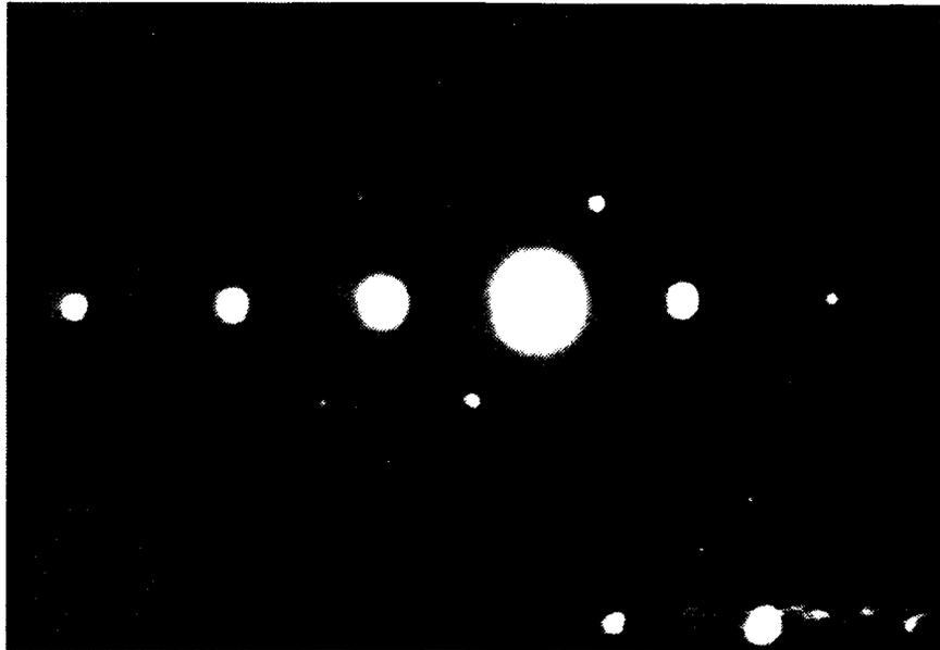
Figure 24. Diffraction Pattern Showing a [133] Crystallographic Zone Axis
