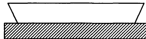
6. Subsequent homoepitaxy to duplicate the large area template.
