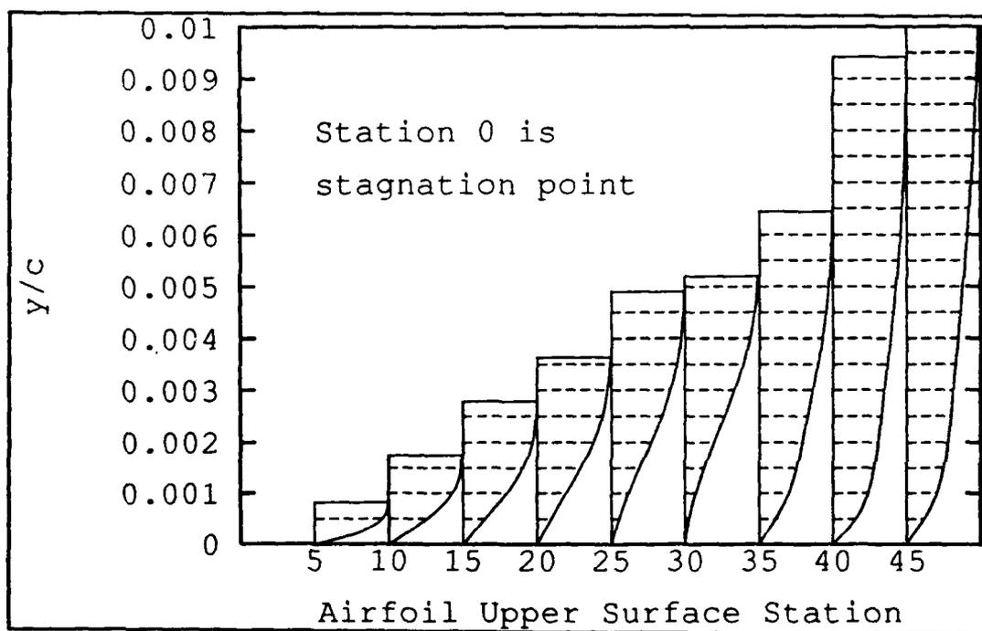
**Figure 3.11 BL2D: Velocity Profiles, NACA 0012, AOA=0°, Re=540,000**
