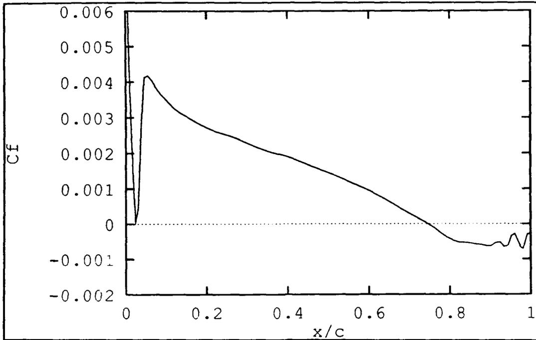
**Figure 4.13 INCOMPBL:  $C_f$ , NACA 0012, AOA= $13.4^\circ$ , Re=540,000**
