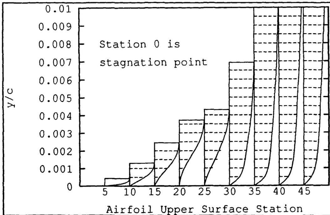
**Figure 3.13 BL2D: Velocity Profiles, NACA 0012, AOA=4°, Re=540,000**
