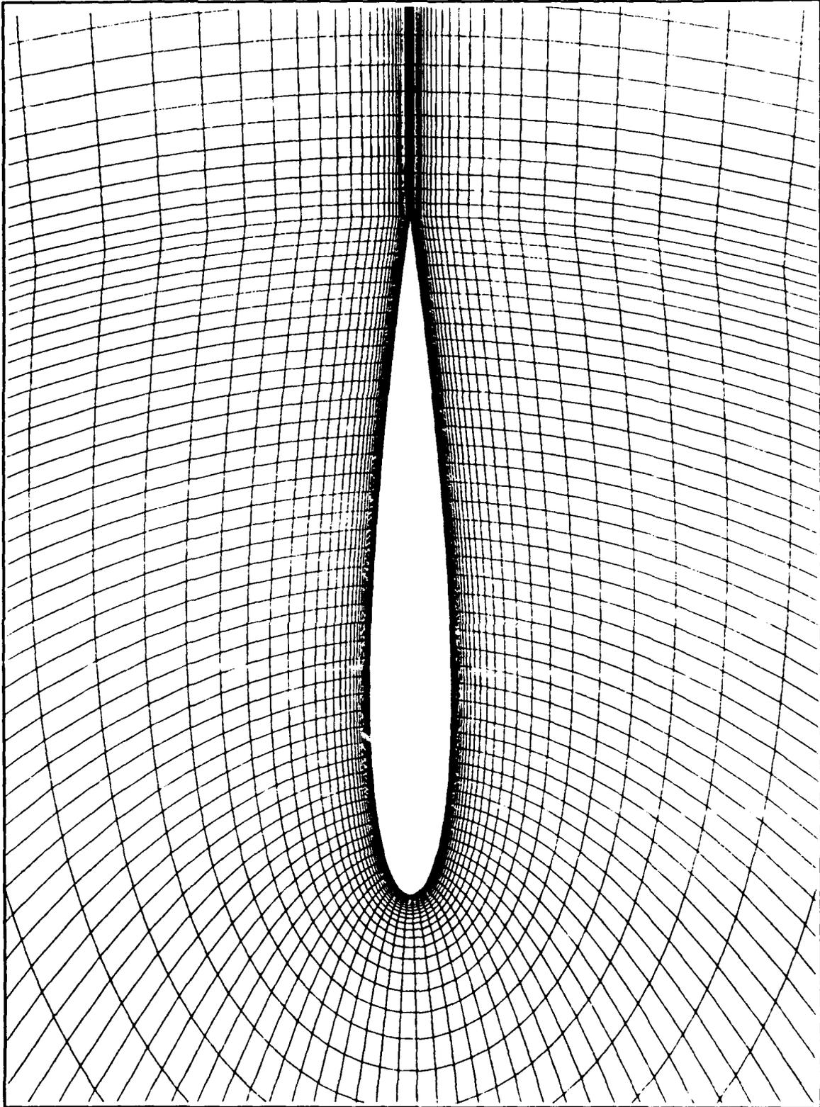
**Figure 6.1 161x64 Viscous Grid for NACA 0012 Airfoil**
