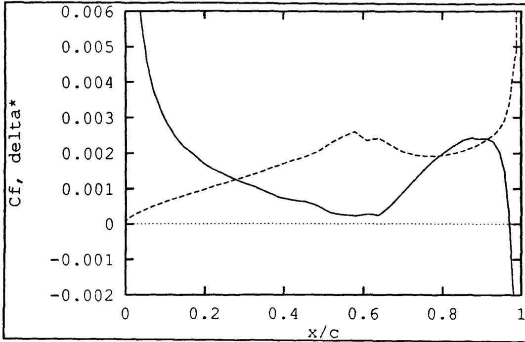
Figure 3.4 BL2D:  $C_f$  and  $\delta^*$ , NACA 0012, AOA= $0^\circ$ , Re=540,000
