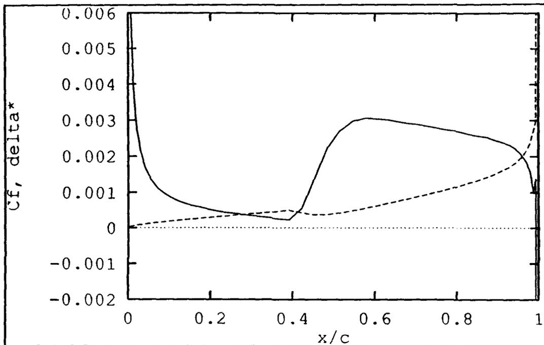
Figure 3.2 Computed  $C_f$  and  $\delta^*$ , NACA 0012, AOA=0°, Re=6,000,000
