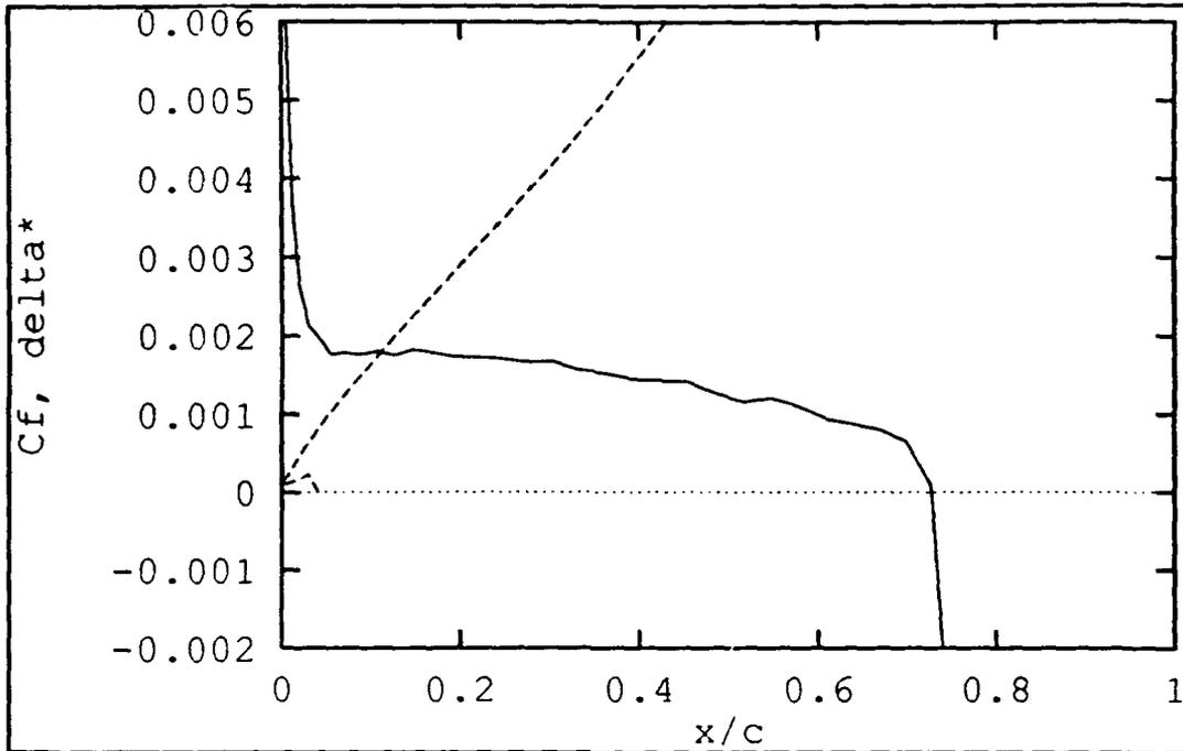
Figure 3.10 BL2D:  $C_f$  and  $\delta^*$ , NACA 0012, AOA =  $12^\circ$ ,  $Re = 540,000$
