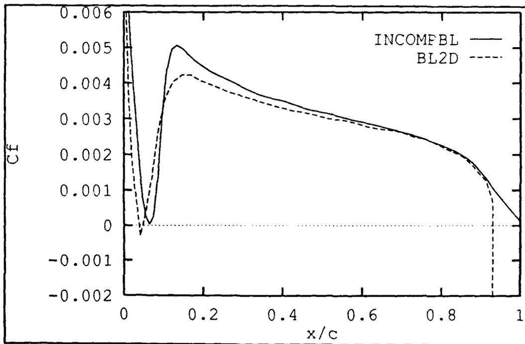
Figure 4.5  $C_f$  Comparison, NACA 0012, AOA=6°, Re=540,000
