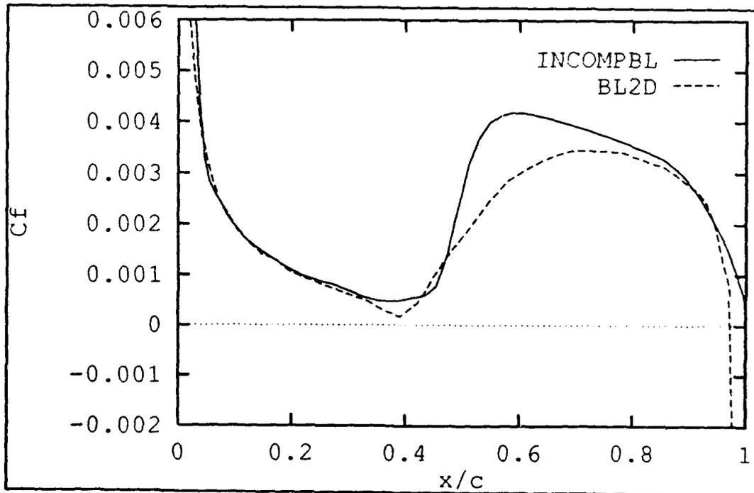
Figure 4.3  $C_f$  Comparison, NACA 0012, AOA=2°, Re=540,000
