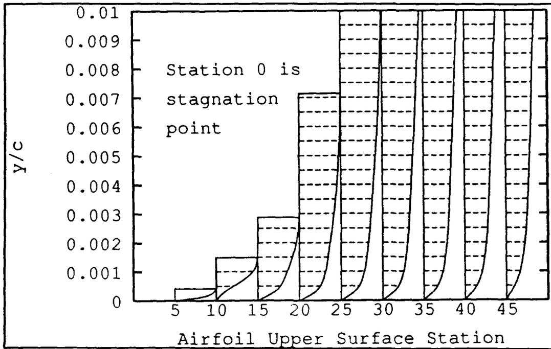
**Figure 3.14 BL2D: Velocity Profiles, NACA 0012, AOA=6°, Re=540,000**
