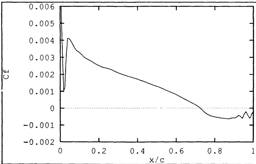
**Figure 4.14 INCOMPBL:  $C_f$ , NACA 0012, AOA= $14^\circ$ , Re=540,000**
