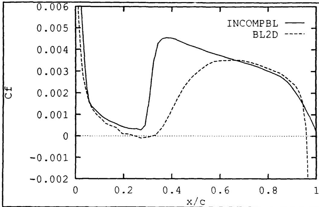
Figure 4.4  $C_f$  Comparison, NACA 0012, AOA=4°, Re=540,000
