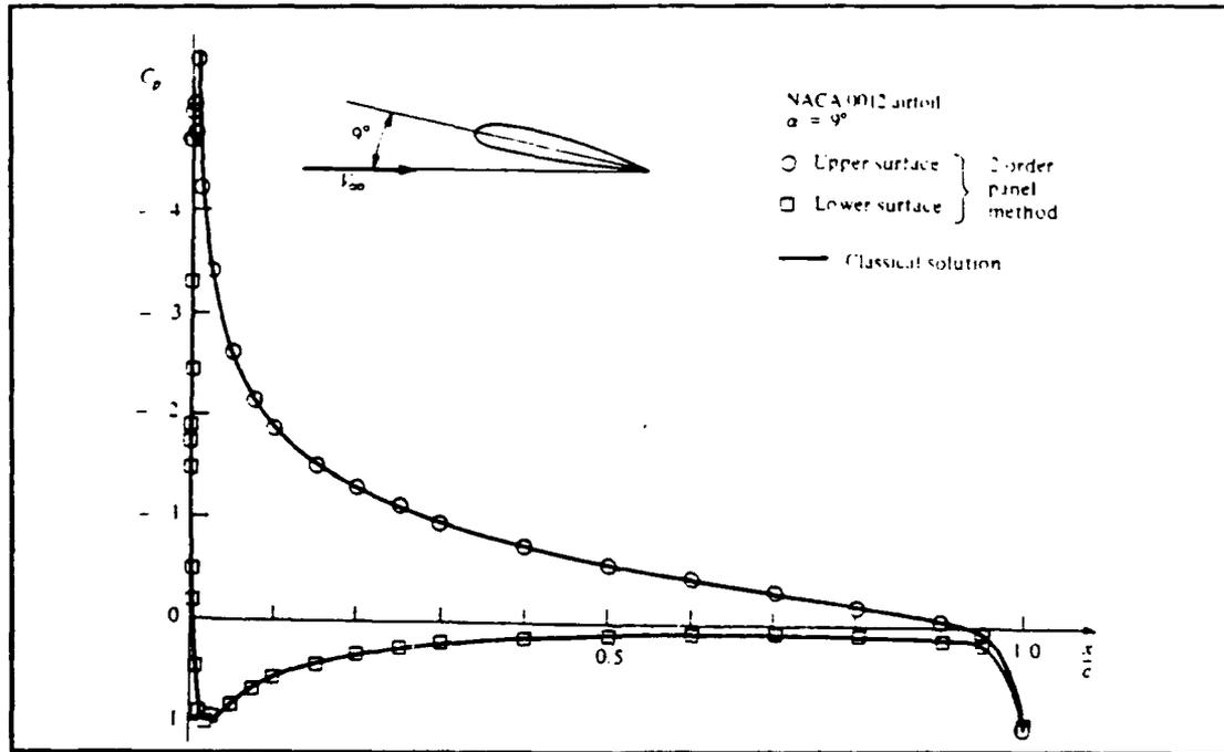
Figure 2.8 Pressure Coefficient Provided by Anderson
