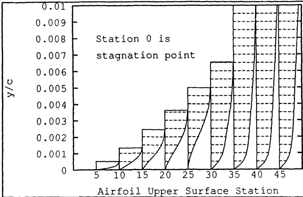
**Figure 3.12 BL2D: Velocity Profiles, NACA 0012, AOA=2°, Re=540,000**
