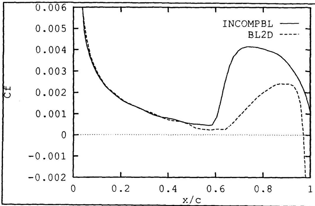
Figure 4.2  $C_f$  Comparison, NACA 0012, AOA=0°, Re=540,000
