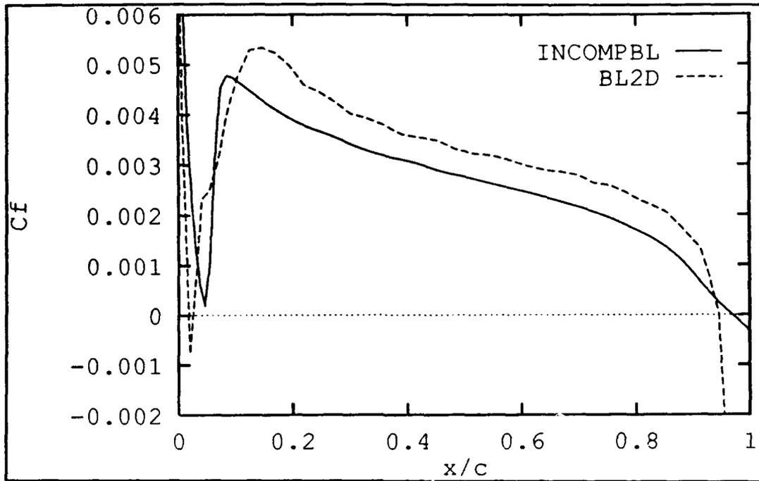
Figure 4.6  $C_f$  Comparison, NACA 0012, AOA= $8^\circ$ , Re=540,000
