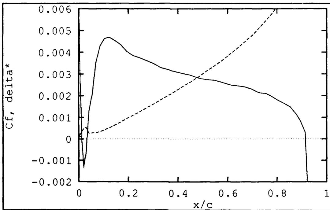
**Figure 3.9 BL2D:  $C_f$  and  $\delta^*$ , NACA 0012, AOA=10°, Re=540,000**
