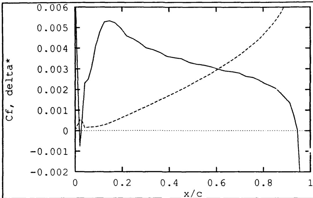
**Figure 3.8 BL2D:  $C_f$  and  $\delta^*$ , NACA 0012, AOA=8°, Re=540,000**
