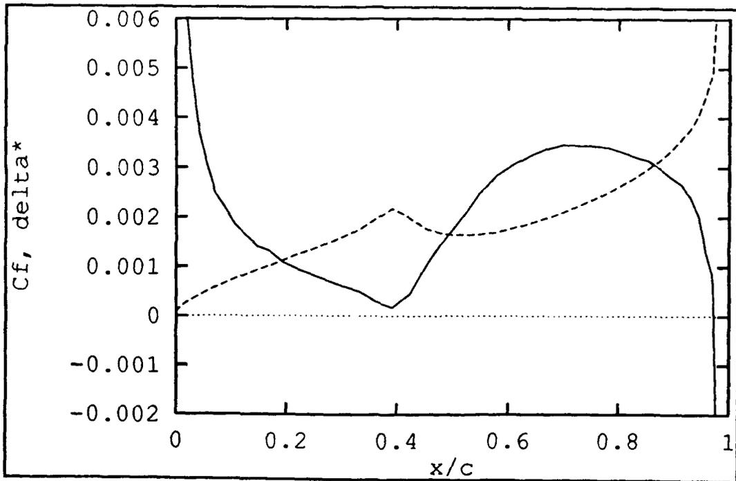
Figure 3.5 BL2D:  $C_f$  and  $\delta^*$ , NACA 0012, AOA= $2^\circ$ , Re=540,000
