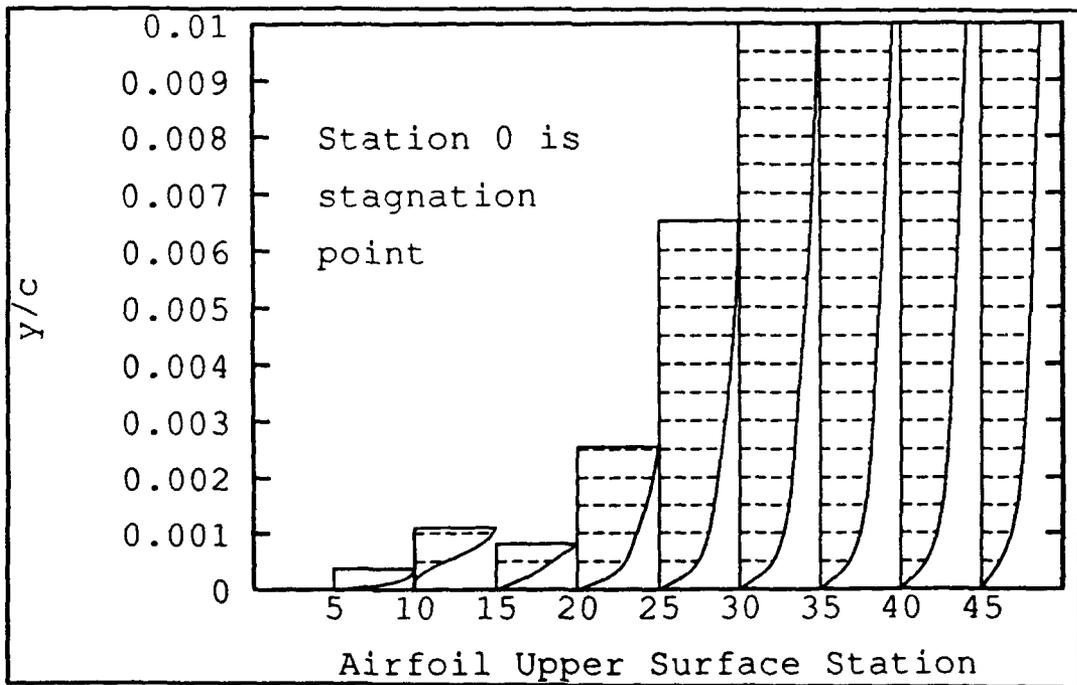
**Figure 3.15 BL2D: Velocity Profiles, NACA 0012, AOA=8°, Re=540,000**
