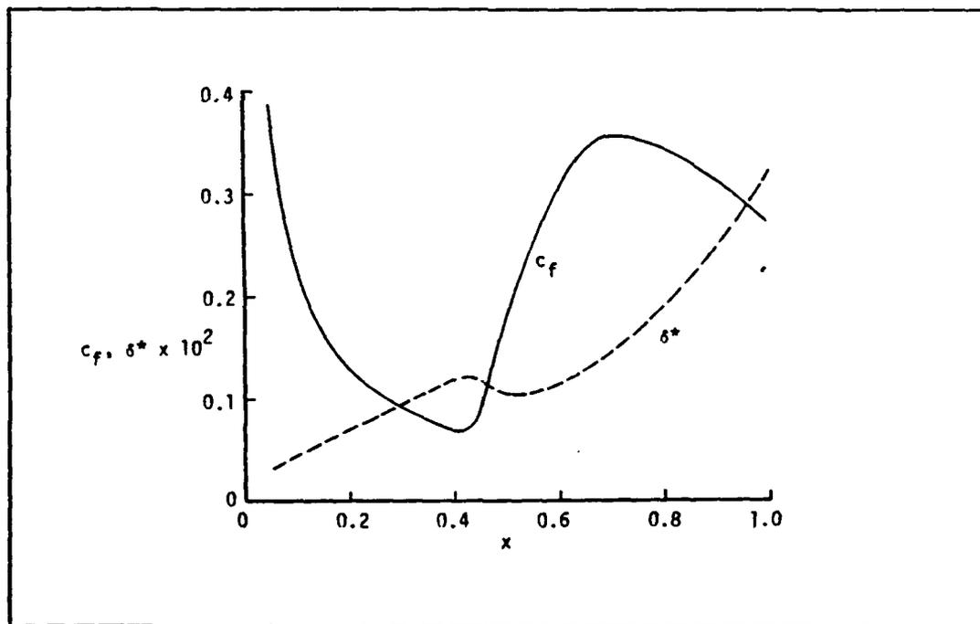
Figure 3.3 Reference  $C_f$  and  $\delta^*$ , NACA 0012, AOA=0°, Re=6,000,000
