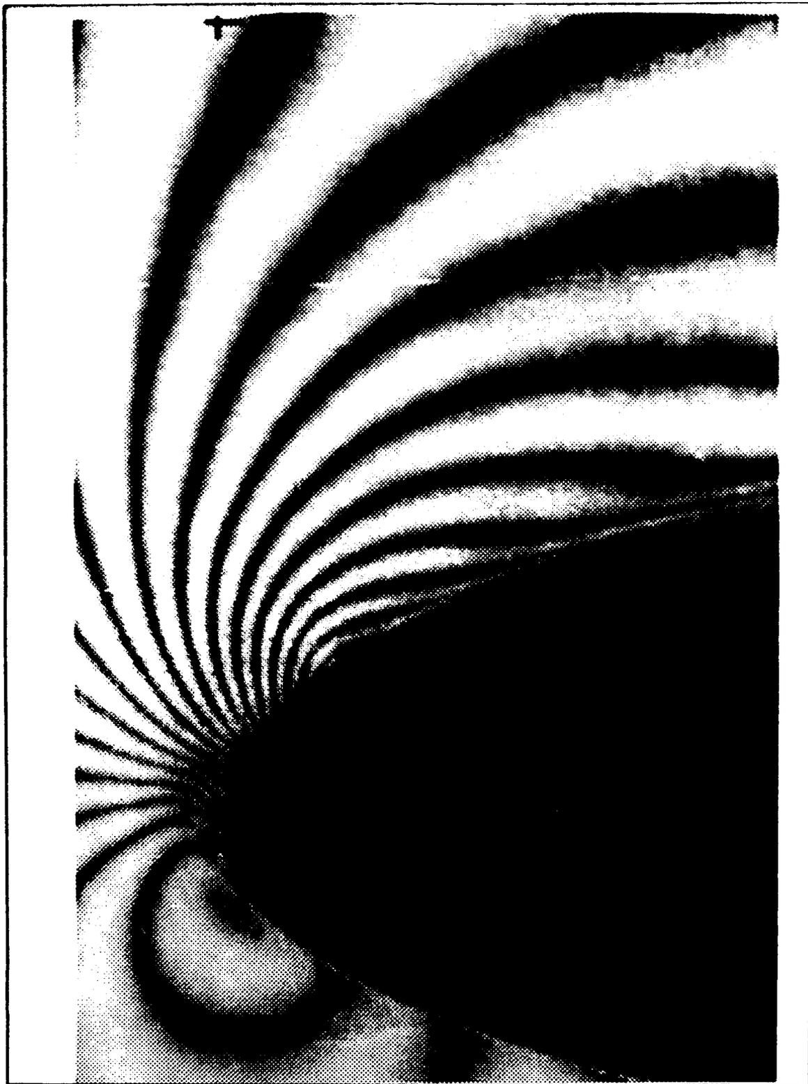
**Figure 5.4 Enlarged Leading Edge Interferogram, AOA=6°**
