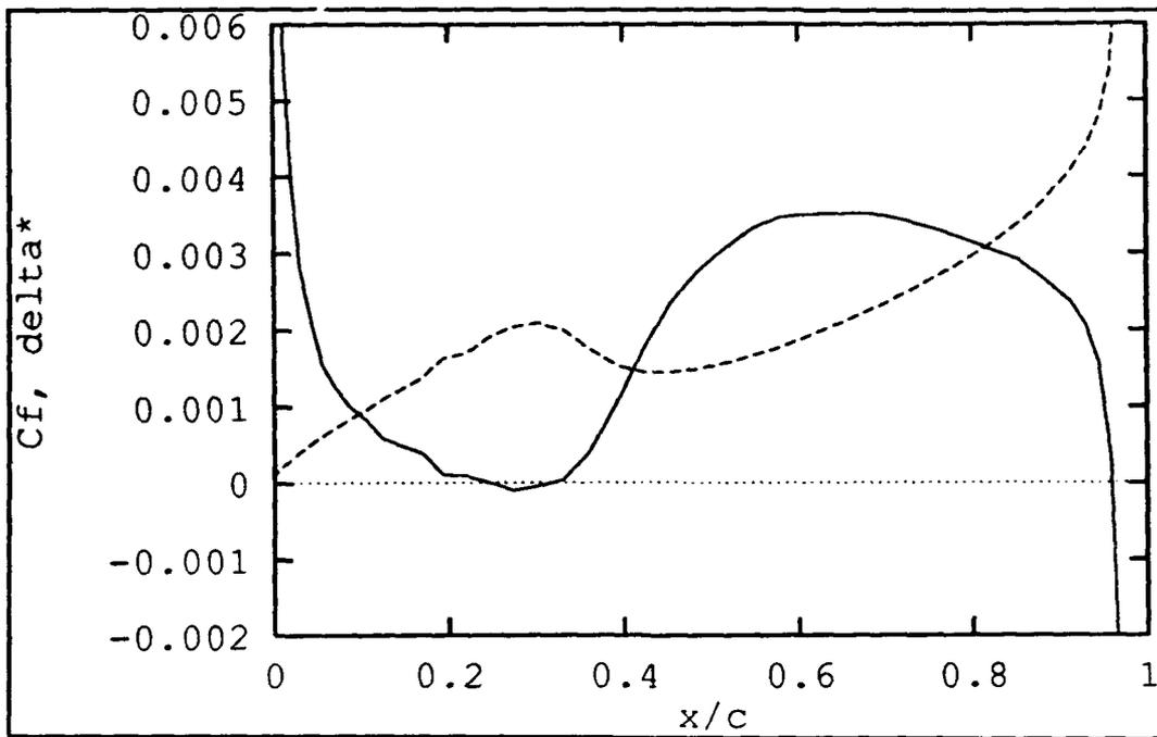
Figure 3.6 BL2D:  $C_f$  and  $\delta^*$ , NACA 0012, AOA=4°, Re=540,000
