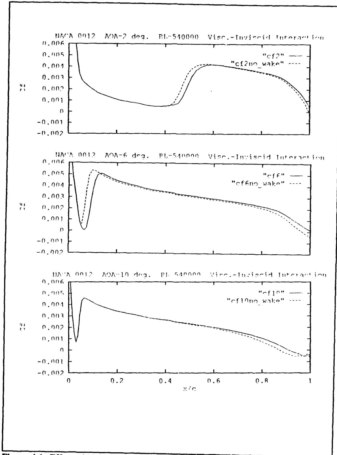
Figure 4.1 Effect of Wake Calculations
