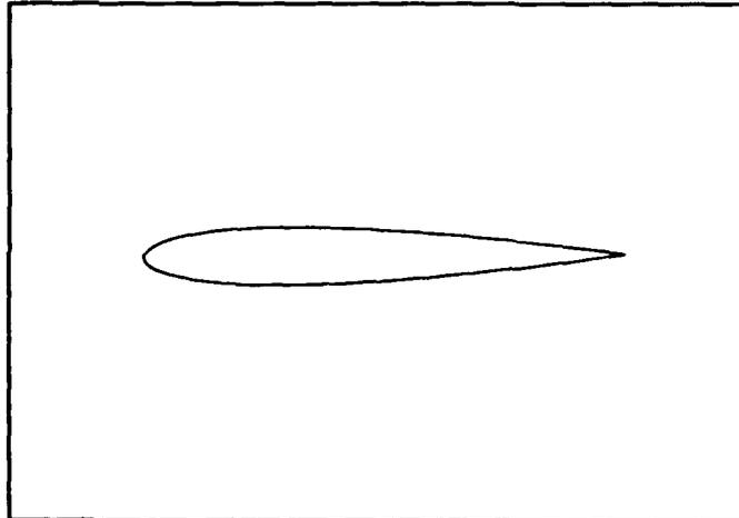
show a comparison of program **Figure 2.6 NACA 0012 Airfoil** results and those provided by Anderson [Ref. 2] for the NACA 0012 airfoil at  $9^\circ$  angle of attack. The pressure distributions both come to a suction peak of -5.2. It should be noted that Figure 2.8 differs slightly from the original reference plot in that the error in the decimal place of the ordinate values has been corrected.
