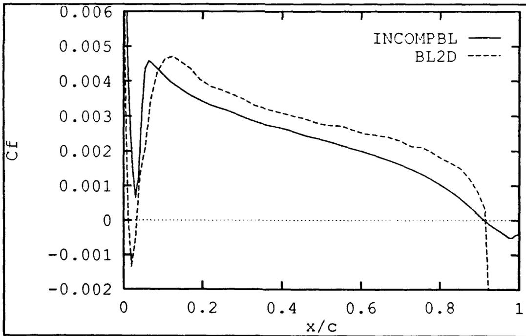
Figure 4.7  $C_f$  Comparison, NACA 0012, AOA= $10^\circ$ , Re=540,000
