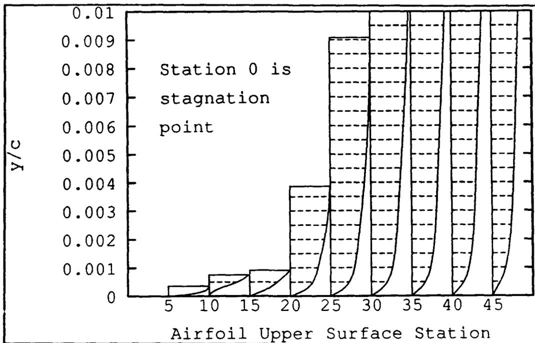
**Figure 3.16 BL2D: Velocity Profiles, NACA 0012, AOA=10°, Re=540,000**
