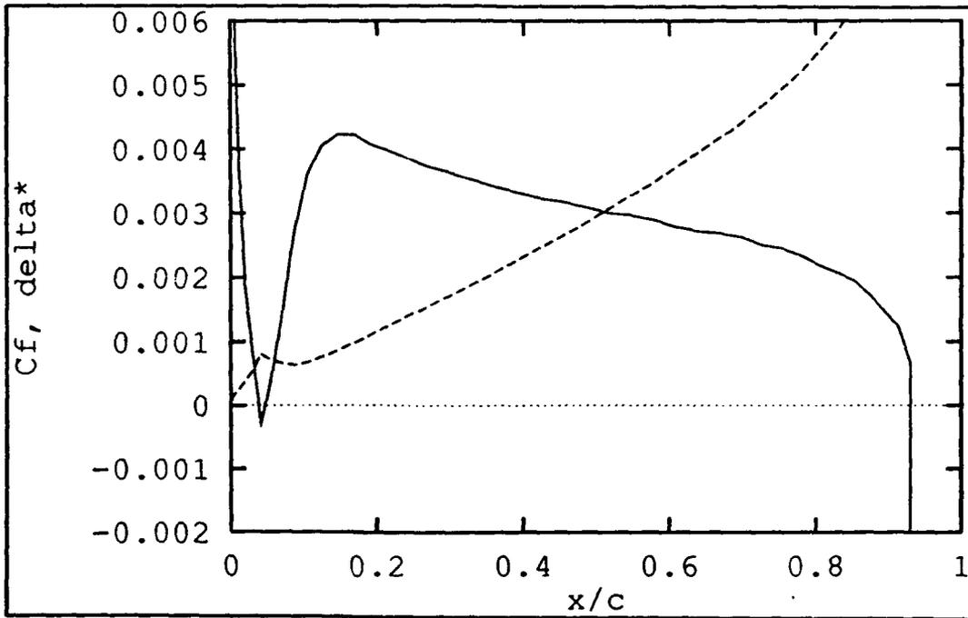
Figure 3.7 BL2D:  $C_f$  and  $\delta^*$ , NACA 0012, AOA=6°, Re=540,000
