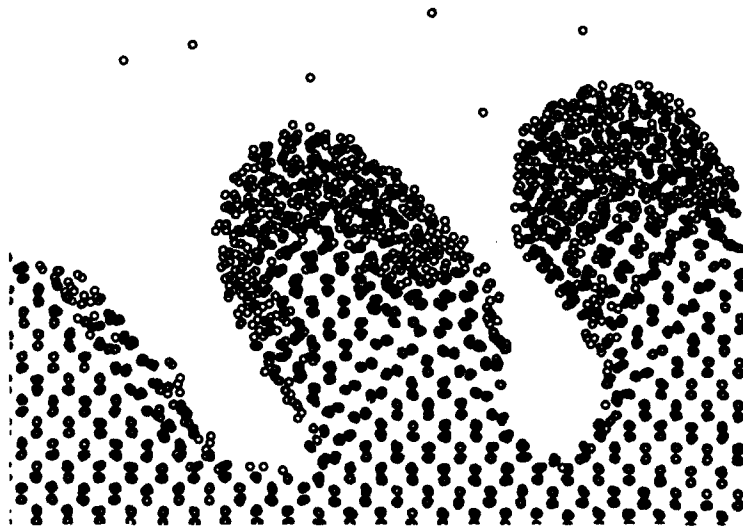
Figure 5. Molecular dynamics simulation result of Si columnar structure growth.
