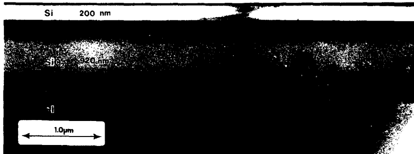
Figure 4. Silicon on insulator fabricated by bond and etch back using a SiGe alloy as etch stop.
