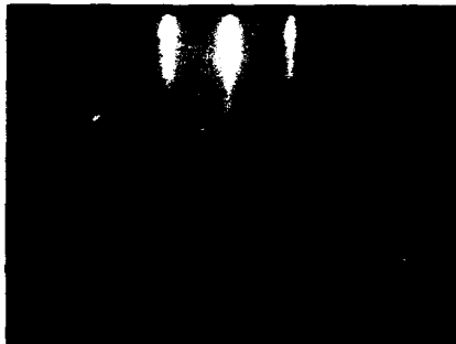
Fig. 1c: RHEED-pattern of a 200nm thick BaF 2 layer grown at 450°C.
