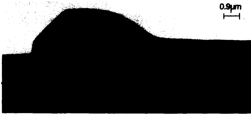
Fig. 4 A small DCS is applied in the prebake and ramp-down periods. In the absence of the HF vapor treatment, the epilayer is defective with interfacial oxide islands and threading dislocations.
